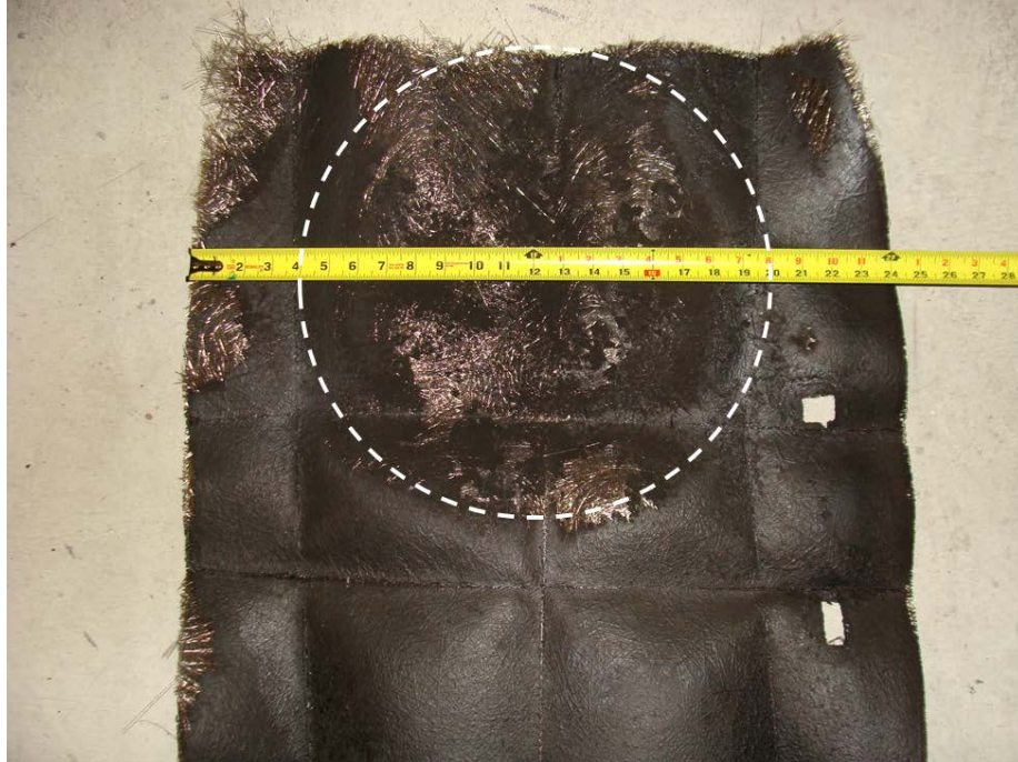
Figure 44. The damage area is shown for the DOT headliner: diameter of damaged area = 16" = 40.6 cm, radius = 20.3 cm
