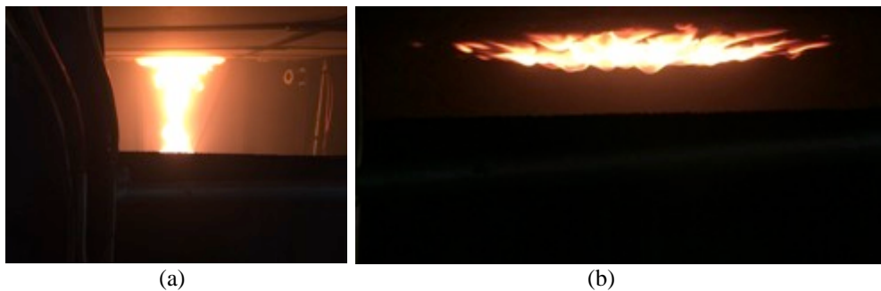
Figure 9. Ceiling flames: (a) fire below and (b) ceiling alone
