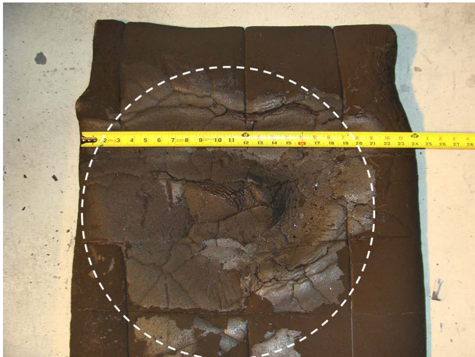
Figure 43. The damage area is shown for the gray foam: diameter of damaged area = 21" = 53.3 cm, radius = 26.7 cm
