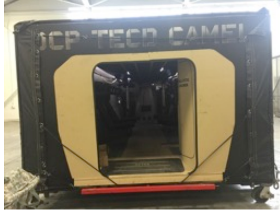
Figure 8. TARDEC “wood buck” model for fire testing
