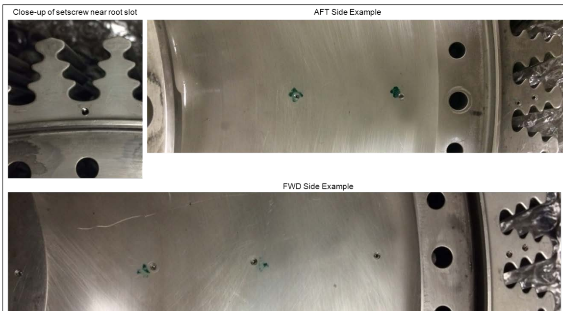
Figure 16. Close-up views of 2-56 tapped holes installed in JT8D second-stage turbine disk
