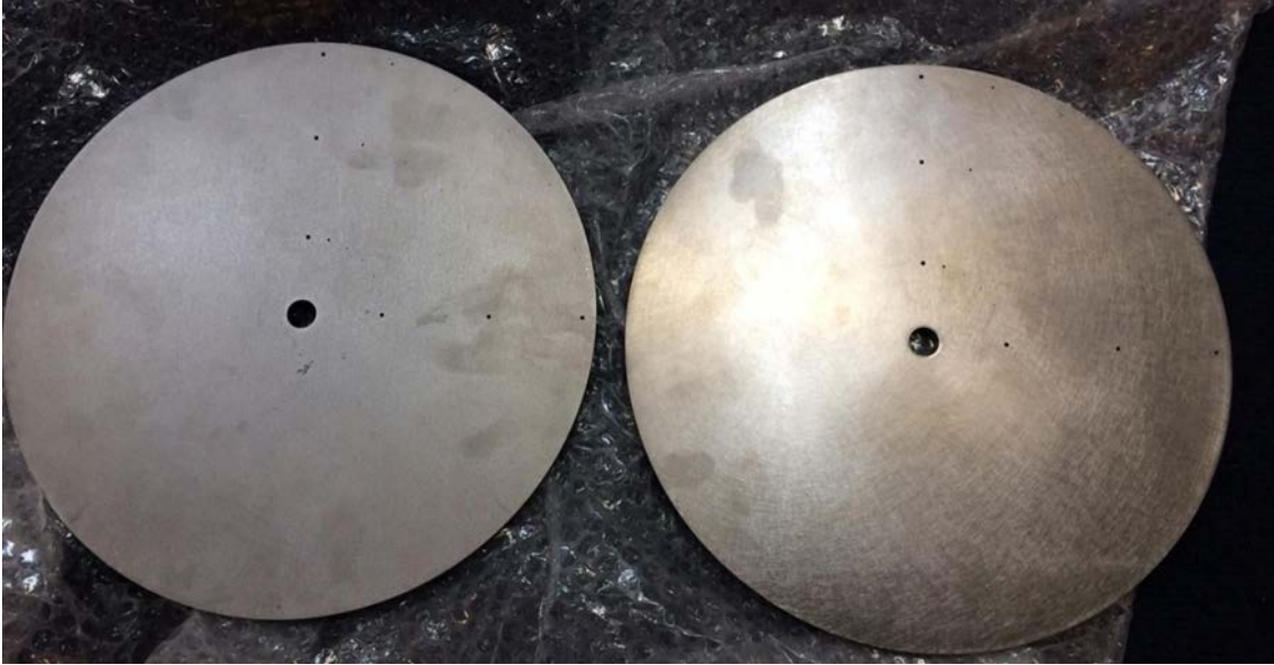
Figure 3. Defect specimen disks—Ti6-4 (left) and IN718 (right)
