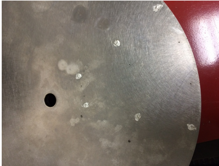
Figure 9. Epoxy installation on test disk, pre-sanding
