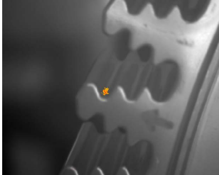
Figure B-5. JT8D turbine disk with DRA results revealing HCF crack
