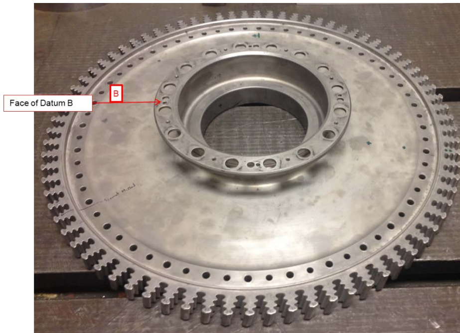
Figure A-2. AFT view of JT8D disk
