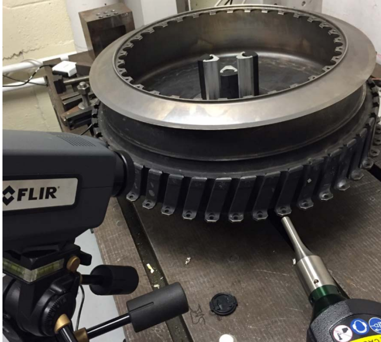
Figure C-1. Example SIR inspection configuration for disk
