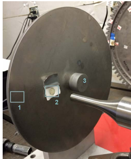
Figure 5. Excitation locations of AD disk for SIR
