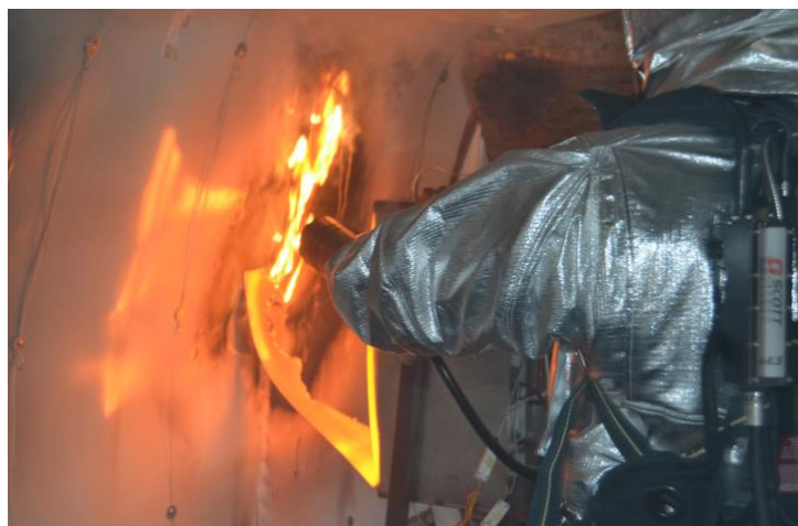
Figure 45. Fire Caused by Failed Aluminum Panel: Test 7
