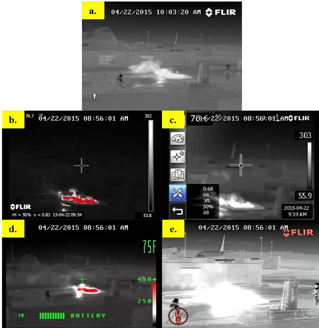
Figure 69. The 6-ft-Square Pan Fire Being Extinguished Captured by (a) Patrol IR, (b) P660, (c) T420, (d) XR, and (e) M625L
