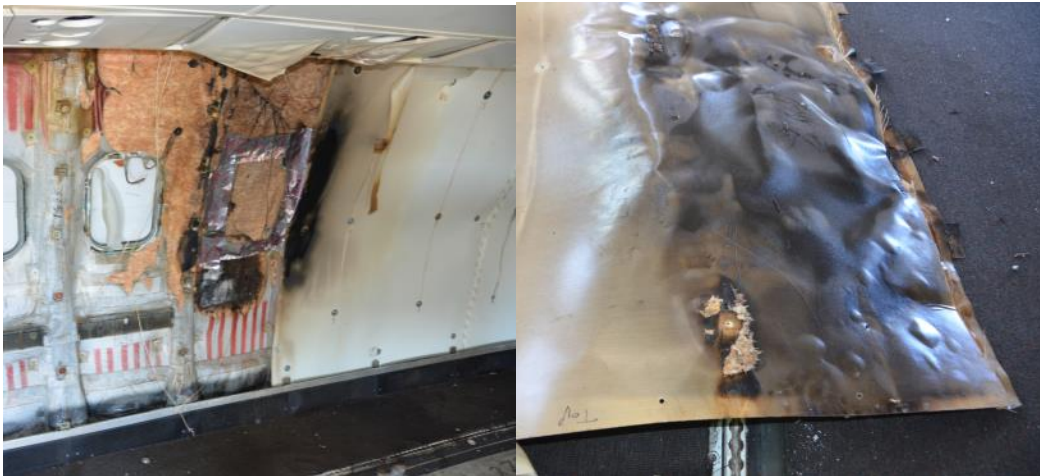
Figure 43. Damage to Interior: Test 5
