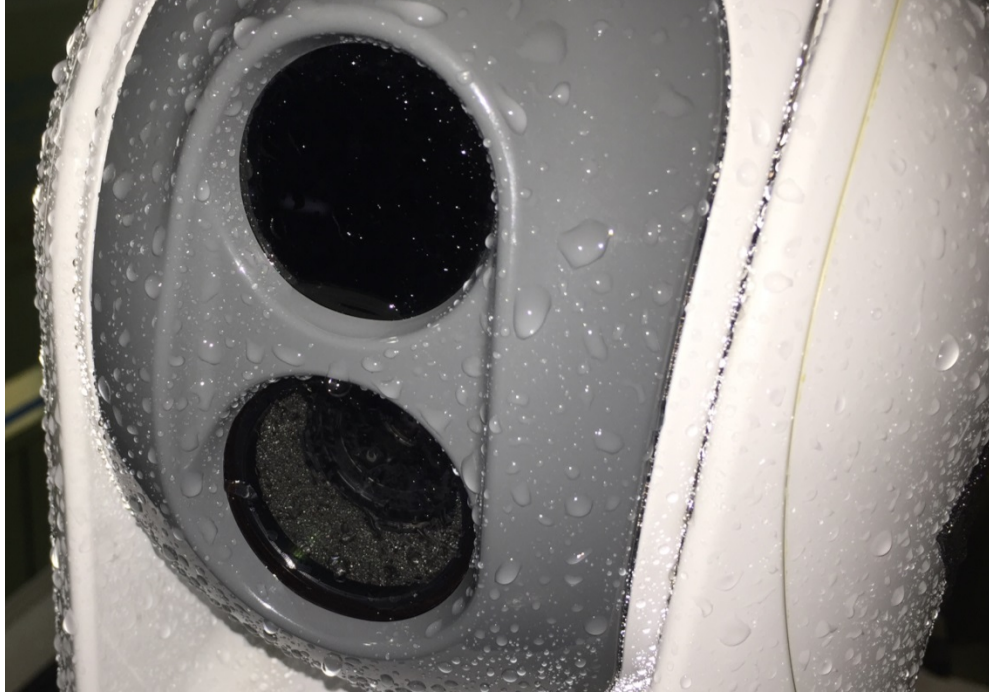
Figure 66. Rain Accumulation for Heavy Rain
