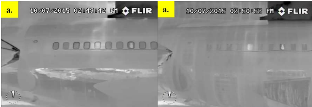
Figure 26. Before and After Wet-Down Strategy: Test 2 Using Patrol IR
