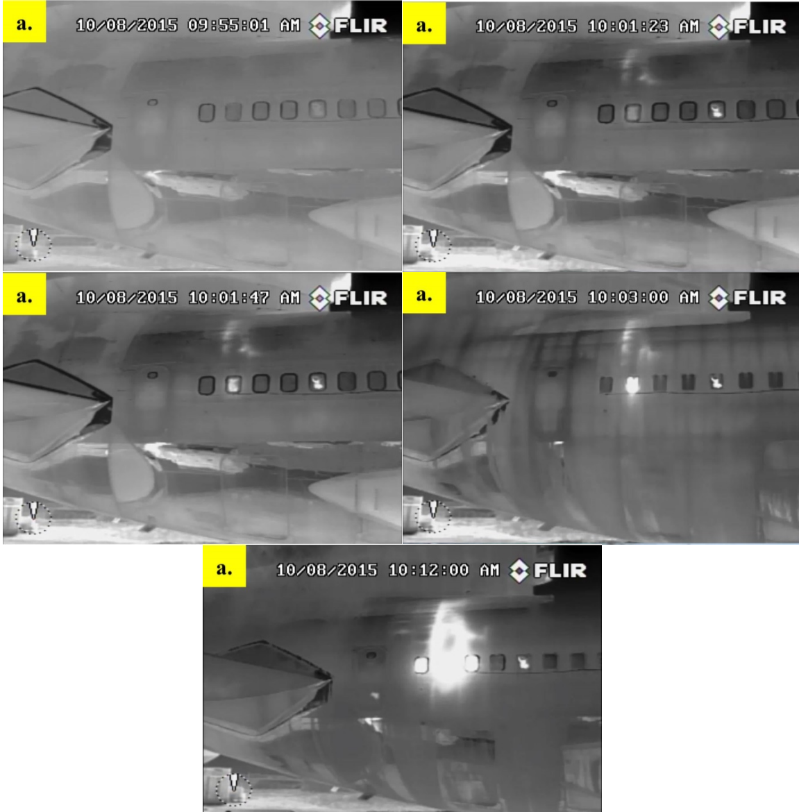
Figure A-11. Test 3 IR Camera Screen Captures: Patrol IR
