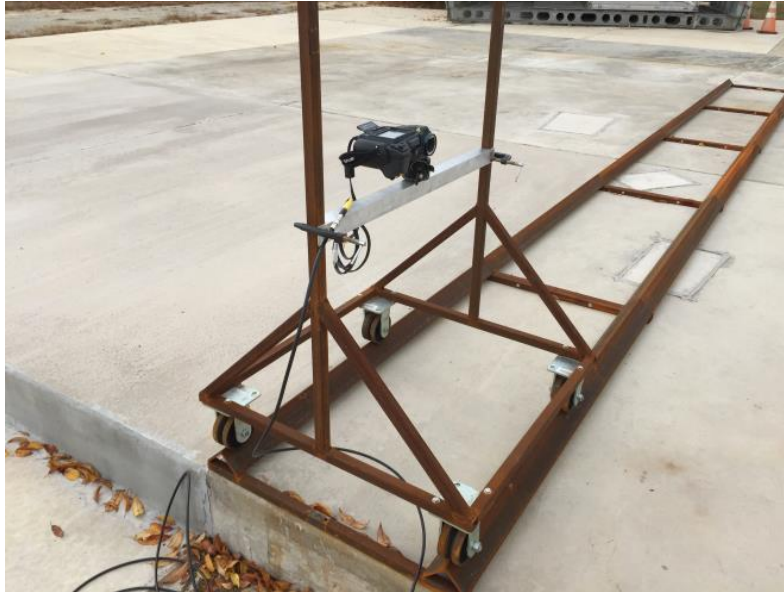
Figure 16. Camera Track System
