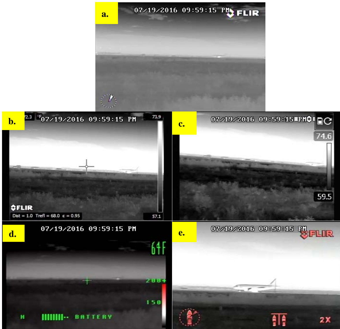
Figure 79. The 2500-ft DEVS Nighttime Test Using (a) Patrol IR, (b) P660, (c) T420, (d) XR, and (e) M625L
