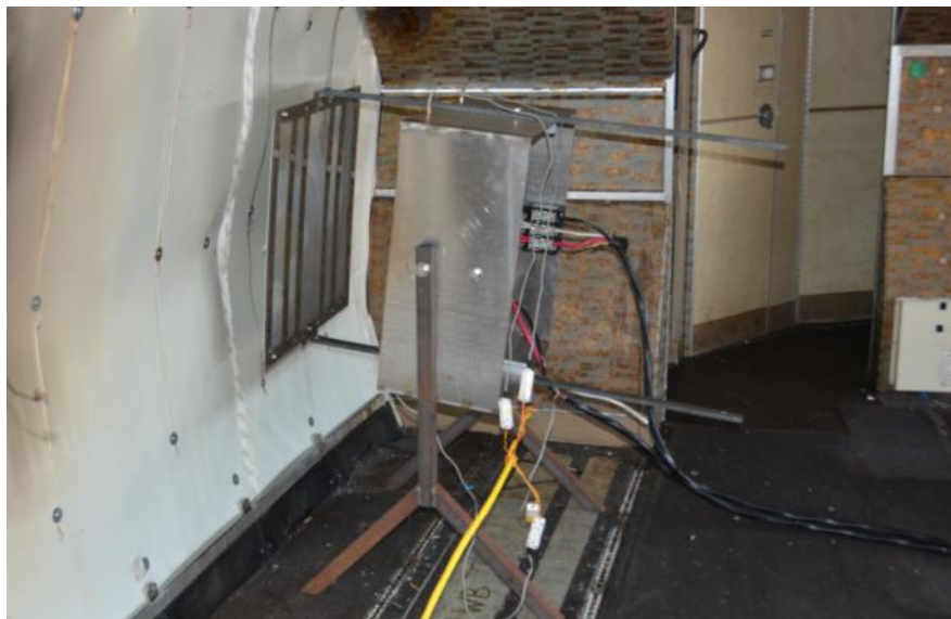
Figure 13. Quartz Heater Assembly With Simulated ULD Panel
