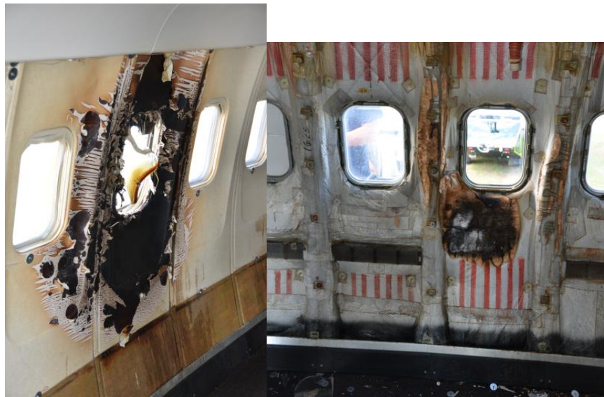
Figure 36. Damage to Aircraft Interior: Test 2
