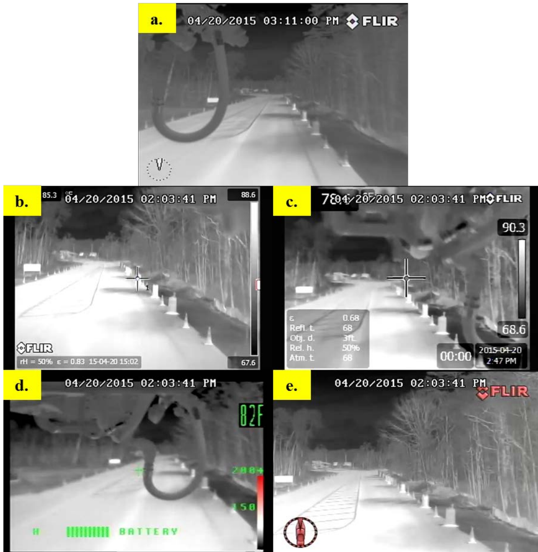
Figure 58. Asphalt Road Comparison II Using (a) Patrol IR, (b) P660, (c) T420, (d) XR, and (e) M625L
