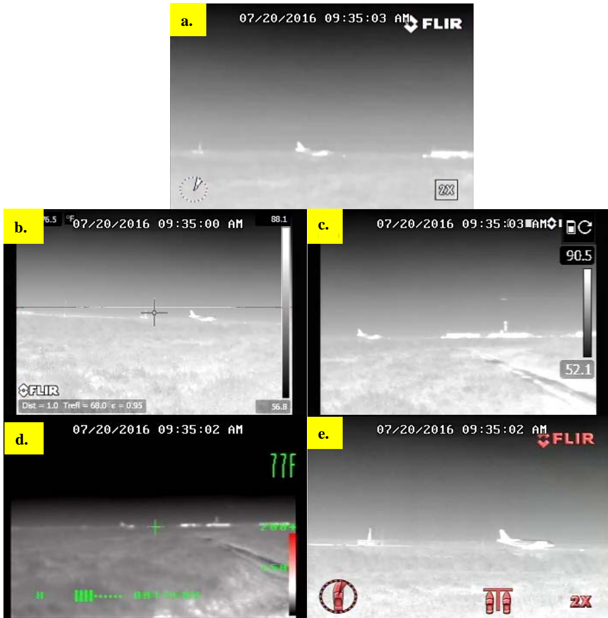
Figure 77. The 3000-ft DEVS Daytime Test 2 Using (a) Patrol IR, (b) P660, (c) T420, (d) XR, and (e) M625L
