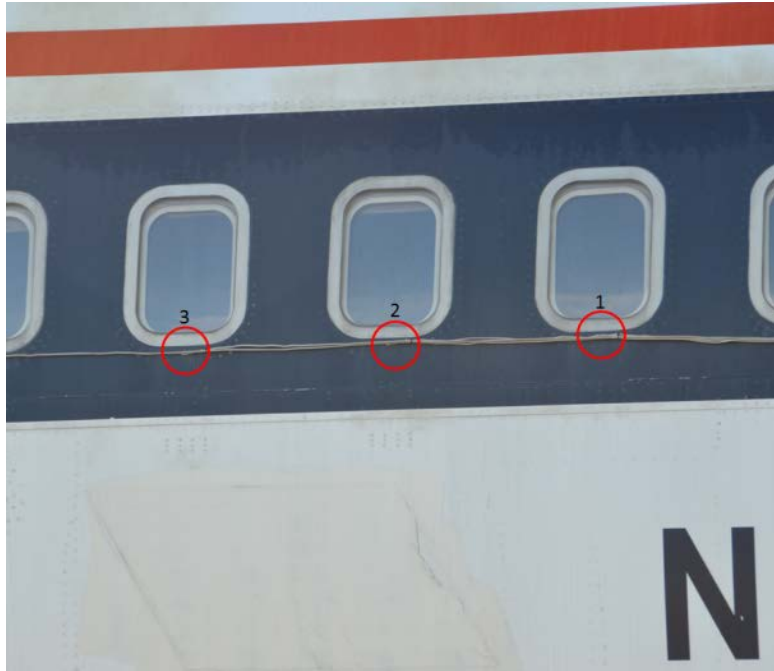
Figure 11. The L-1011 Exterior Thermocouple Locations
