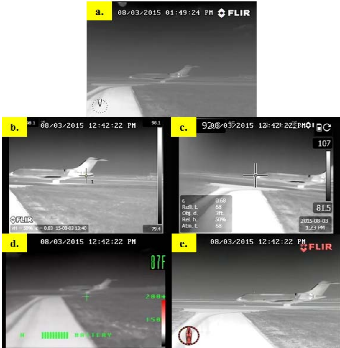
Figure 80. Hot Brakes Test Using (a) Patrol IR, (b) P660, (c) T420, (d) XR, and (e) M625L
