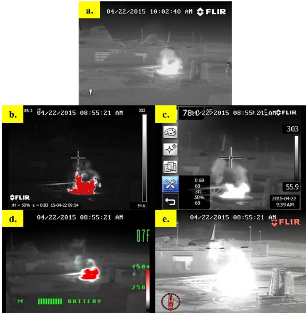
Figure 68. The 6-ft-Square Pan Fire Captured by (a) Patrol IR, (b) P660, (c) T420, (d) XR, and (e) M625L
