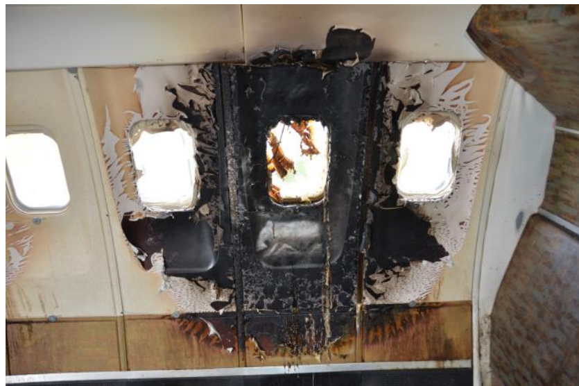
Figure 37. Damage to Aircraft Interior: Test 3
