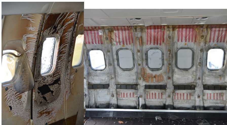
Figure 35. Damage to Aircraft Interior: Test 1
