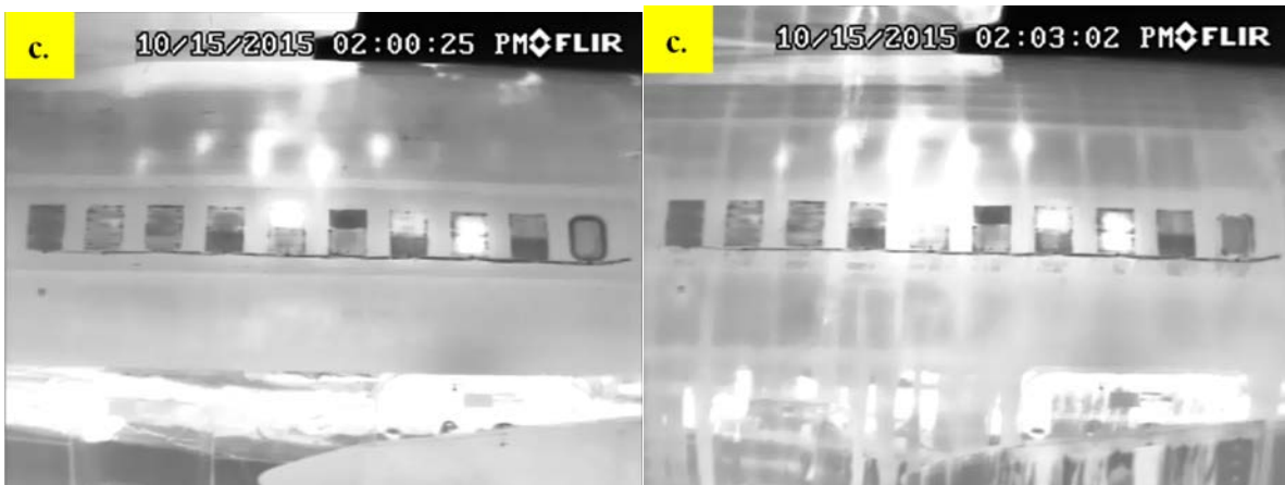
Figure 31. Before and After Wet-Down Strategy: Test 5 Using T420
