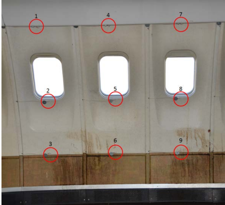
Figure 9. The L-1011 Interior Thermocouple Locations Passenger Configuration
