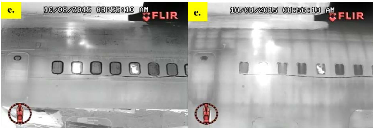
Figure 30. Before and After Wet-Down Strategy: Test 3 Using M625L
