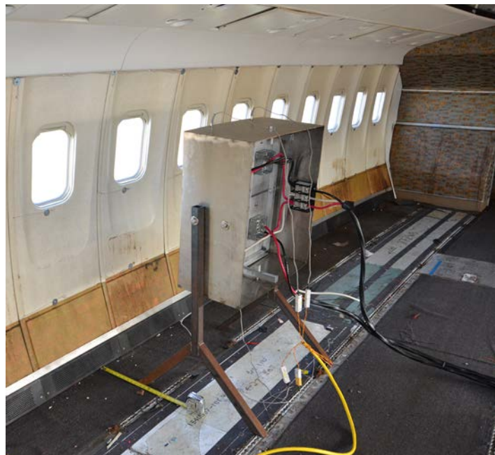
Figure 1. Quartz Heater Assembly Placement
