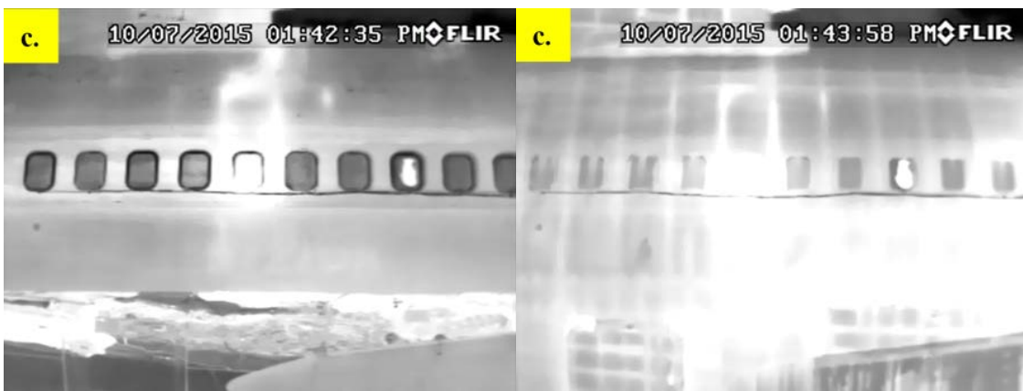
Figure 28. Before and After Wet-Down Strategy: Test 2 Using T420
