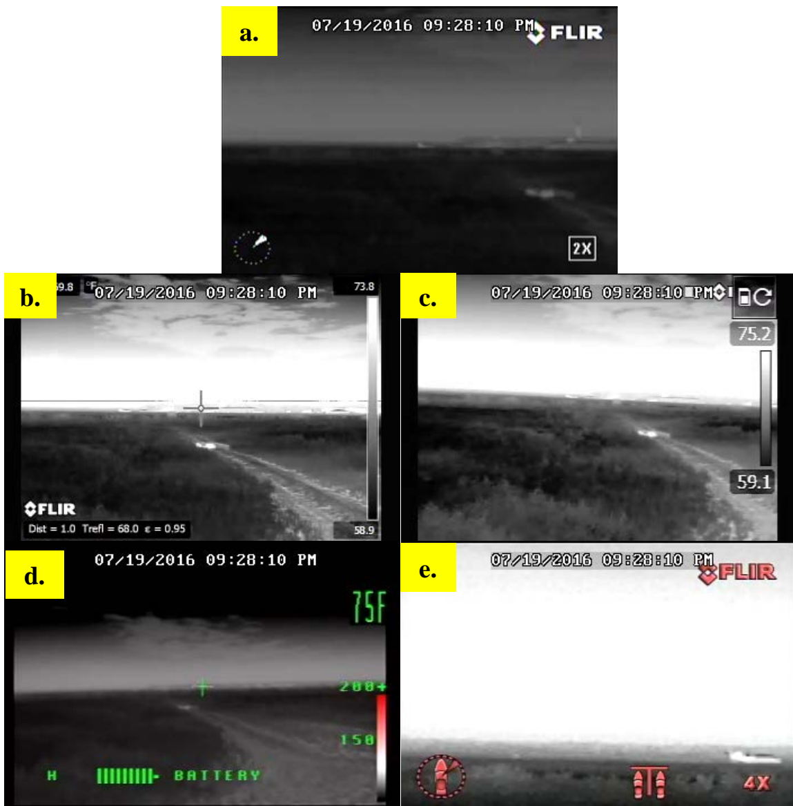
Figure 78. The 3000-ft DEVS Nighttime Test Using (a) Patrol IR, (b) P660, (c) T420, (d) XR, and (e) M625L
