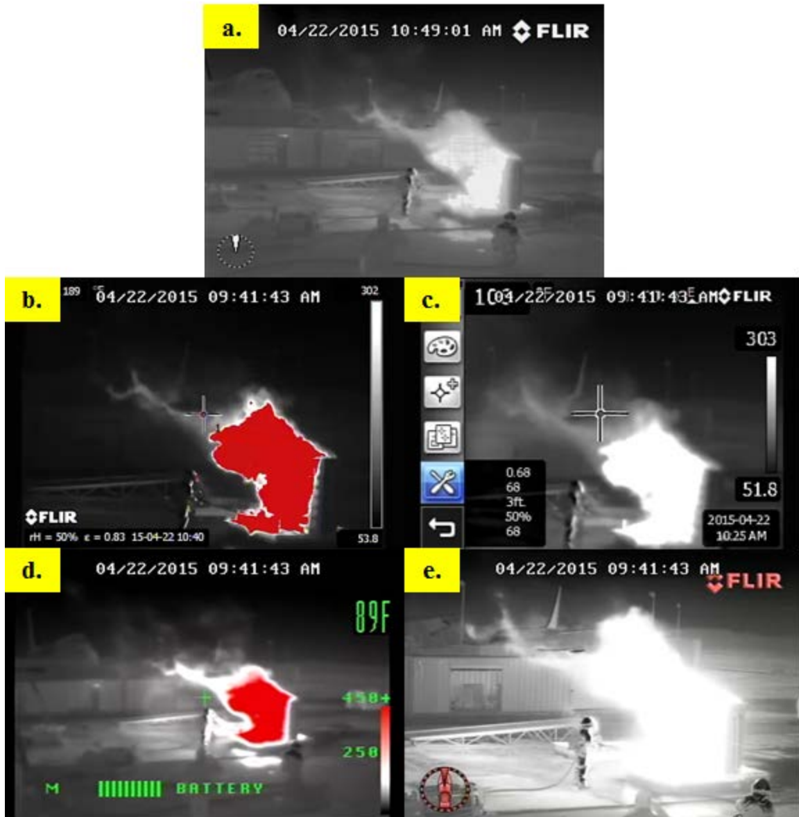
Figure 71. The 3-D Fire Being Extinguished Captured by (a) Patrol IR, (b) P660, (c) T420, (d) XR, and (e) M625L
