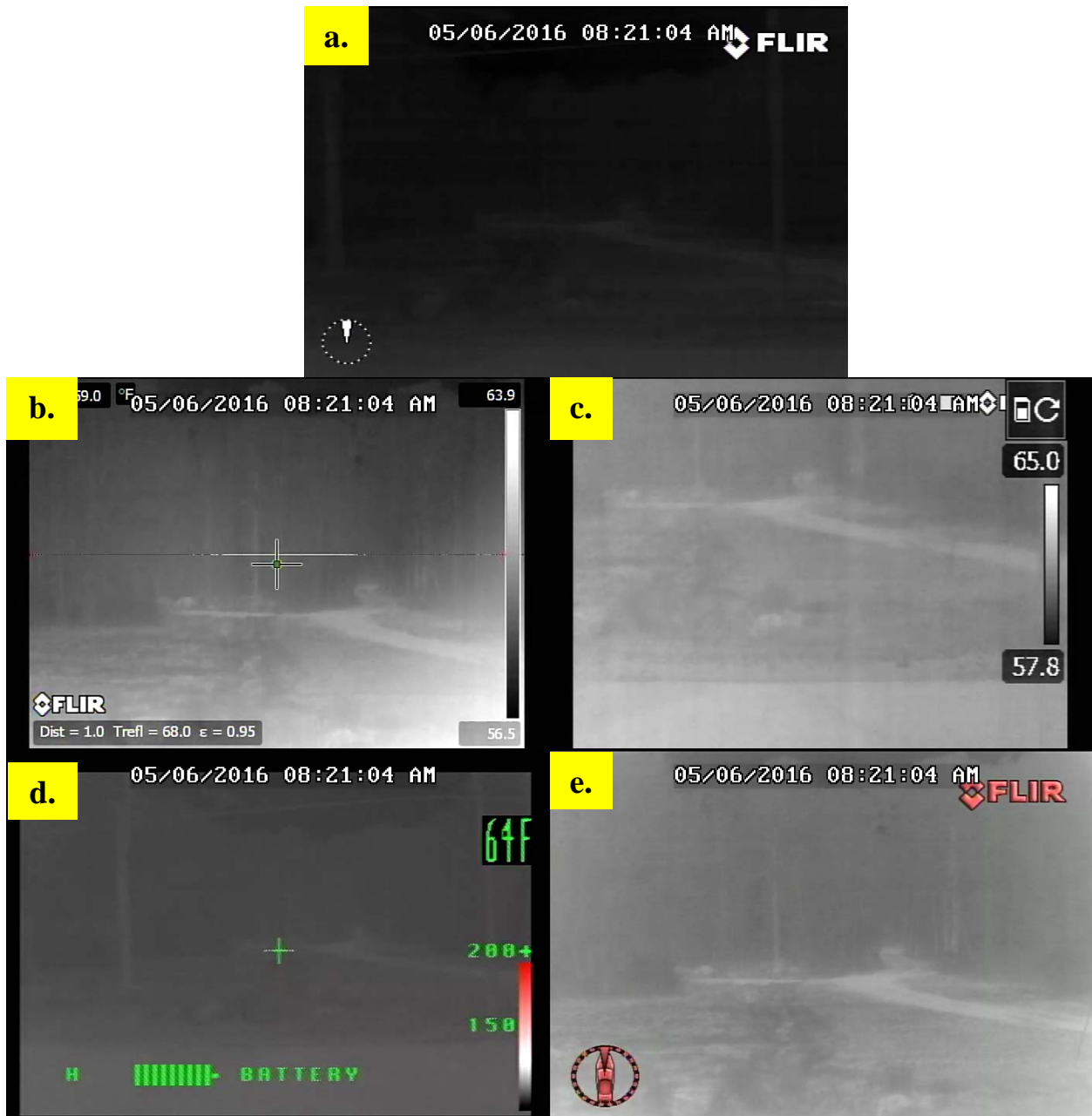
Figure 63. Moderate Rain, Woods/Dirt Road View Using (a) Patrol IR, (b) P660,(c) T420, (d) XR, and (e) M625L
