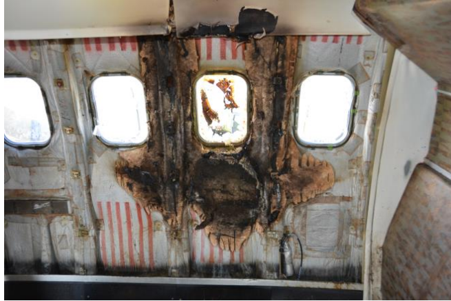
Figure 38. Damage to Aircraft Insulation: Test 3
