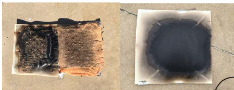
Figure 54. Sample of Insulation and Interior Cargo Liner Panel Damage
