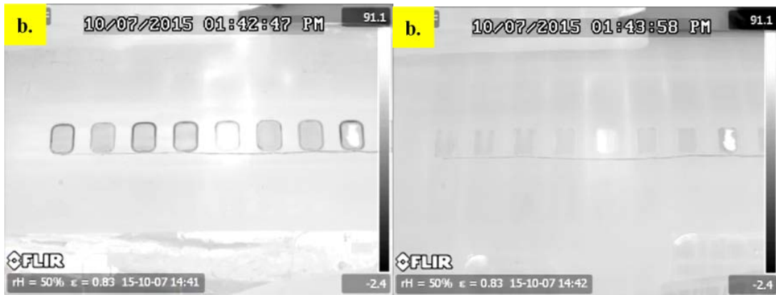
Figure 27. Before and After Wet-Down Strategy: Test 2 Using P660
