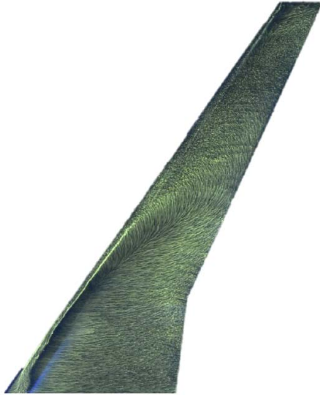
Figure 12. Oil flow of the stalled clean wing ( A = 9.6^\circ )
