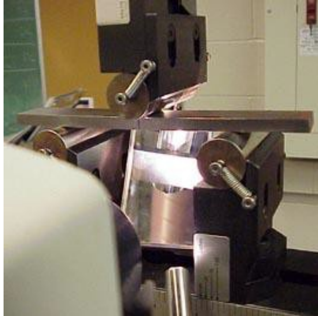
Figure 32. Sample loaded in three-point bending
