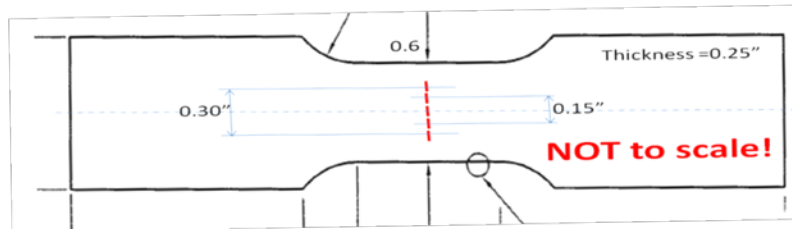
Figure G-7. Location of FIB notches in SC(T) specimens used in the previous program
