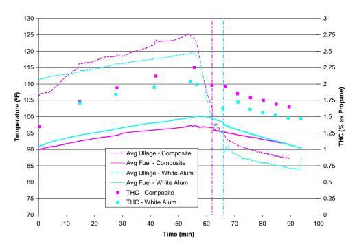
Figure 7. Comparison of white-painted aluminum and bare composite material fuel tank results for a 60% fuel load under the low-heat setting
