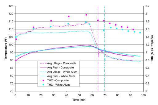
Figure 6. Comparison of white-painted aluminum and bare composite material fuel tank results for a 40% fuel load under the low-heat setting
