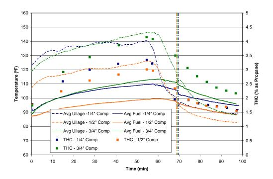
Figure 19. Comparison of various thickness composite material fuel tank results for a 40% fuel load under the high-heat setting
