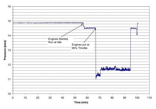
Figure 1. Typical pressure profile of fuel tank during wind tunnel operations
