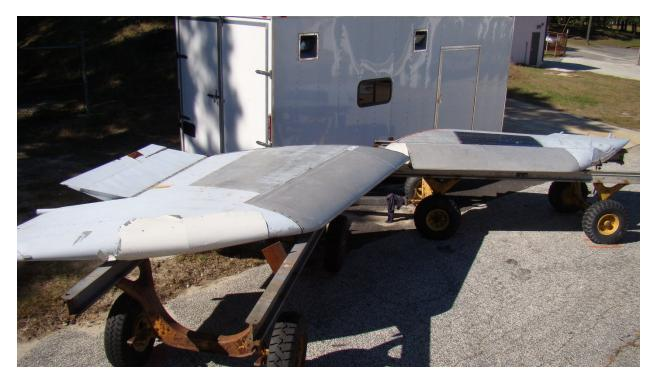
Figure 2. 727 wing tank test articles
