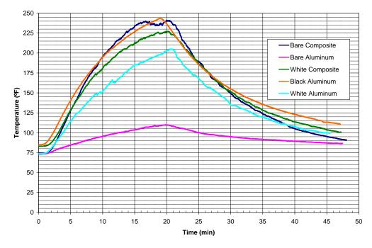
Figure 4. Comparison of center-point temperature for the bare and painted composite and aluminum materials during panel-heating test
