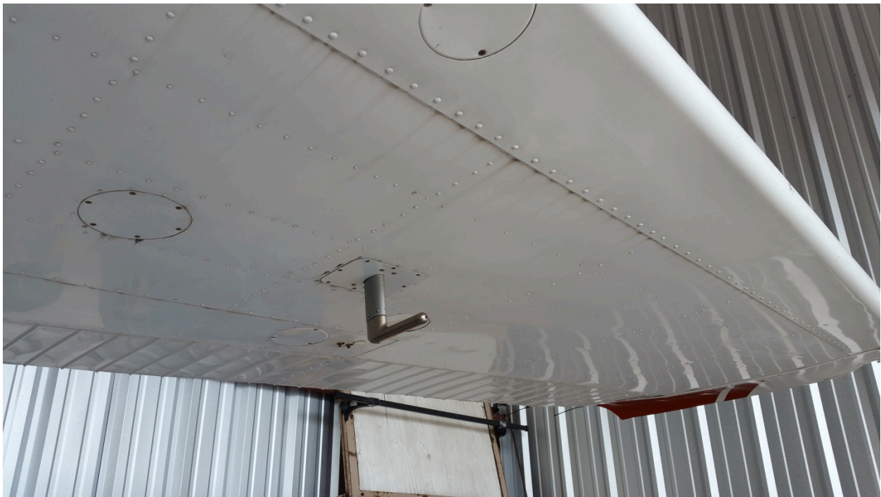
Figure 2. Initial location of Garmin multi-hole GAP 26 probe sensor in test aircraft
