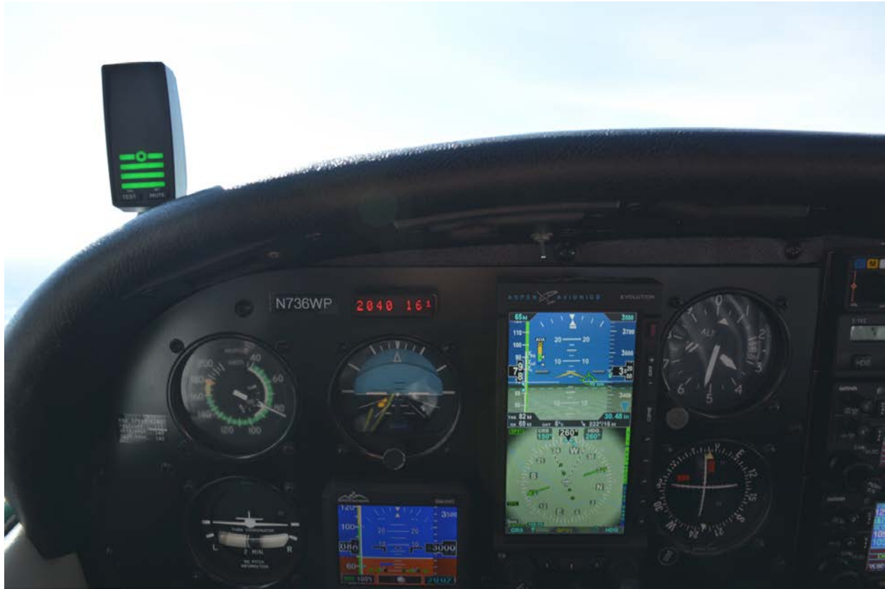
Figure 1. Garmin GI 260 indicator on left side of glareshield in test aircraft
