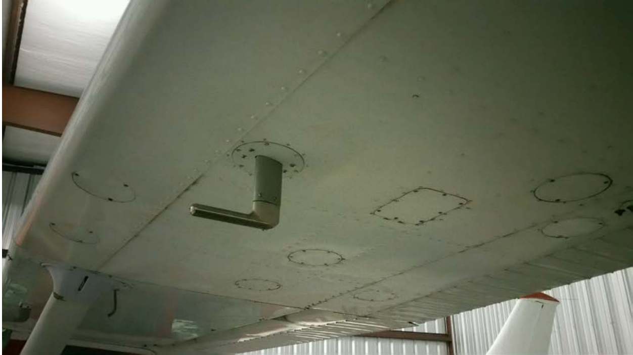
Figure 3. Relocated Garmin GAP 26 probe on test aircraft
