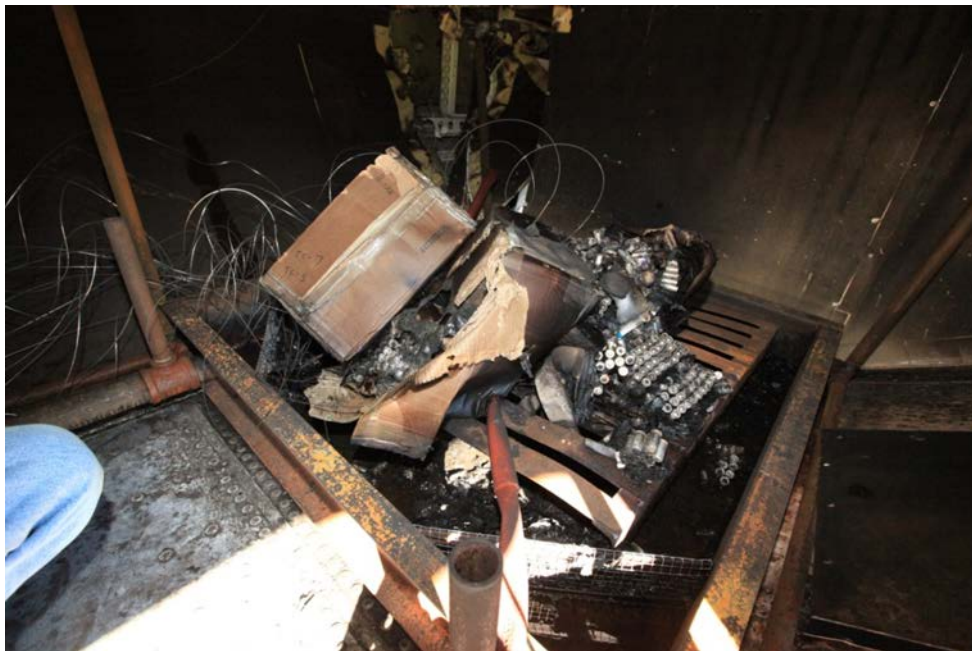
Figure 19. Lithium-metal cells post test
