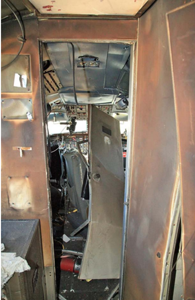
Figure 21. Flight deck bulkhead damage and door
