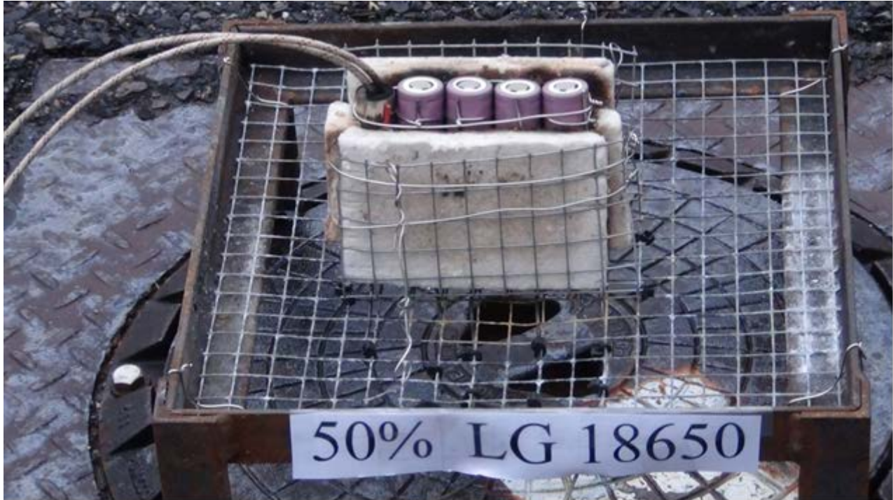
Figure 9. Propagation test configuration
