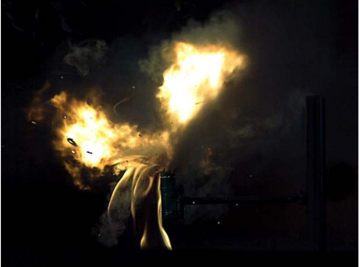
Figure 1. High-speed video capture of lithium-ion LiCoO 2 cell in thermal runaway
