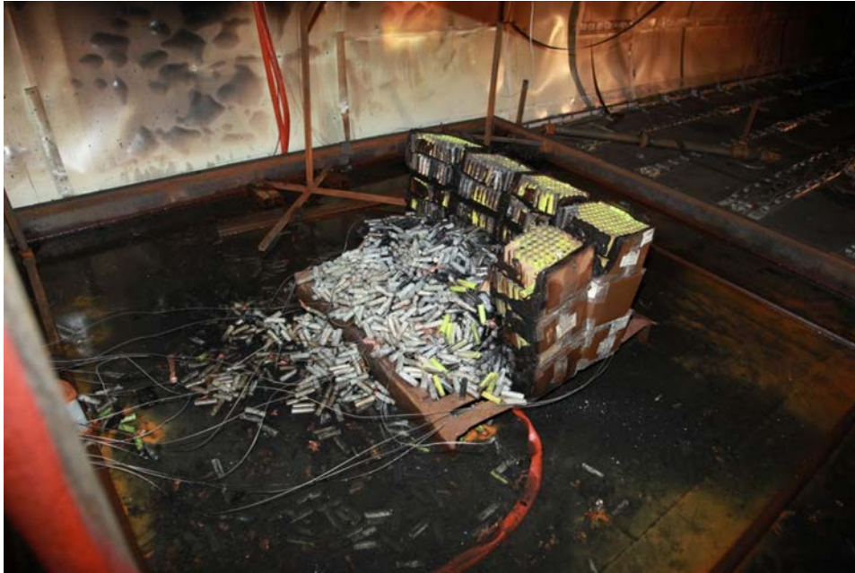
Figure 15. Lithium-ion cells consumed post test
