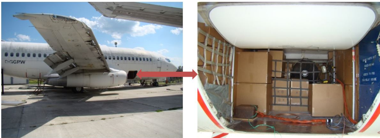
Figure 37. Pressure chamber used to simulate 70% loaded cargo compartment
