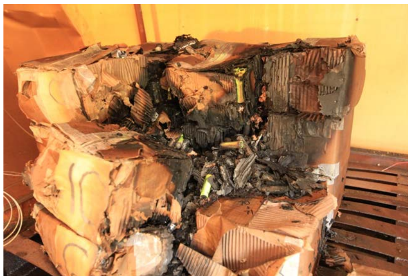
Figure 18. Image of the 1200 lithium-ion cells that were consumed
