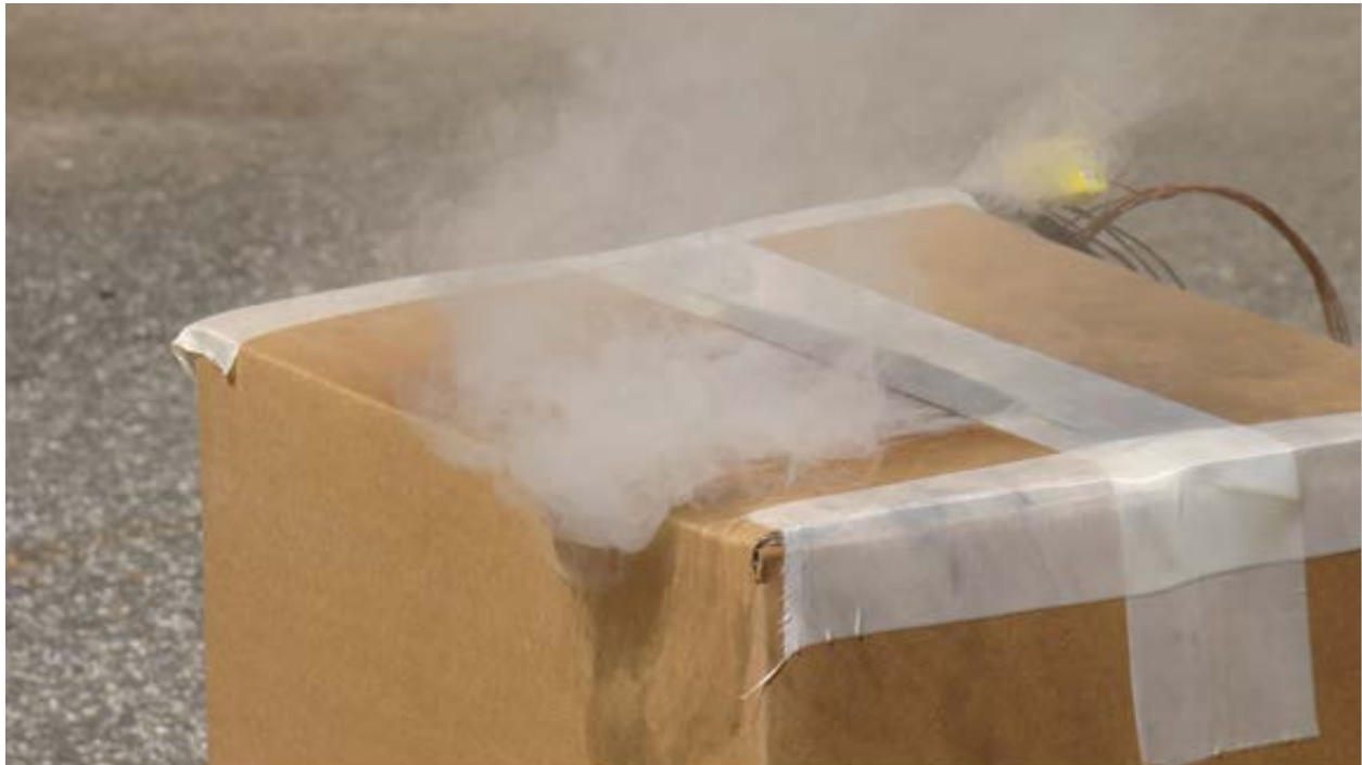
Figure 6. Oxygen-generator overpack test
