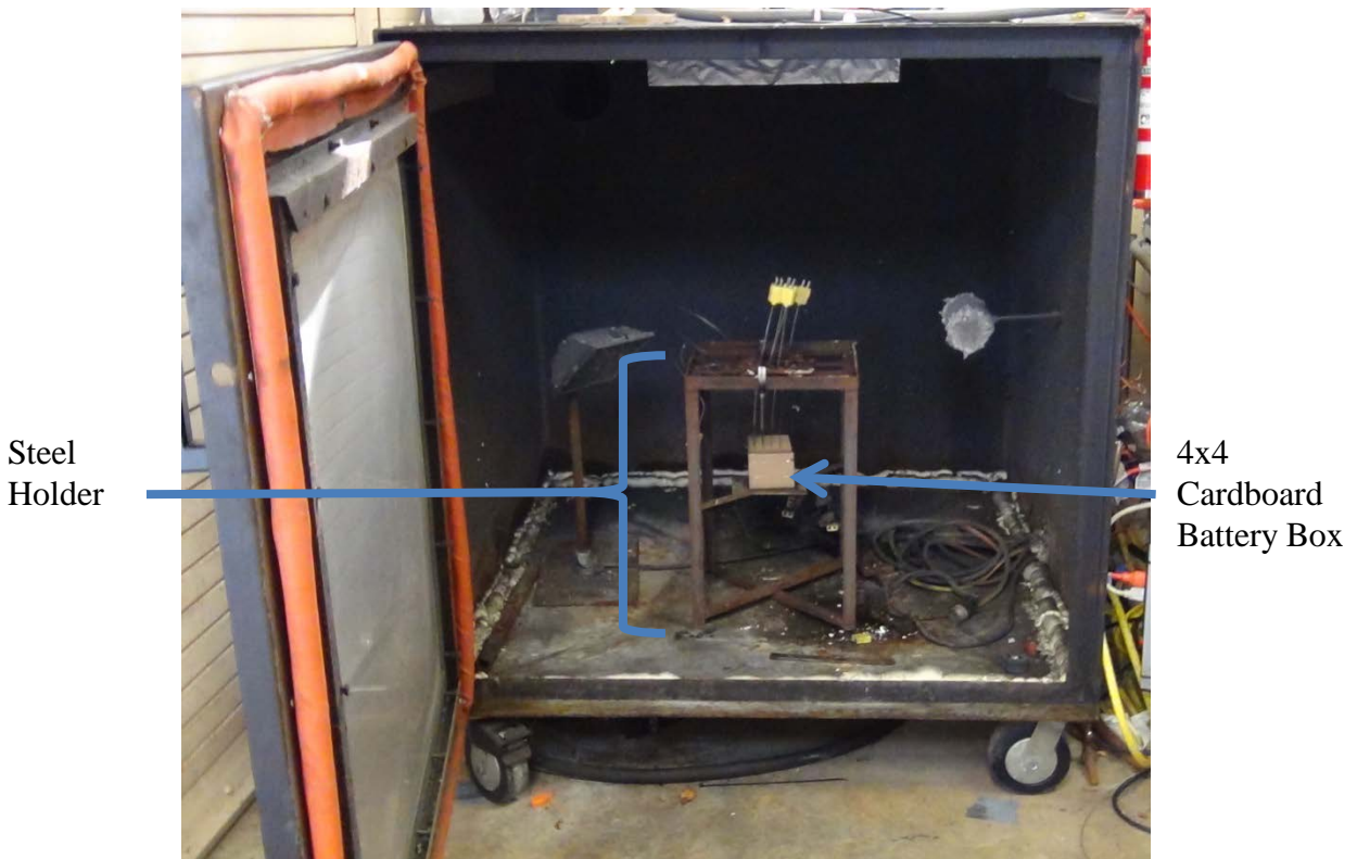
Figure 47. Test chamber and setup
