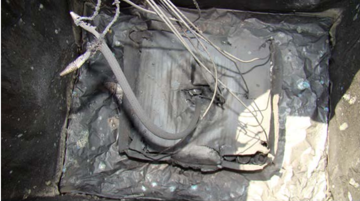
Figure 7. Oxygen-generator overpack post test
