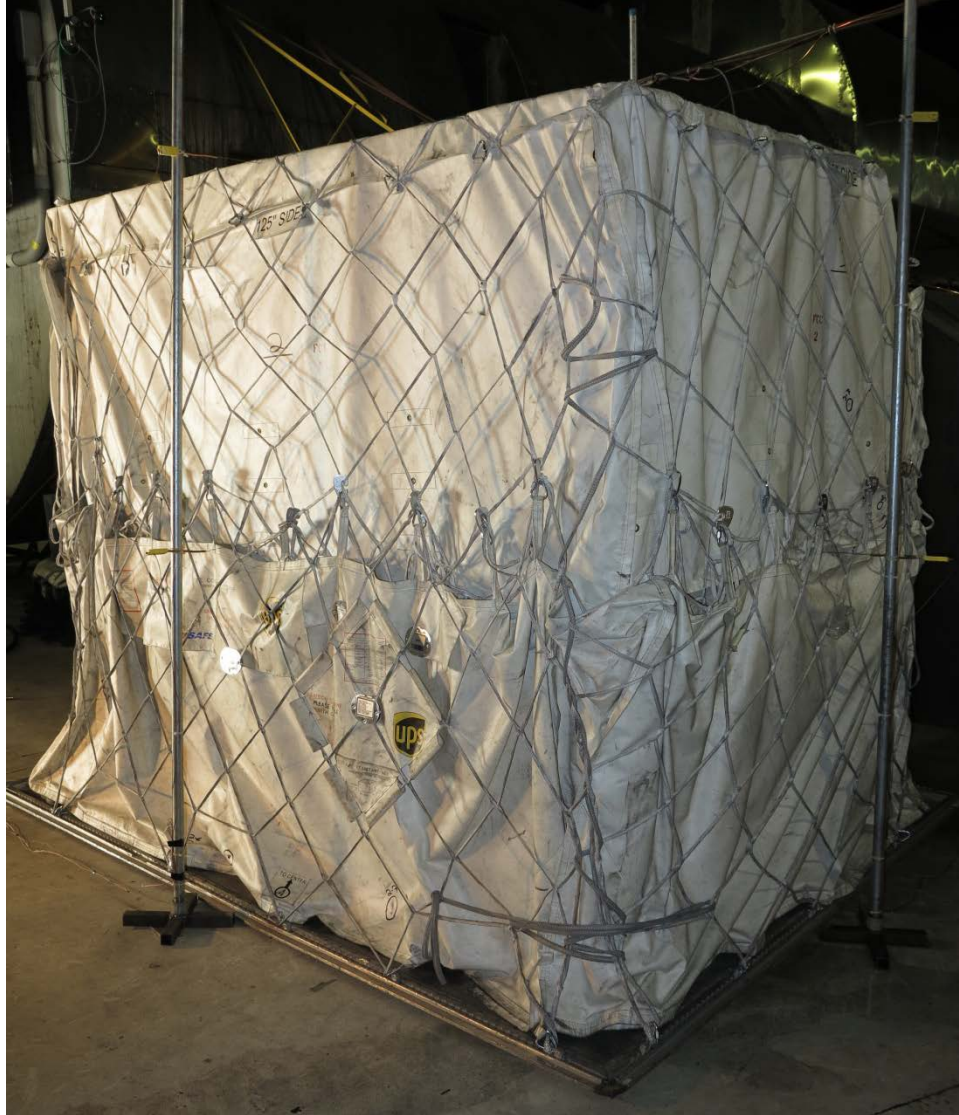
Figure 24. Full-scale fire-test setup of an FCC
