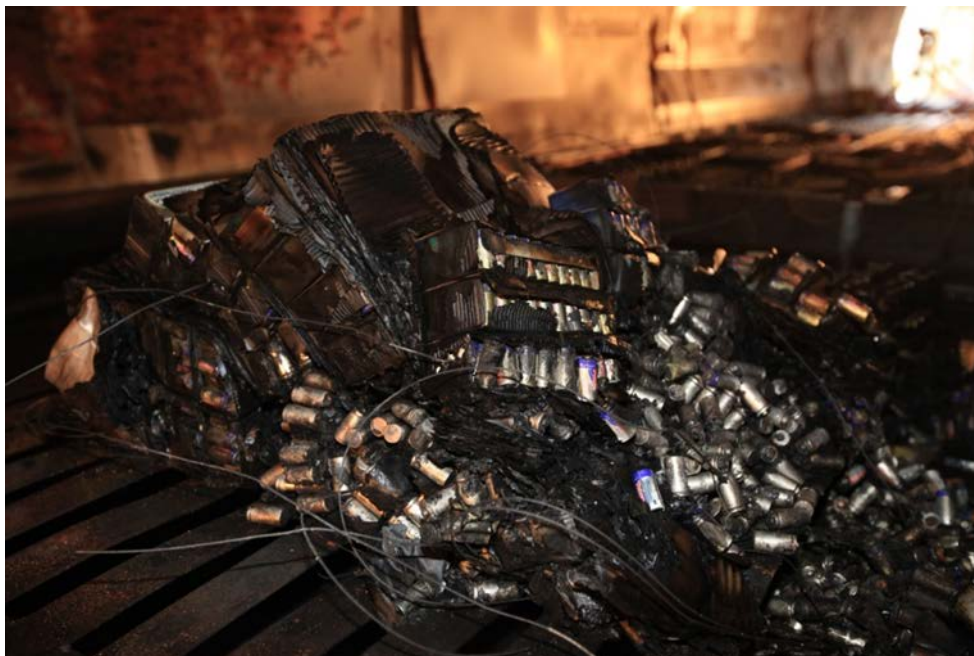
Figure 16. Lithium-metal cells post test
