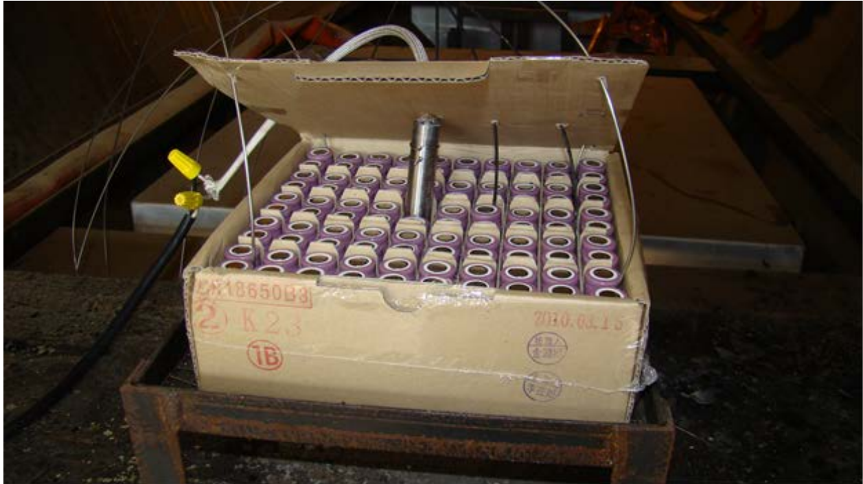
Figure 3. Shipping box with interlocking cardboard separators for 100 18650 LiCoO 2 lithium-ion cells
