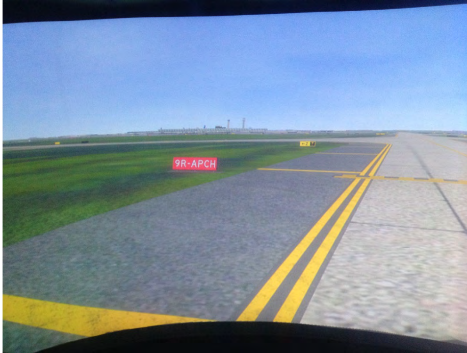
Figure B-3. Standard Sign With Only Approach RWY: TWY T, North of TWY Z Intersection, Day
