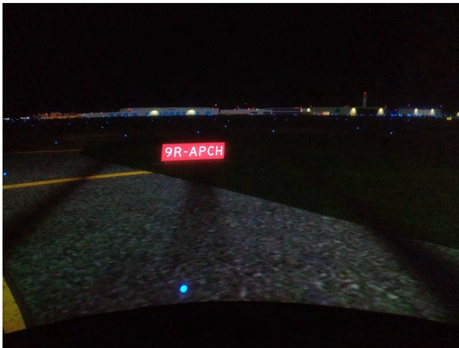
Figure B-6. Standard Sign With Only Approach RWY: TWY T, South of TWY W Intersection, Night
