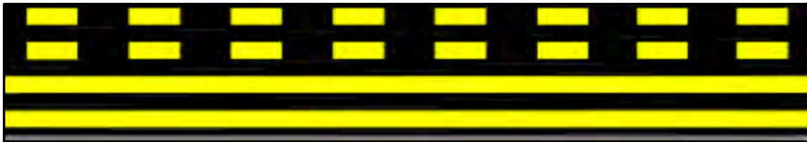
Figure 2. Pattern A Runway Holding Position Marking [2]
