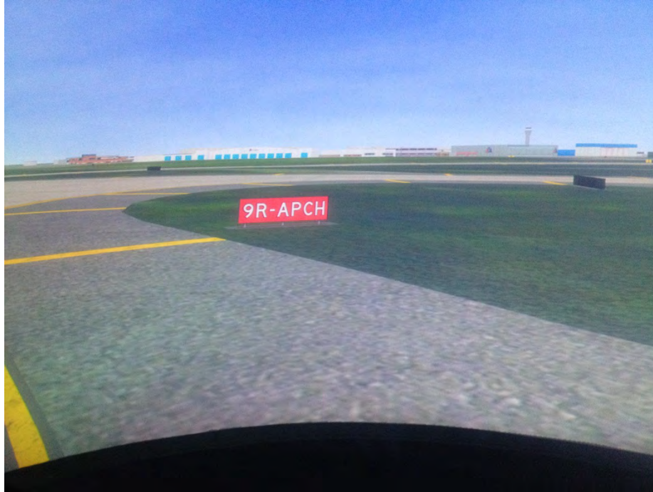
Figure B-5. Standard Sign With Only Approach RWY: TWY T, South of TWY W Intersection, Day
