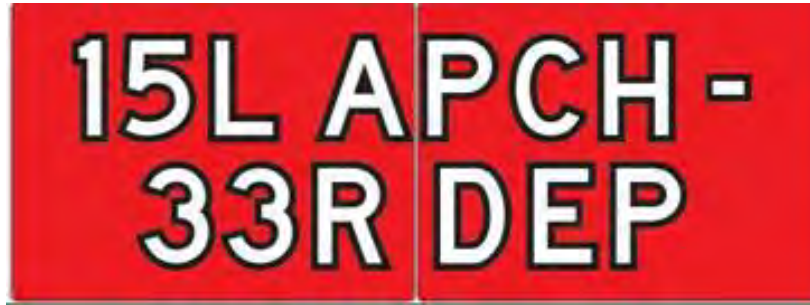
Figure C-3. Stacked Runway Safety Area/Approach Hold Signage
