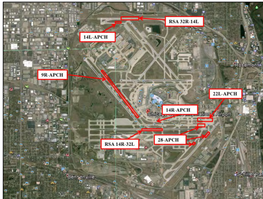
Figure 22. View of Approach Hold and RSA Signs and Marking Areas at ORD
