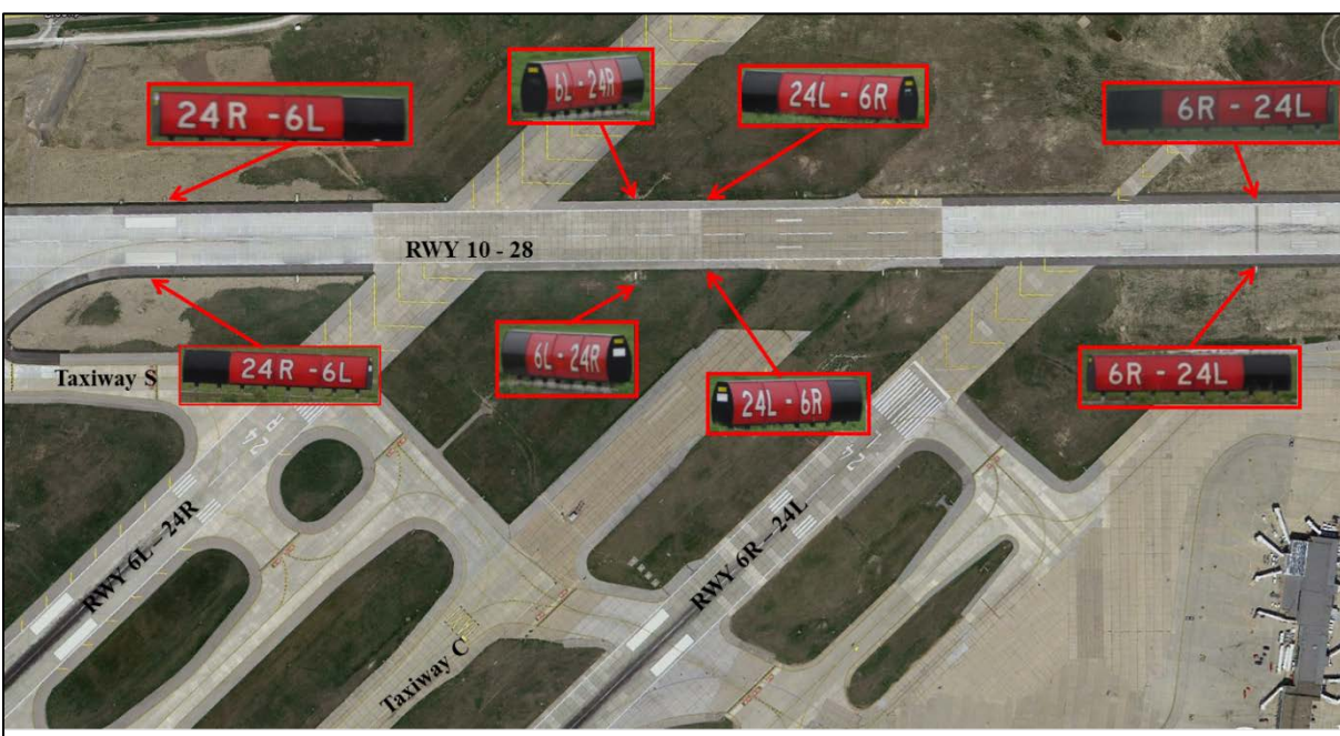
Figure 31. The RSA Locations Where RWYs 6L-24R and 6R-24L Intersect With RWY 10-28 at CLE
