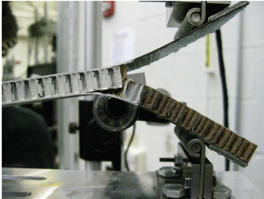
(b) Kinking and core rupture
