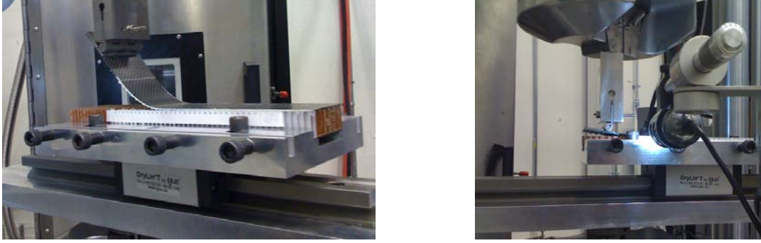
Figure 8. Sliding SCB test fixture design
