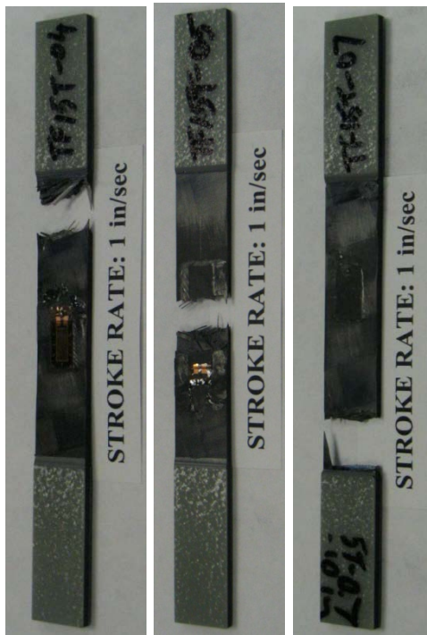
Figure D-11. Failure modes for carbon fabric [15^\circ/-15^\circ]_{2S} at a speed of 1 in/s, in tension
