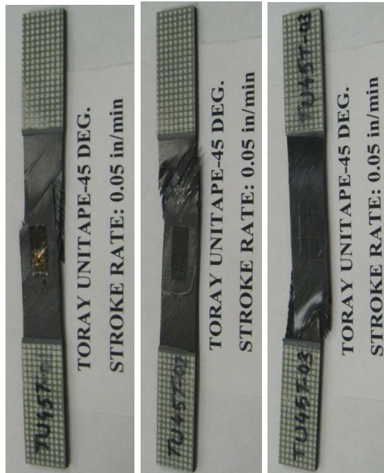
Figure C-25. Failure modes for carbon Unitape [45°/-45°] 2S at a speed of 0.0008 in/s, in tension
