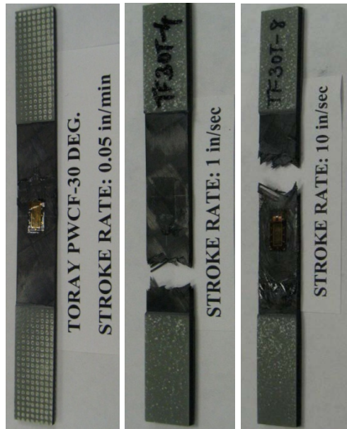
Figure D-23. Failure modes for carbon fabric [30^\circ/-30^\circ]_{2S} : summary of all speeds, in tension
