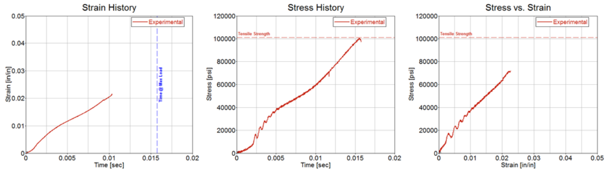
Figure 42. Stress-strain curve limited by strain gage capability in fiberglass [0^\circ]_4 at a speed of 10 in/s
