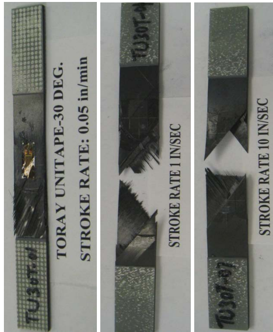
Figure C-23. Failure modes for carbon Unitape [30^\circ/-30^\circ]_{2S} : summary of all speeds, in tension
