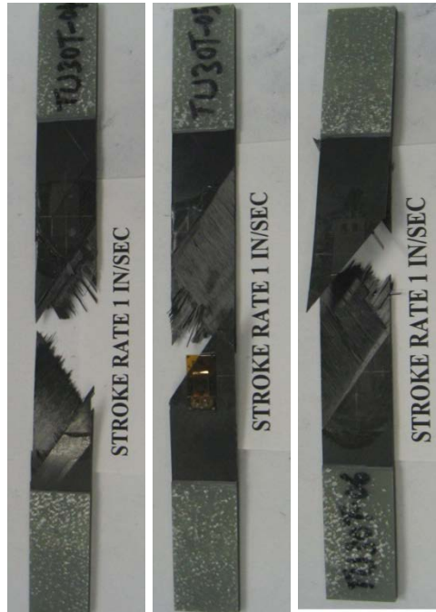
Figure C-19. Failure modes for carbon Unitape [30°/-30°] 2S at a speed of 1 in/s, in tension
