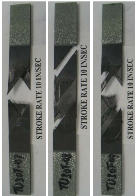
Figure C-21. Failure modes for carbon Unitape [30°/-30°] 2S at a speed of 10 in/s, in tension
