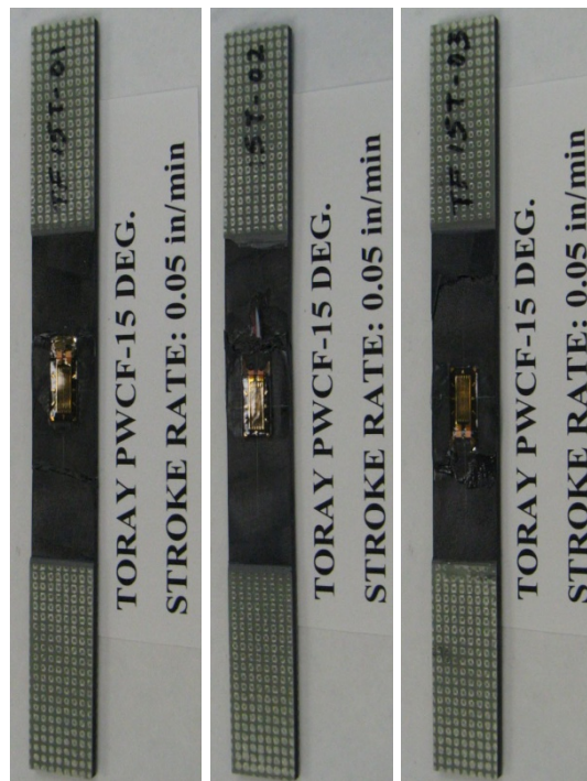
Figure D-9. Failure modes for carbon fabric [15°/-15°] 2S at a speed of 0.0008 in/s, in tension
