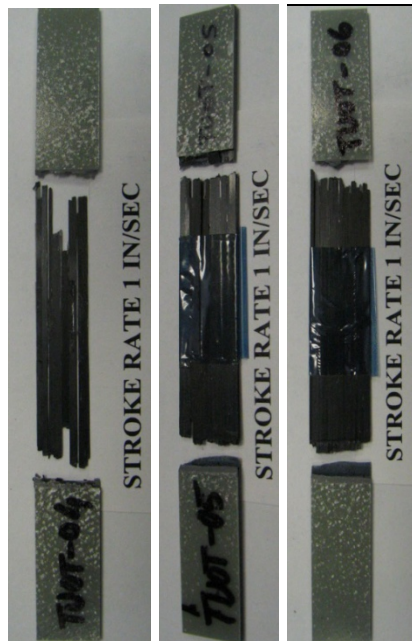
Figure C-3. Failure modes for carbon Unitape [0°] 2 at a speed of 1 in/s, in tension
