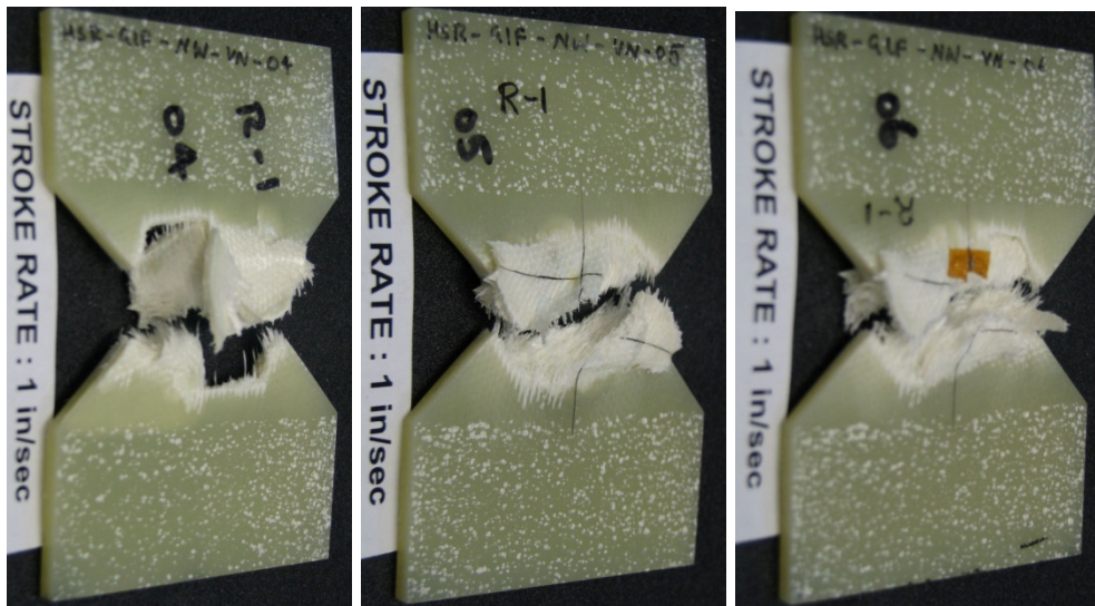
Figure E-3. Failure modes for fiberglass [0^\circ]_{12} at a speed of 1 in/s, in shear
