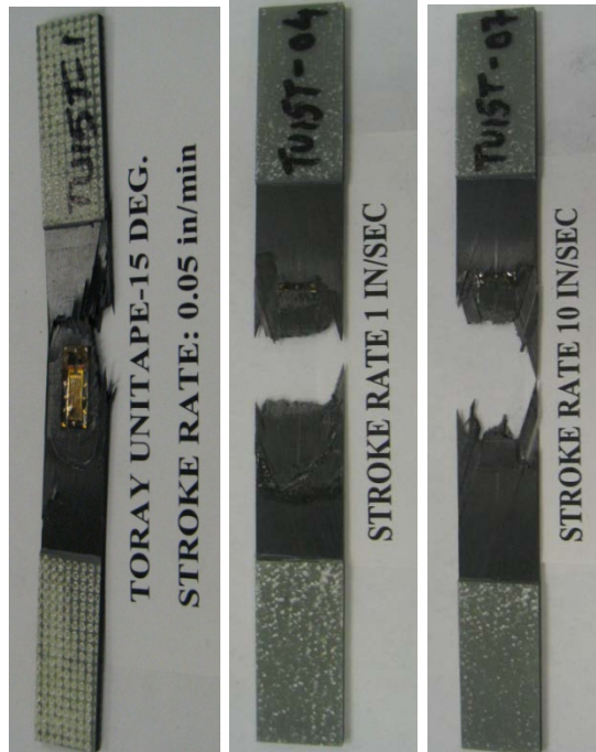
Figure C-15. Failure modes for carbon Unitape [15^\circ/-15^\circ]_{2S} : summary of all speeds, in tension
