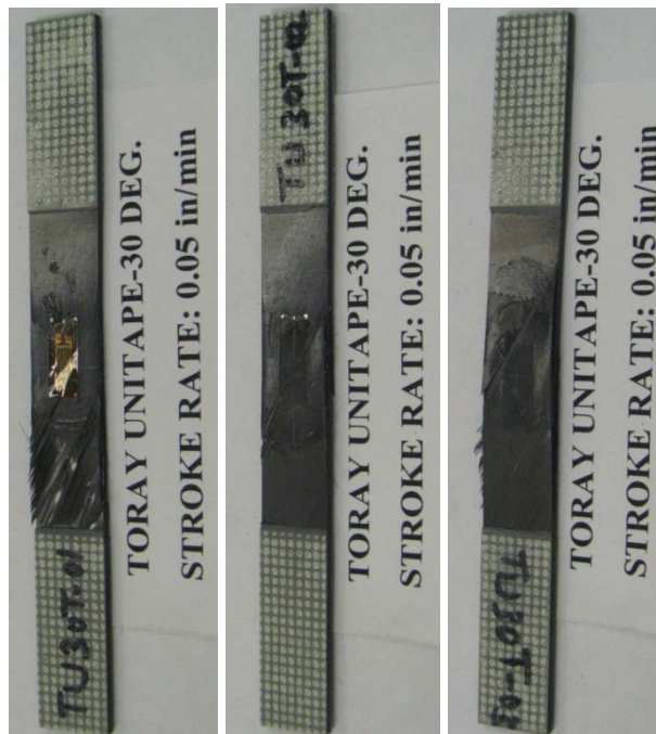
Figure C-17. Failure modes for carbon Unitape [30°/-30°] 2S at a speed of 0.0008 in/s, in tension
