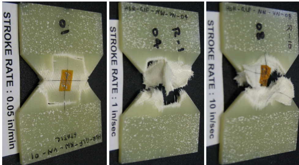
Figure E-7. Failure modes for fiberglass [0]_{12} : summary of all speeds, in shear
