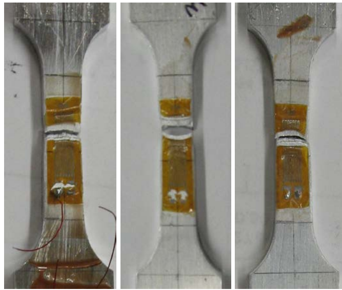
Figure A-9. Failure modes for aluminum 7075-T6 at a speed of 75 in/s
