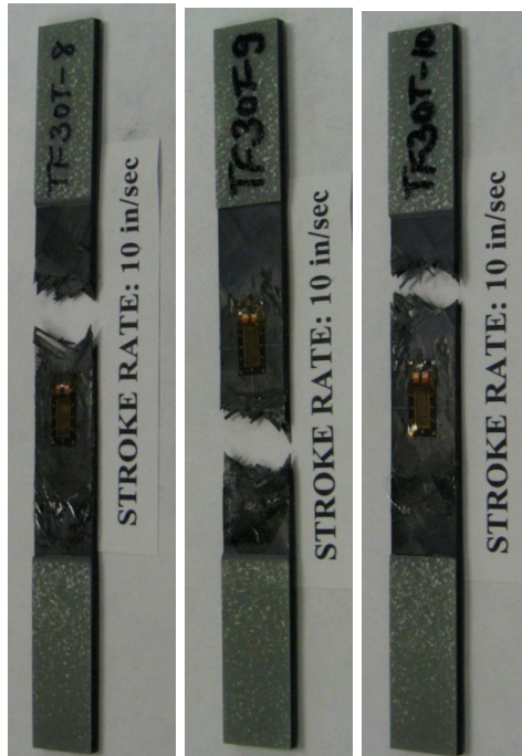
Figure D-21. Failure modes for carbon fabric [30^\circ/-30^\circ]_{2s} at a speed of 10 in/s, in tension
