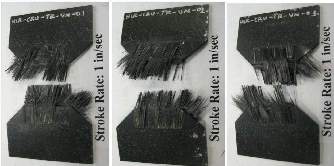
Figure F-2. Failure modes for carbon Unitape [0°] 12 at a speed of 1 in/s, in shear
