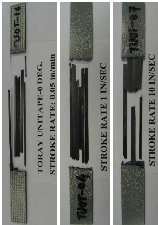
Figure C-7. Failure modes for carbon Unitape [0]_2 : summary of all speeds, in tension
