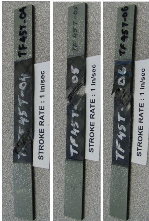
Figure D-27. Failure modes for carbon fabric [45^\circ/-45^\circ]_{2s} at a speed of 1 in/s, in tension
