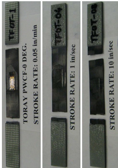
Figure D-7. Failure modes for carbon fabric [0^\circ]_4 : summary of all speeds, in tension
