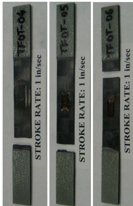
Figure D-3. Failure modes for carbon fabric [0^{\circ}]_4 at a speed of 1 in/s, in tension
