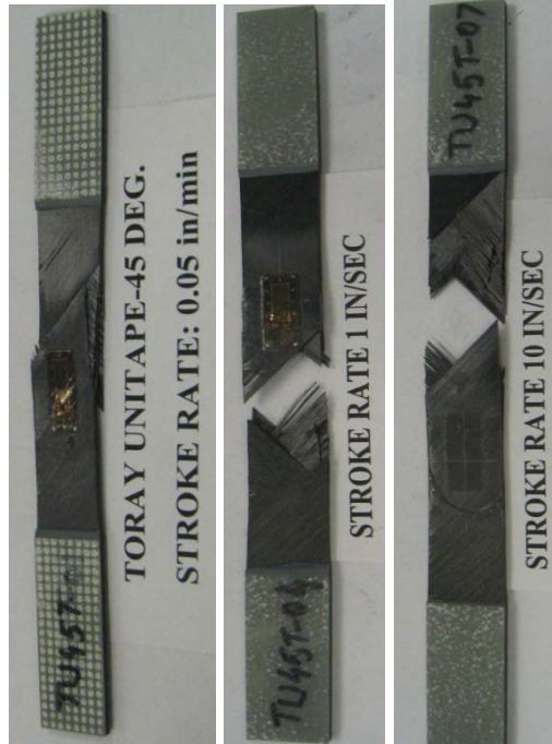
Figure C-31. Failure modes for carbon Unitape [45^\circ/-45^\circ]_{2S} : summary of all speeds, in tension
