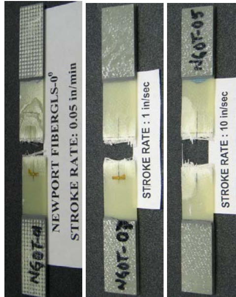
Figure B-7. Failure modes for fiberglass [0]4: summary of all speeds
