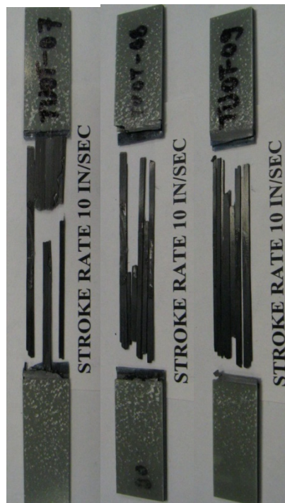
Figure C-5. Failure modes for carbon Unitape [0°] 2 at a speed of 10 in/s, in tension
