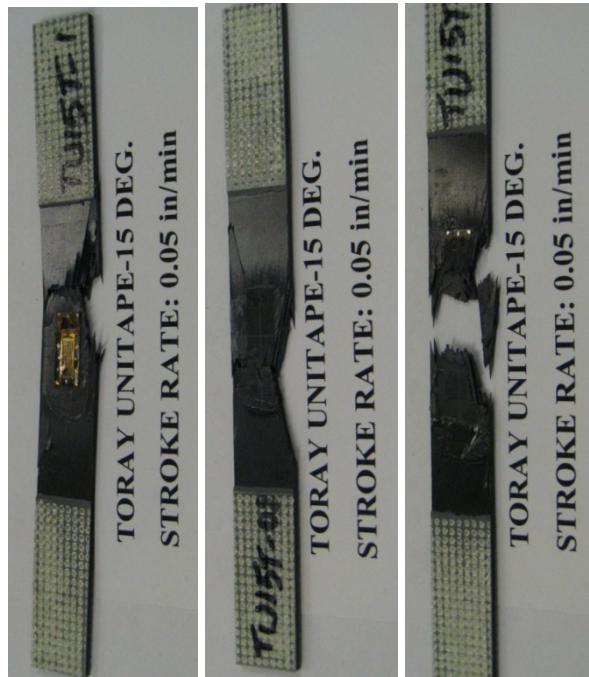
Figure C-9. Failure modes for carbon Unitape [15°/-15°] 2S at a speed of 0.0008 in/s, in tension
