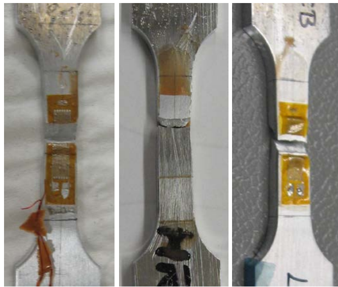
Figure A-3. Failure modes for aluminum 7075-T6 at a speed of 1 in/s
