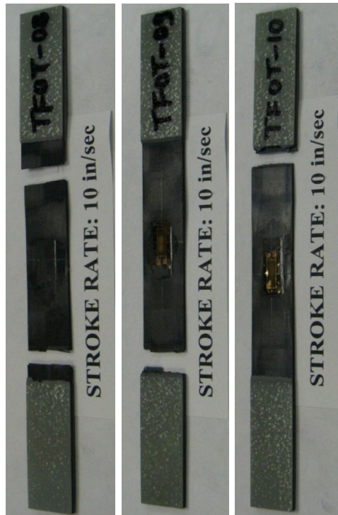
Figure D-5. Failure modes for carbon fabric [0°]4 at a speed of 10 in/s, in tension
