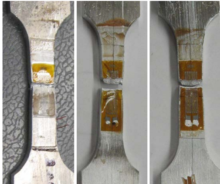
Figure A-1. Failure modes for aluminum 7075-T6 at a speed of 0.1 in/s
