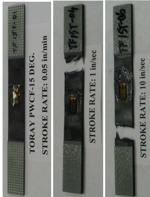
Figure D-15. Failure modes for carbon fabric [15^\circ/-15^\circ]_{2S} : summary of all speed, in tension
