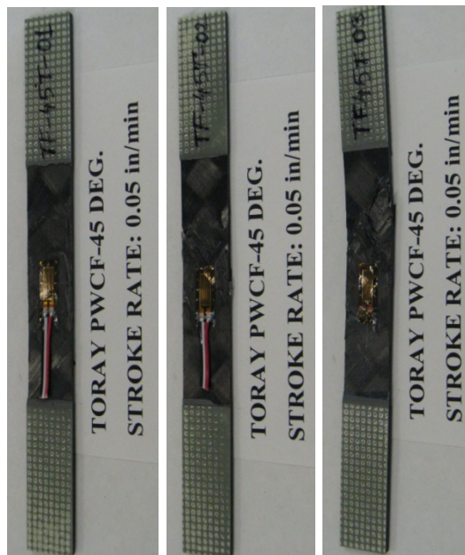
Figure D-25. Failure modes for carbon fabric [45°/-45°] 2S at a speed of 0.0008 in/s, in tension
