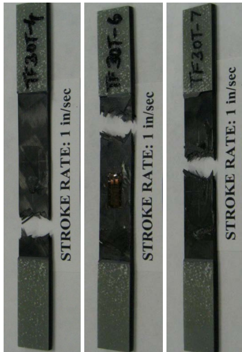
Figure D-19. Failure modes for carbon fabric [30^\circ/-30^\circ]_{2S} at a speed of 1 in/s, in tension
