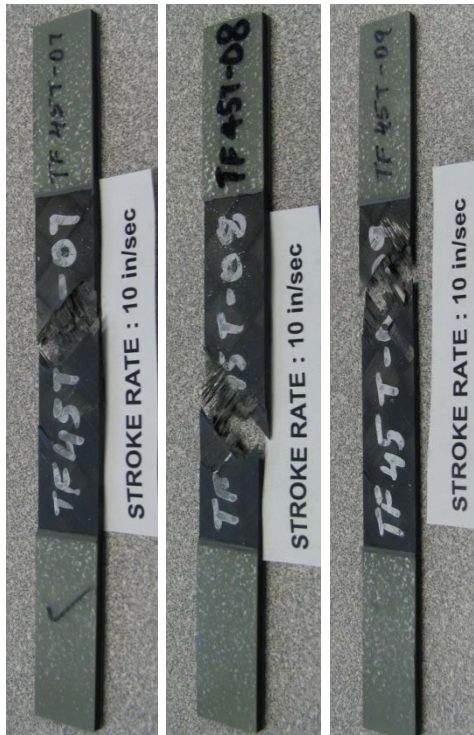
Figure D-29. Failure modes for carbon fabric [45°/-45°] 2s at a speed of 10 in/s, in tension
