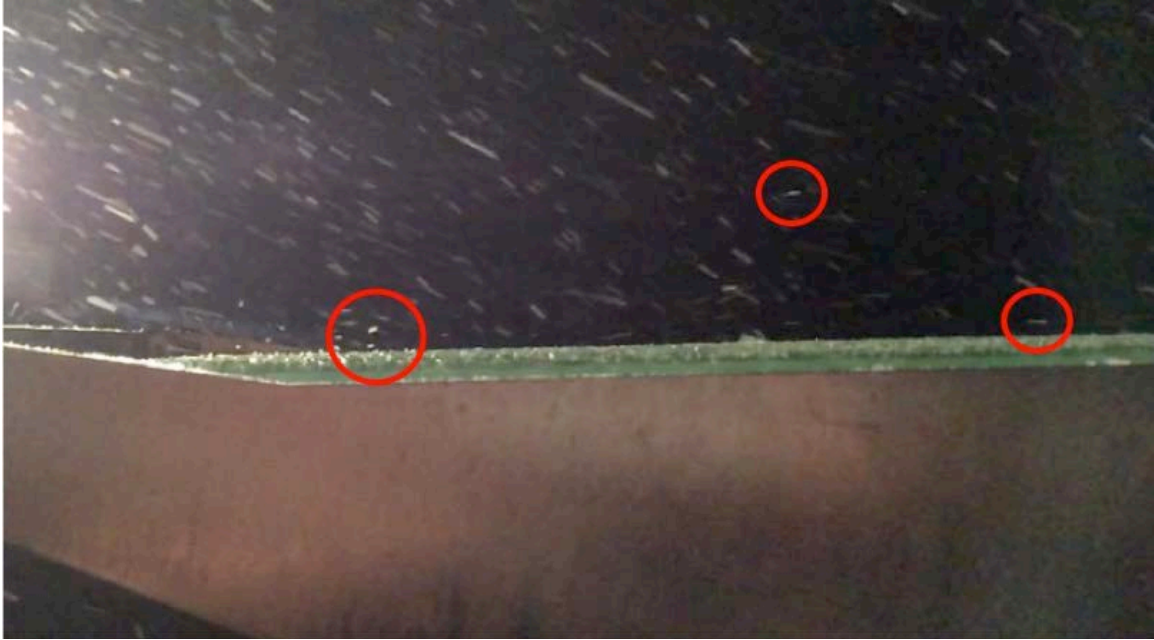
Figure 20. Photograph of snow particles bouncing (noted by streaks moving anti-parallel to the free-stream particles) when they hit the fluid surface
