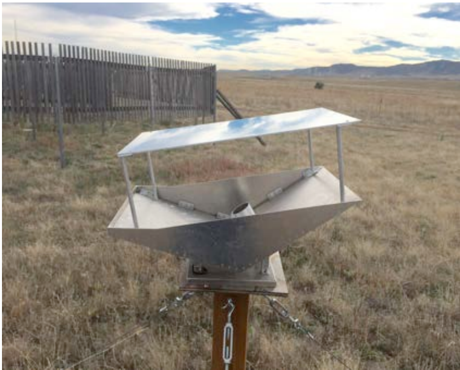
Figure 6. The outdoor tall frosticator assembly used in the free-stream environment
