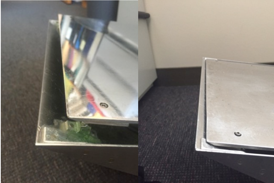
Figure 16. The modified height frosticator assembly used for testing in the snow machine (the standard assembly is shown to the right to emphasize the differences)
