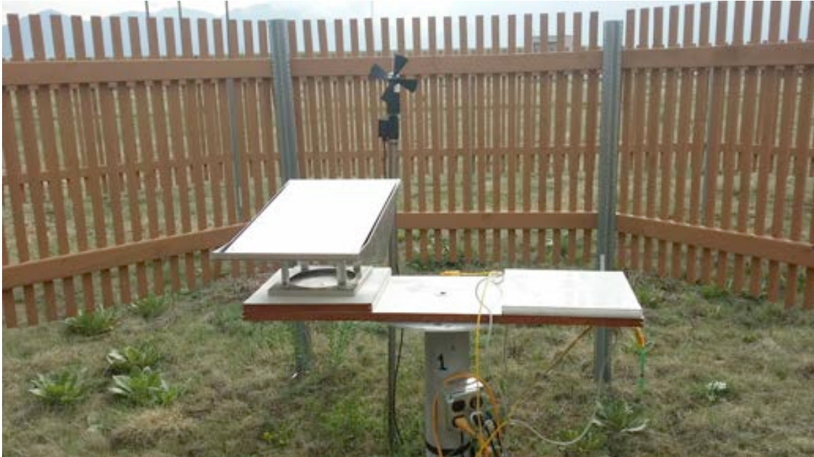
Figure 7. The standard frosticator assembly used in the DFIR shield
