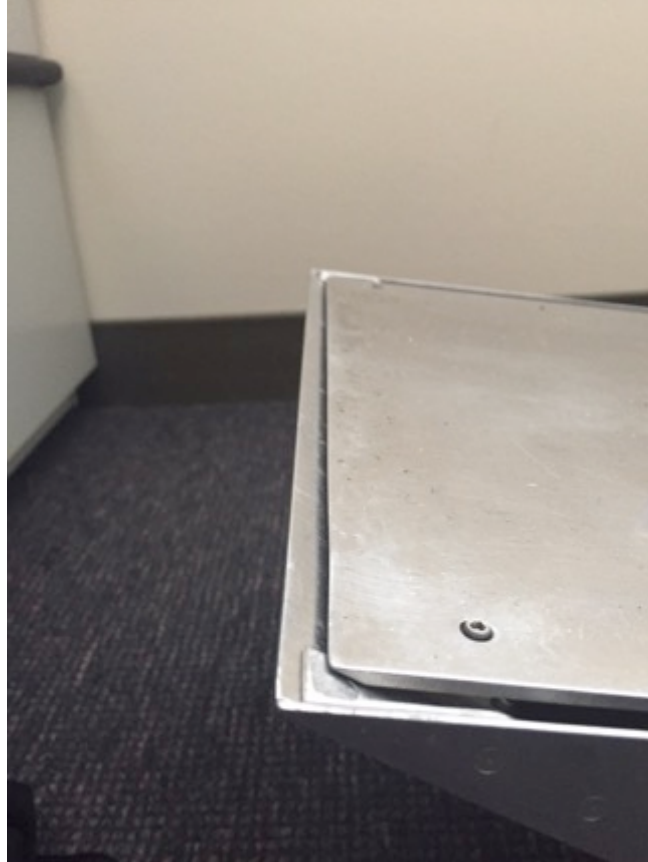
Figure 13. Close-up view of the top of the standard frosticator assembly showing the shallow gap between the tray and the frosticator plate
