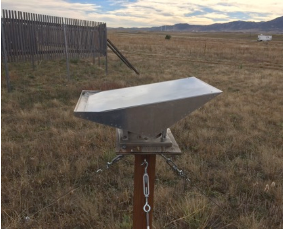
Figure 5. The outdoor standard frosticator assembly used in the free-stream environment
