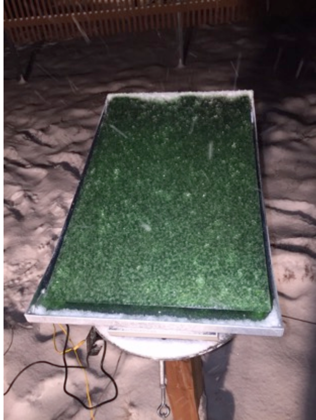
Figure 11. Snow buildup/fluid failure beginning near the top of the standard frosticator assembly at 0550 UTC
