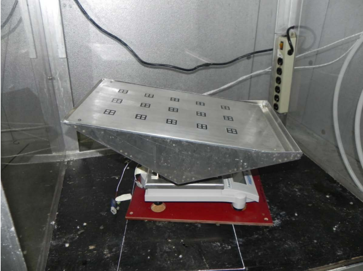
Figure 3. Indoor frosticator plate and tray assembly on a mass balance in the snow machine
