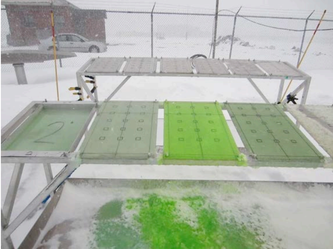
Figure 2. Outdoor frosticator plates used for anti-icing fluid testing and the corresponding rate pan, shown at far left with a drawn-in “2”
