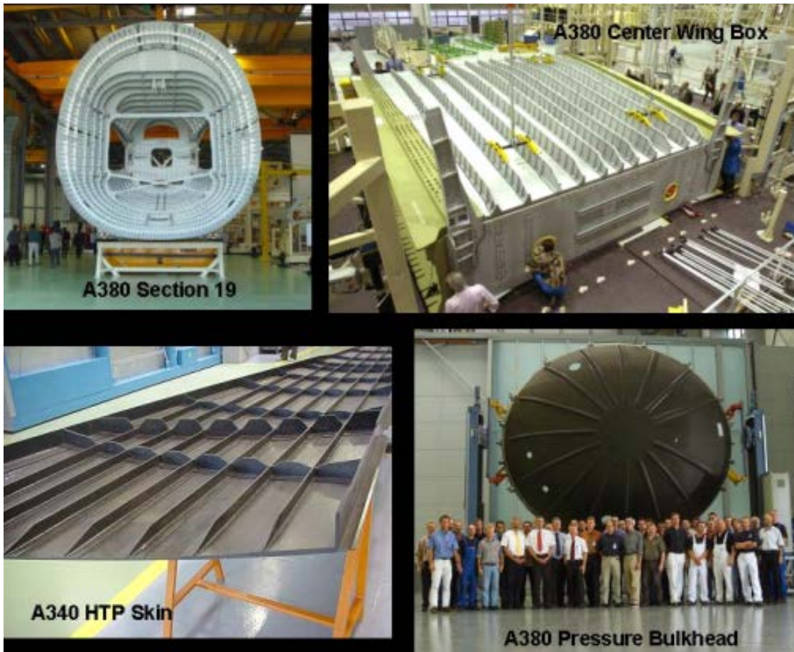
Figure 7. Summary of advanced composite applications on A380 primary structures
