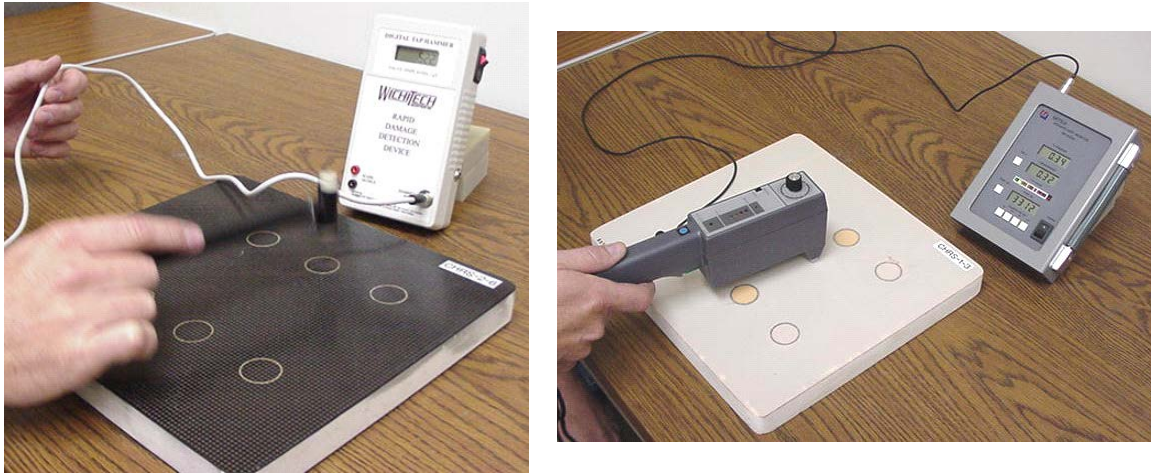
Figure 33. Instrumented tap test devices: DTH (left) and Woodpecker (right)
