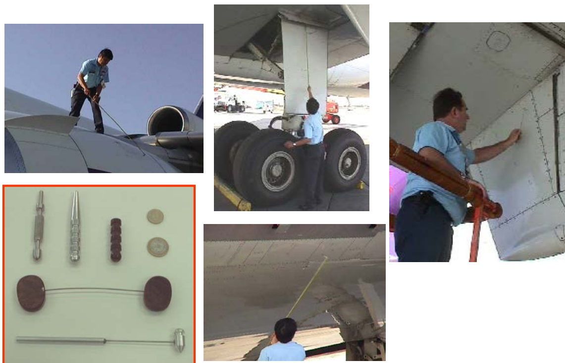
Figure 150. Sample tap testing at maintenance depots and alternative tappers identified in study
