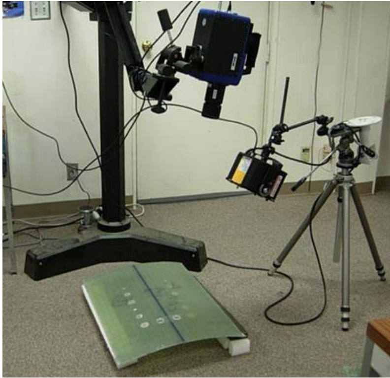
Figure 74. MoviTHERM lock-in thermography with halogen heat lamp being used as the excitation source
