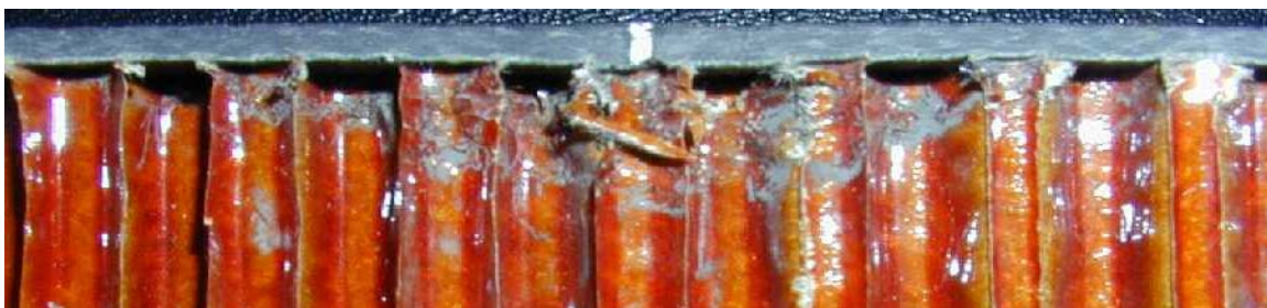
Figure 139. Cross-section of sample impact damage in composite honeycomb experiment panels showing crushed core but no skin deformation
