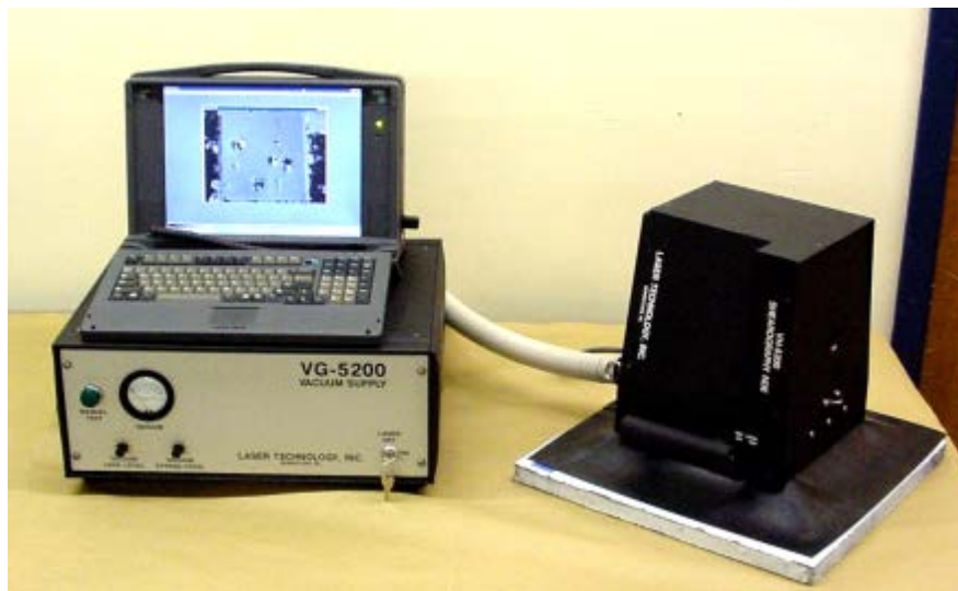
Figure 76. LTI-5200 portable shearography system with camera on test specimen
