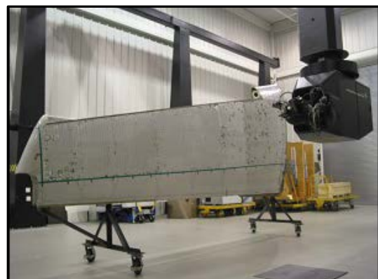
Figure 120. Schematic of laser UT method and deployment in gantry system and rail system
