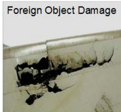
Figure 13. Sample sources of damage to composite structures
