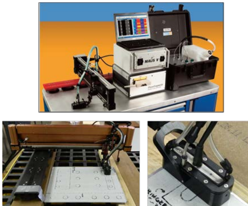
Figure 107. FlawInspecta linear array UT system deployed on MAUS V scanner platform—linear array UT probe includes a delay line shoe
