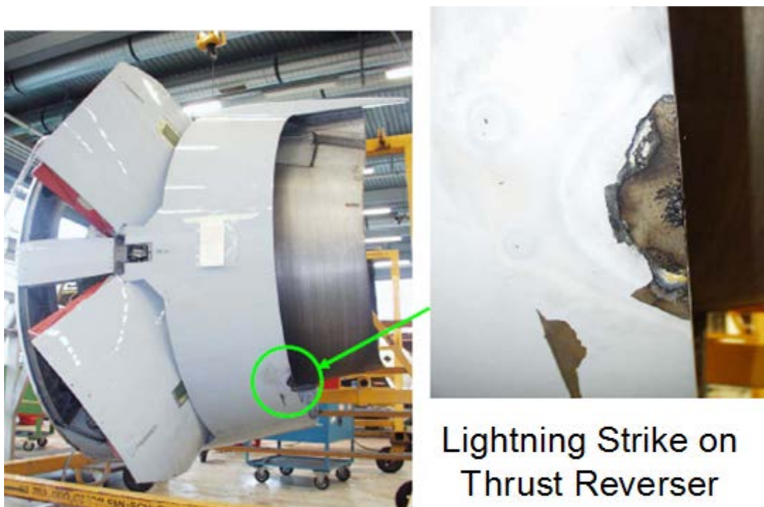
Figure 17. Sample damage from lightning strike
