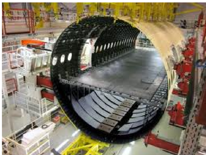
Figure 6. Production of an all-composite fuselage section
