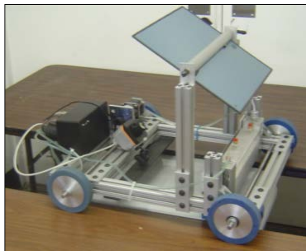
Figure 70. MISTRAS LST system—crawler used on composites
