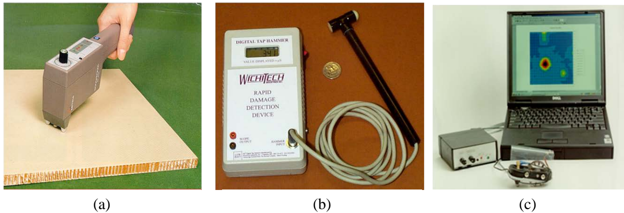
Figure 47. Three examples of instrumented tap test devices: a) Woodpecker, b) RD 3 , and c) CATT
