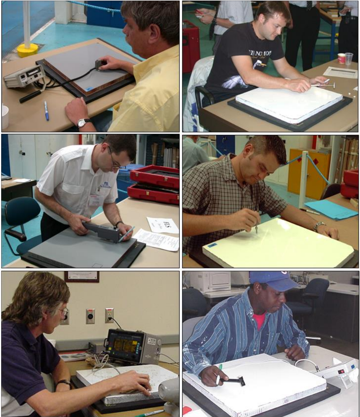
Figure 156. Inspectors completing inspections and marking flaw detections on the test specimens—clockwise from upper right: Airbus tap hammer, Boeing tap hammer, DTH, LFBT, Woodpecker, and MIA
