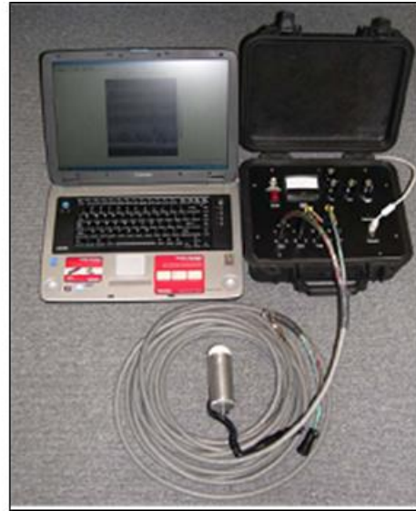
Figure 91. Basic equipment setup for microwave inspection
