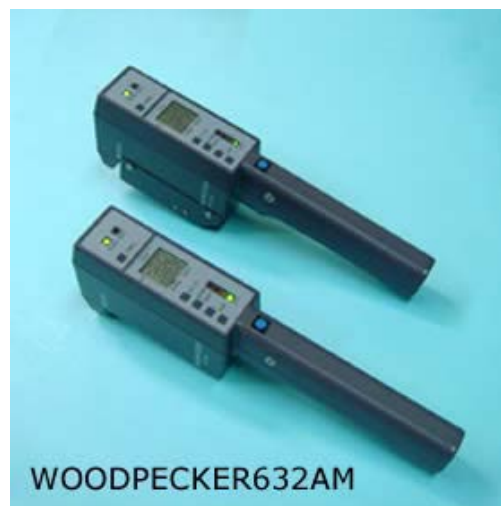
Figure 48. Woodpecker automated tap test device
