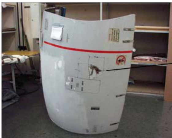
Figure 14. Sample damage from ground service vehicle impact
