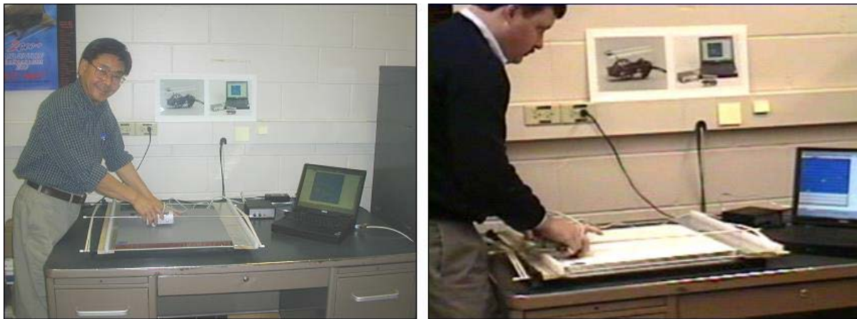
Figure 52. CATT system being deployed by Iowa State University developers on honeycomb flaw detection experiment test panels
