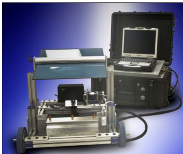
Figure 70. MISTRAS LST system—crawler used on composites
