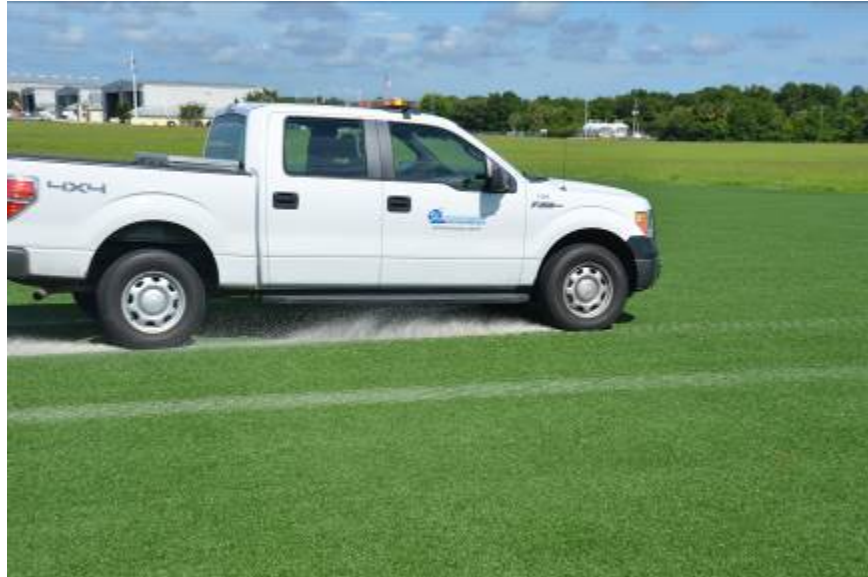
Figure 13. Sand Infill Material Displacement From Ops Truck Passage
