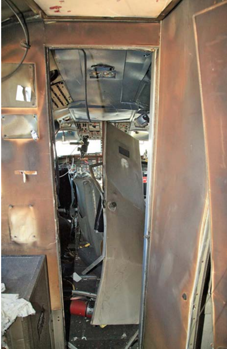
Figure 2. Aftermath of explosion of cargo compartment from lithium battery vent gases
