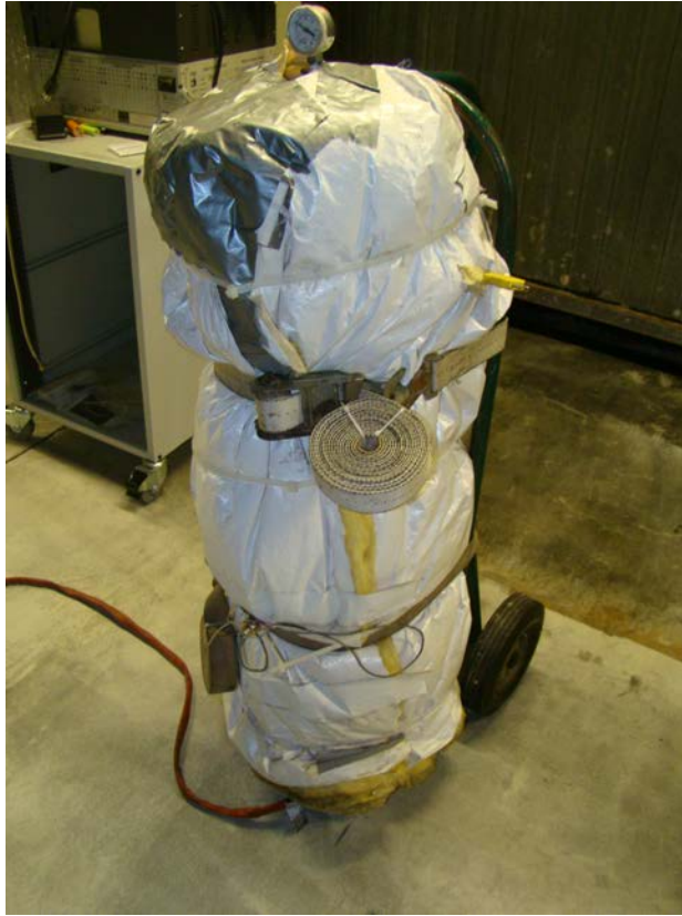
Figure 5. Auxiliary vent gas storage chamber
