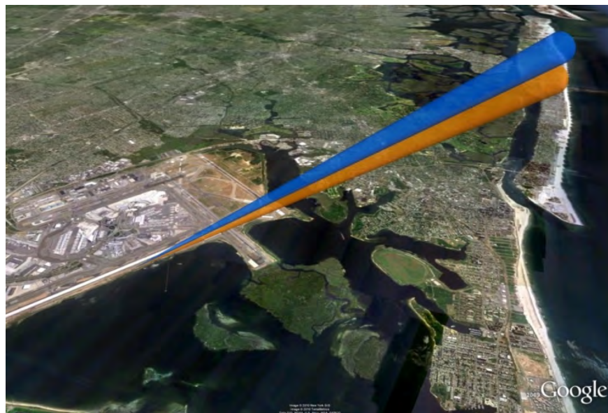
Figure 18. Example of Beam Projection for AR2 Parabolic Dish Antennas Shows the High Beam Projected by the AR2-2 (Blue) and the Low Beam Projected by the AR2-1 (Gold)
