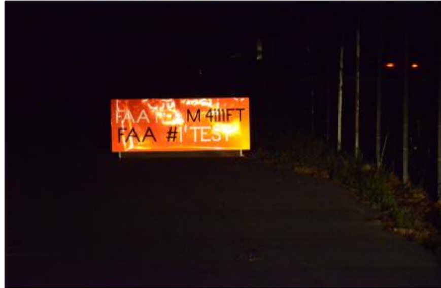
Figure 33. Nighttime Tests at the William J. Hughes Technical Center—With Black and White 8-in. and 9-in. Character Legends
