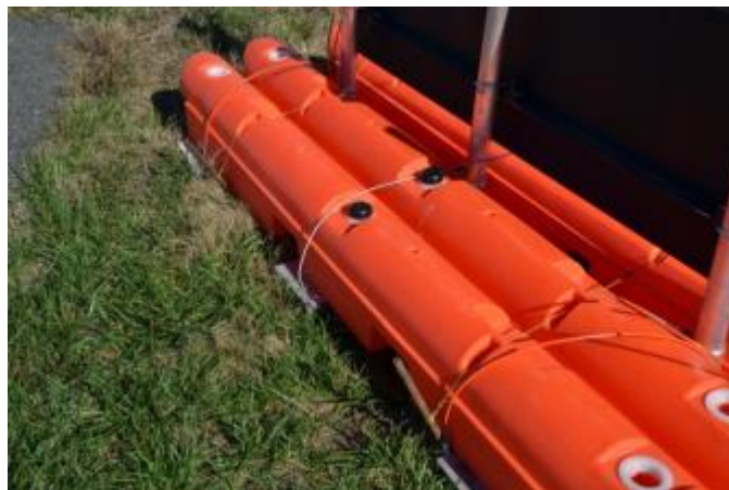
Figure 42. Tethers on Weighted Barriers
