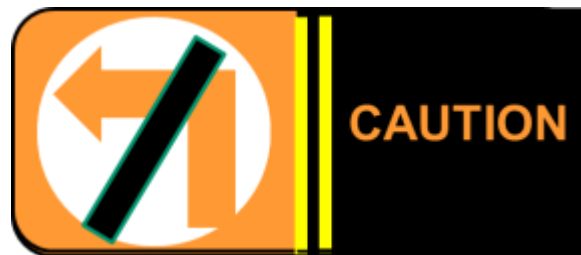
Figure 2. Early Stage Sign—CAUTION NO LEFT TURN
