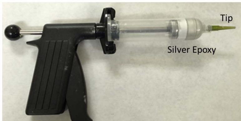
Figure 88. Handheld caulking gun containing silver epoxy
