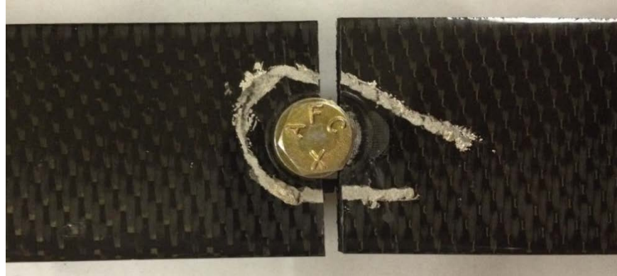
Figure 66. Filled-hole test specimen FHF-5 with silver epoxy bead conductive line after fatigue failure
