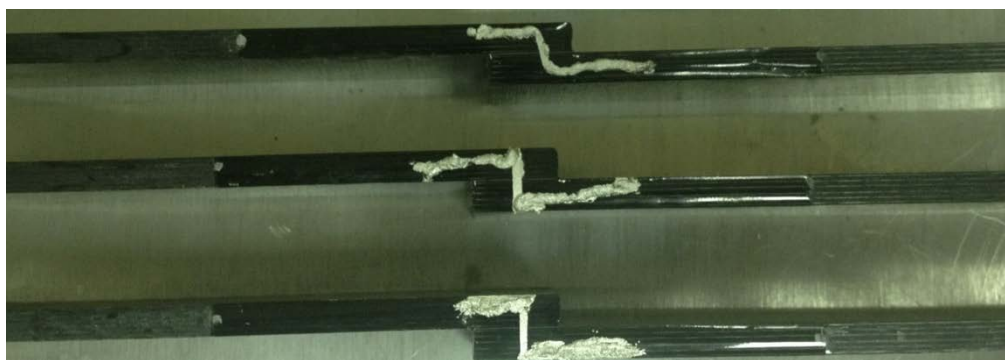
Figure 79. Lap shear test specimens with different types of silver epoxy adhesive conductive lines on epoxy-coated edges
