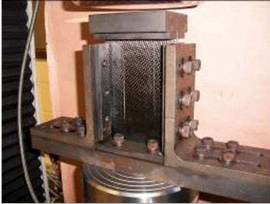
Figure 43. Specimen loaded into compression fixture prior to test
