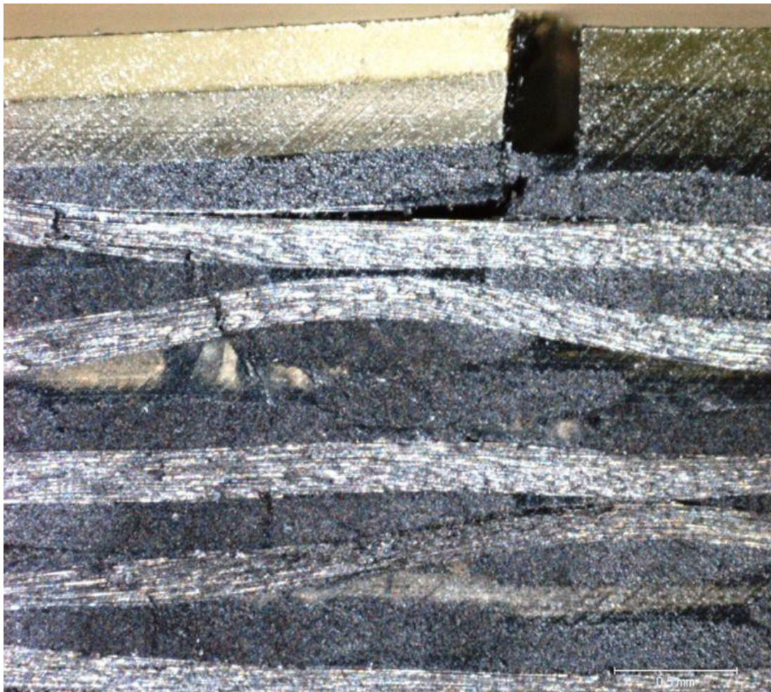
Figure 40. Cross-sectioned composite with crack in the epoxy-coated underside surface (top) from ASTM D7136 impact test
