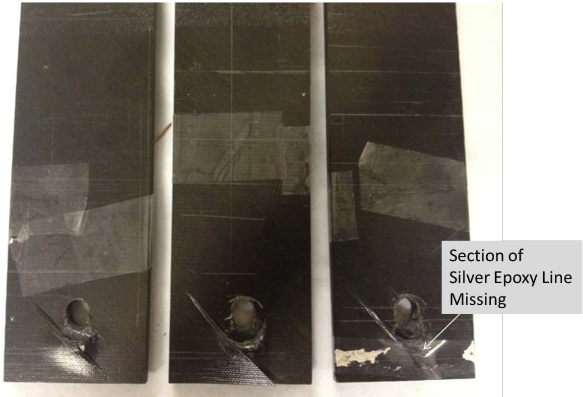
Figure 78. The back surfaces of ASTM D5961 failed test specimens
