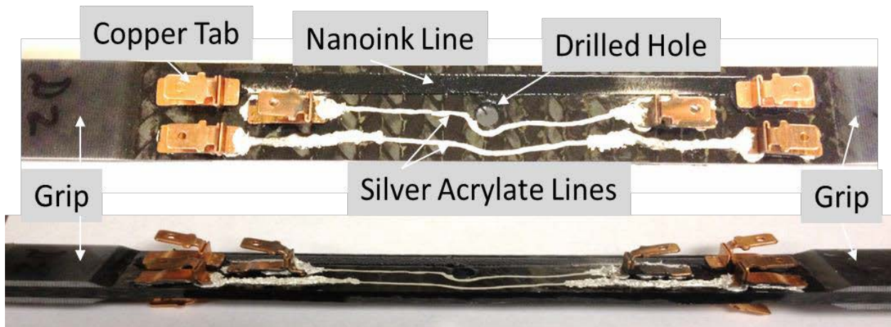
Figure 58. Fatigue test specimens with drilled hole (0.25") and conductive lines (nanoink and silver acrylate)
