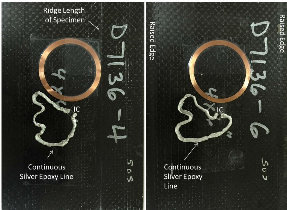
Figure 95. Representative ASTM D7136 test specimens with metallic mesh and Peel-N-Stick smart sensors
