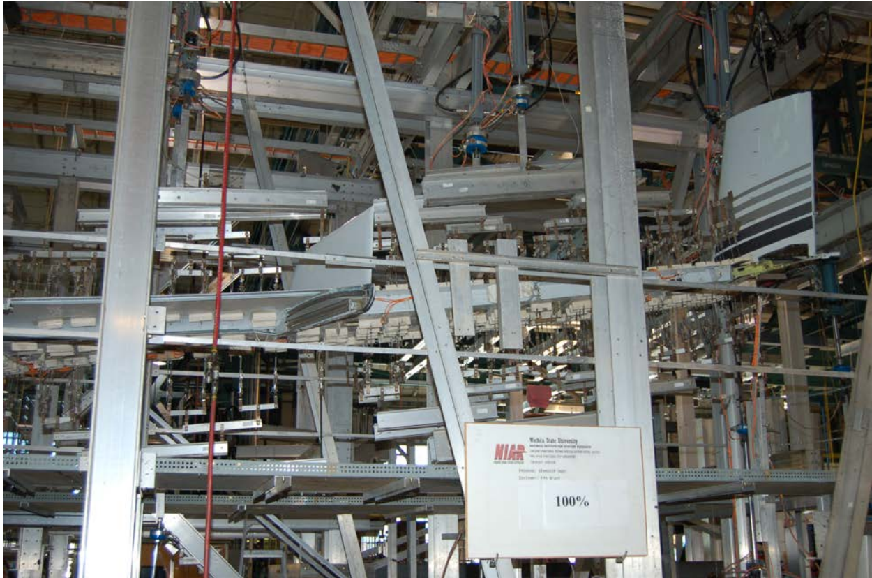
Figure 38. Deformed wing at 100% limit load
