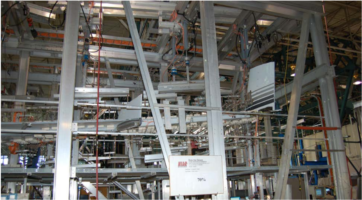
Figure 37. Deformed wing at 70% limit load
