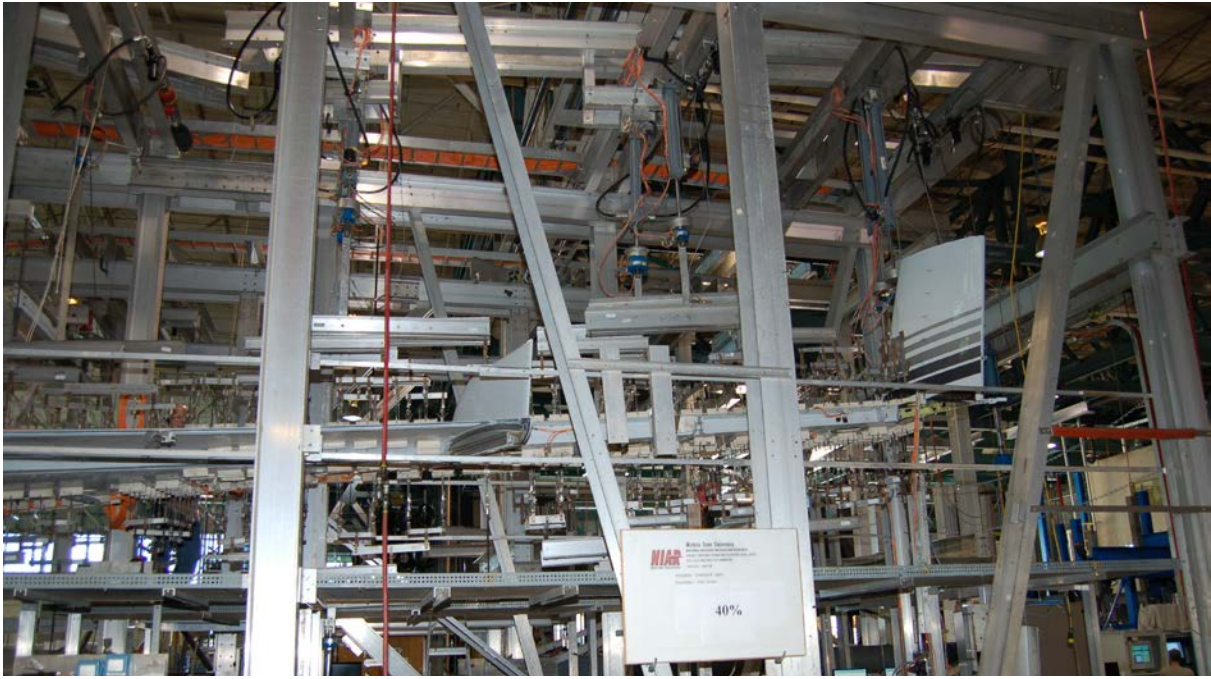
Figure 36. Deformed wing at 40% limit load
