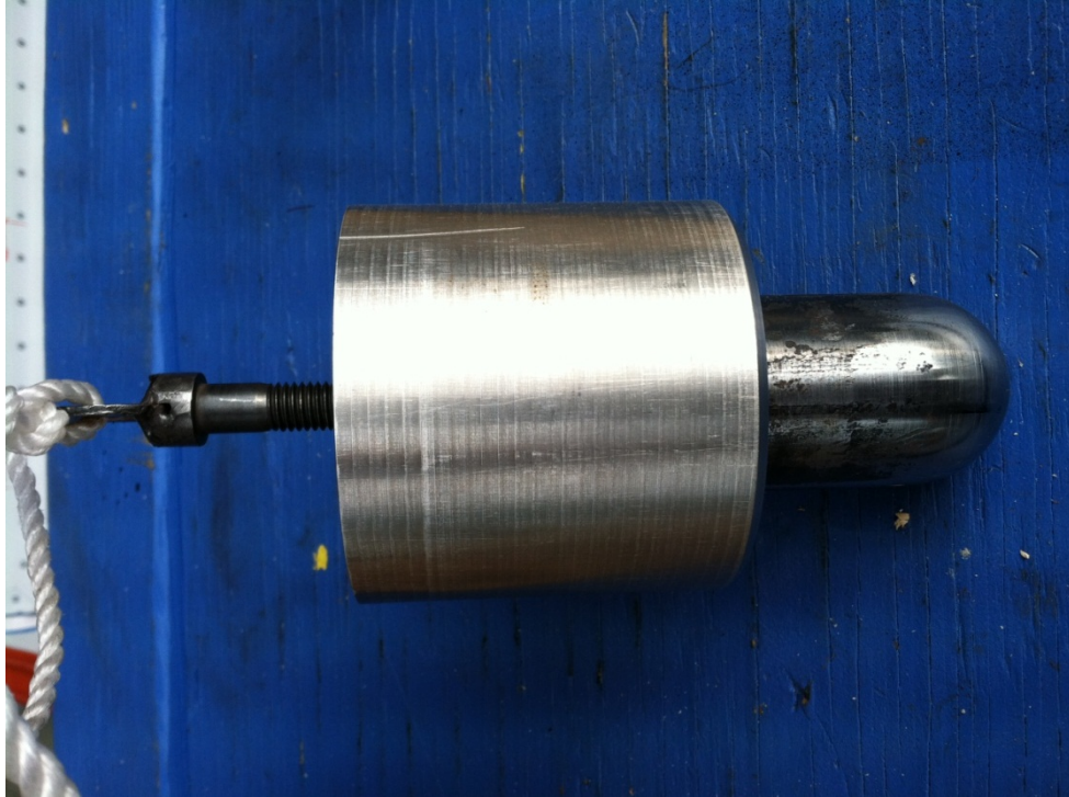
Figure L-2. The tup used for impact
