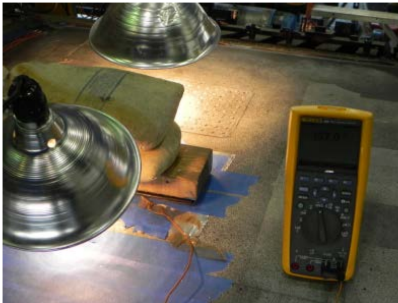
Figure I-5. Repair doubler curing at 150°F
