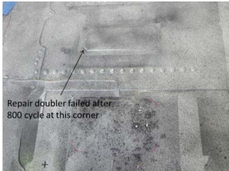
Figure I-6. Repair doubler failed at this corner after 800 cycles
