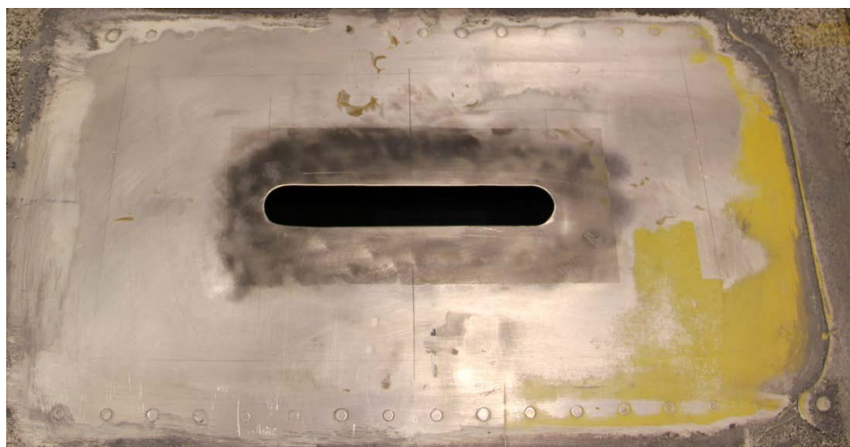
Figure K-2. The cut-out on the fuselage panel before repair installation
