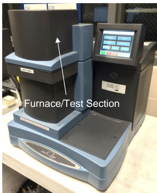
Figure A-1. TA instruments DMA Q800 furnace / test section [A-2]
