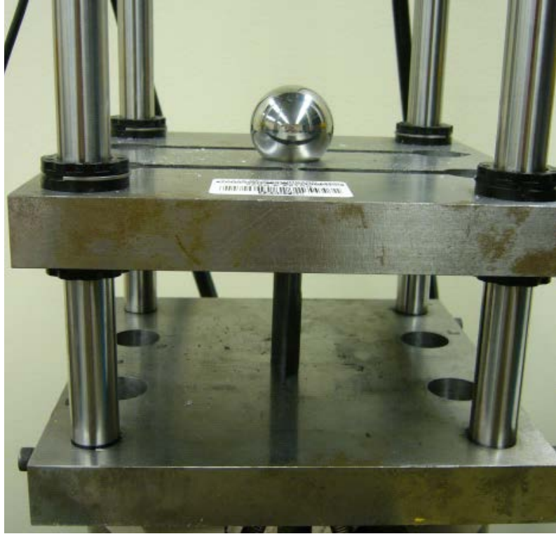
Figure 18. Crush coupon test fixture with corrugated specimen installed
