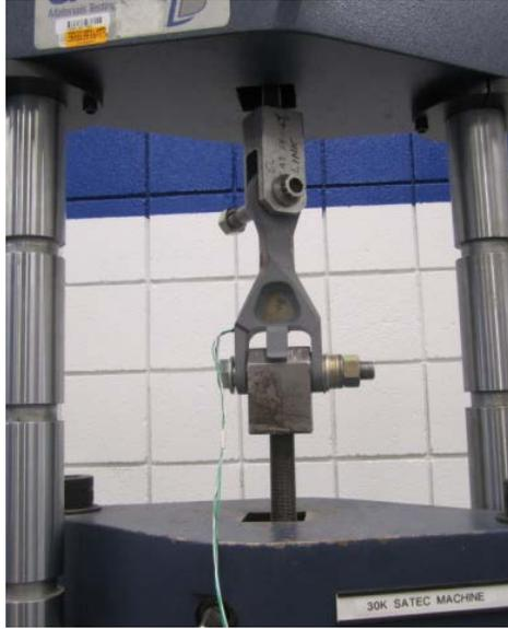
**Figure 4. Main rotor lateral servo link**
