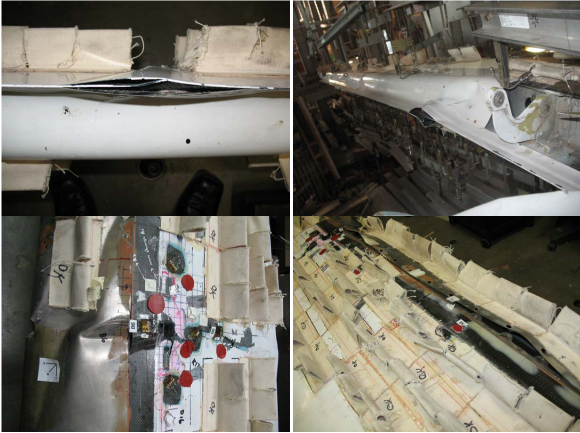
Figure 99. Post-test visual inspections of ST006 DaDT test article after residual strength test
