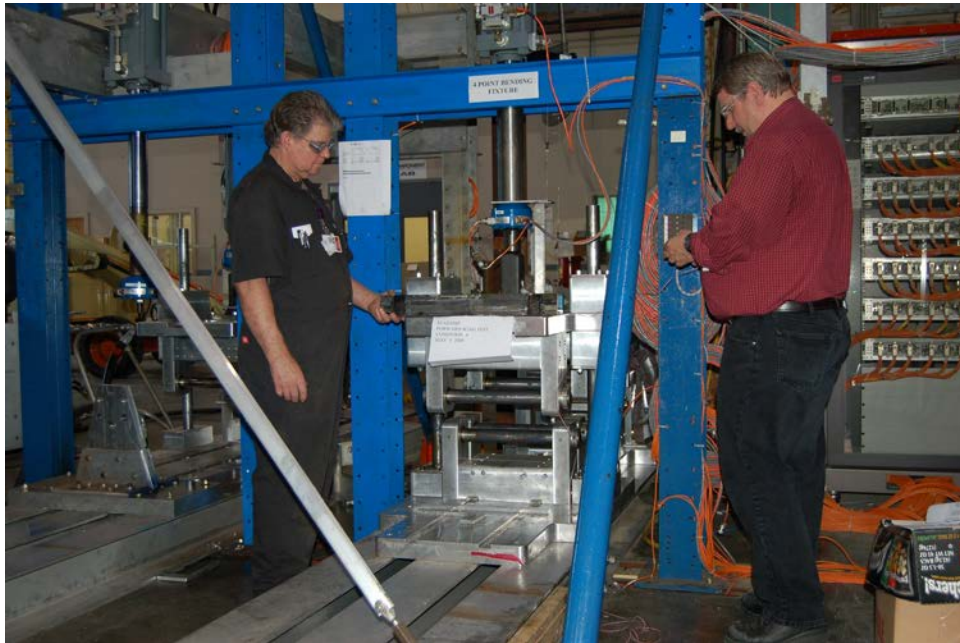
Figure E-4. 4PB element test setup
