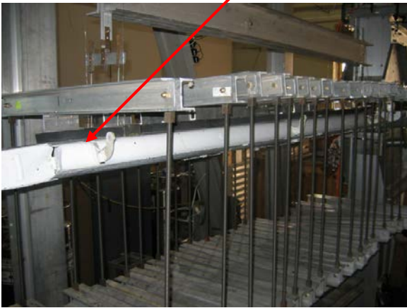
Figure C-2. Forward wing static test whiffletree setup with bonded load formers
