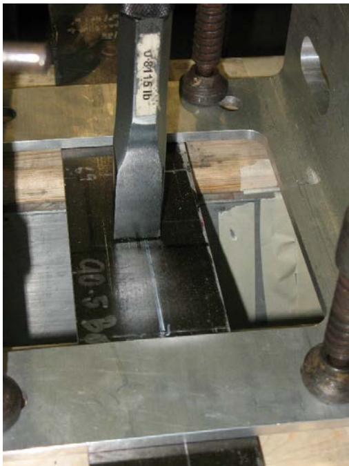
Figure E-3. Impact setup for 90.5B 4PB test specimen
