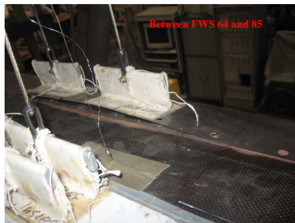
Figure 88. Leading-edge fastener-pullout failure (bottom surface) after 2 DLTs
