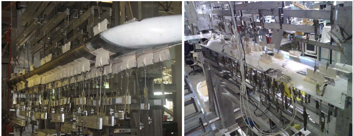
Figure 6. Full-scale fatigue test setup—load patches
