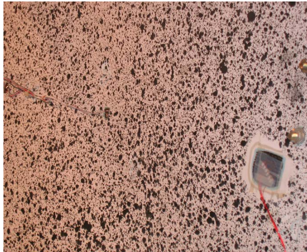
Figure 10. The ARAMIS photogrammetry system and speckle pattern
