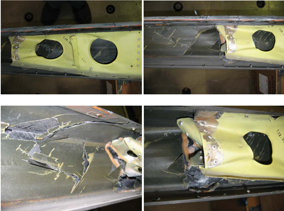
Figure 94. Post-test inspections of ST003 on removal of leading edge
