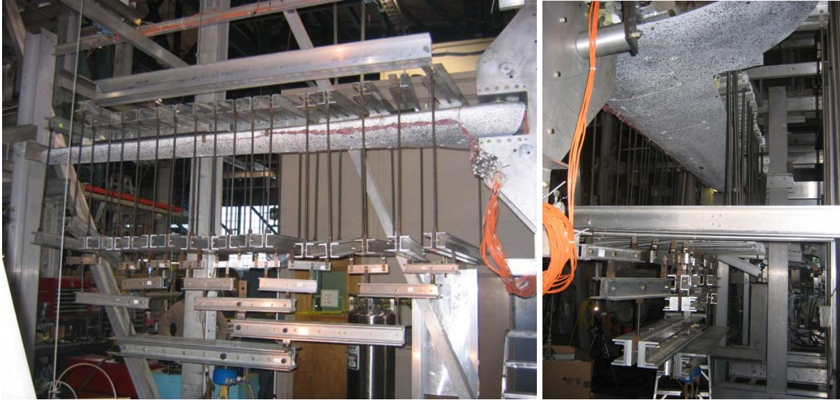
Figure 5. Full-scale static test setup—load formers
