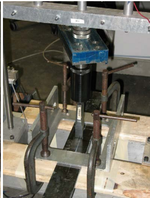
Figure E-3. Impact setup for 90.5B 4PB test specimen
