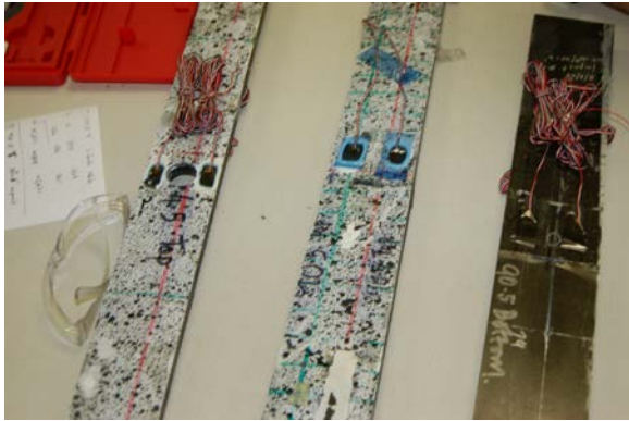
(a) Damaged 4PB elements (post-test)
