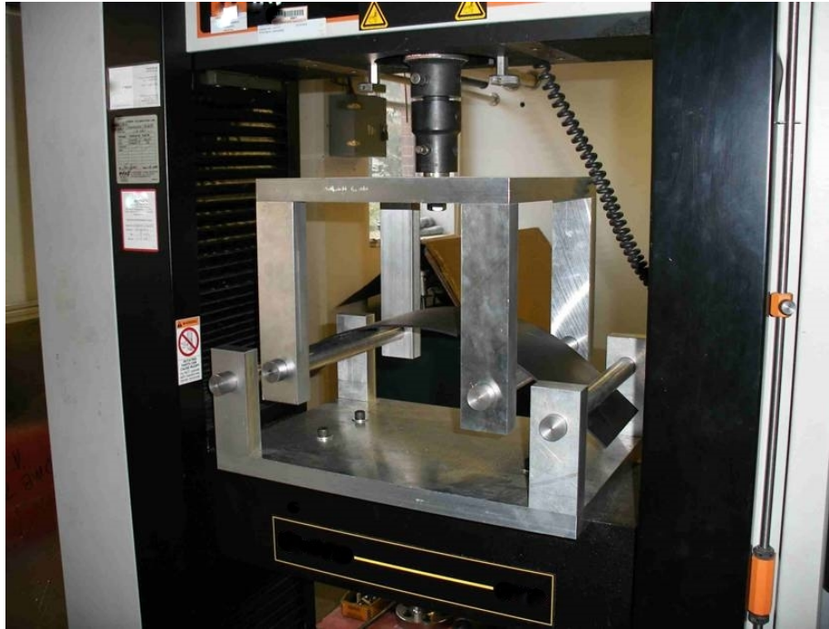
Figure 18. Four-point bending test fixture
