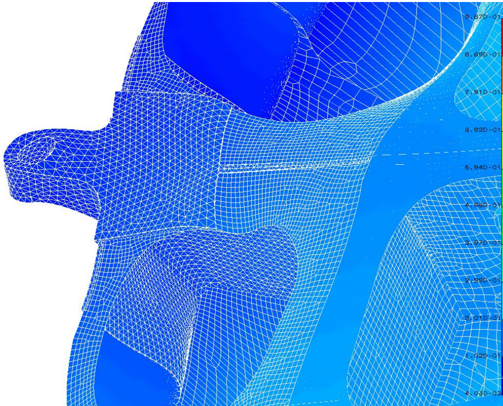
Figure 18. Deformed shape of the casting in the stop region (amplification factor of 500)
