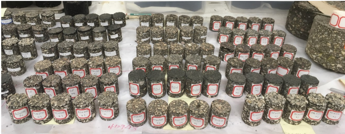
Appendix Figure 45. Partial view of 2-inch-treated pavement cores
