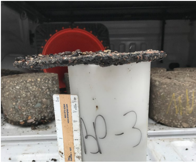
Appendix Figure 3. BP#3, partially damaged, 6-9 years
