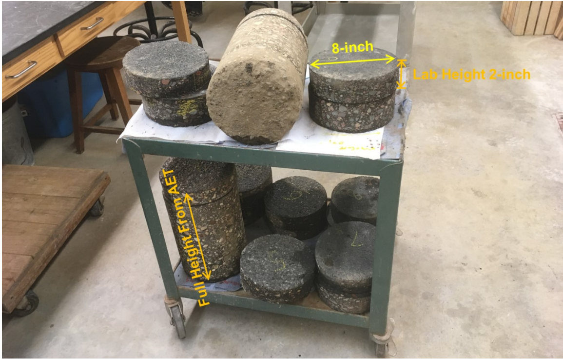
Appendix Figure 44. Height-treated pavement cores
