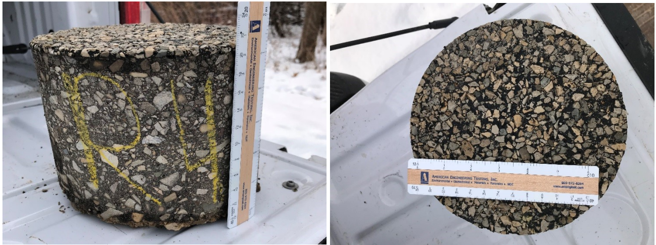
Appendix Figure 33. RCHSTR#4, partially damaged, 10-20 years
