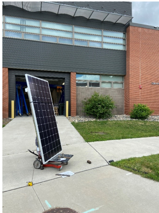
Figure 3.3 The assembled solar panels using the suggested connectors
