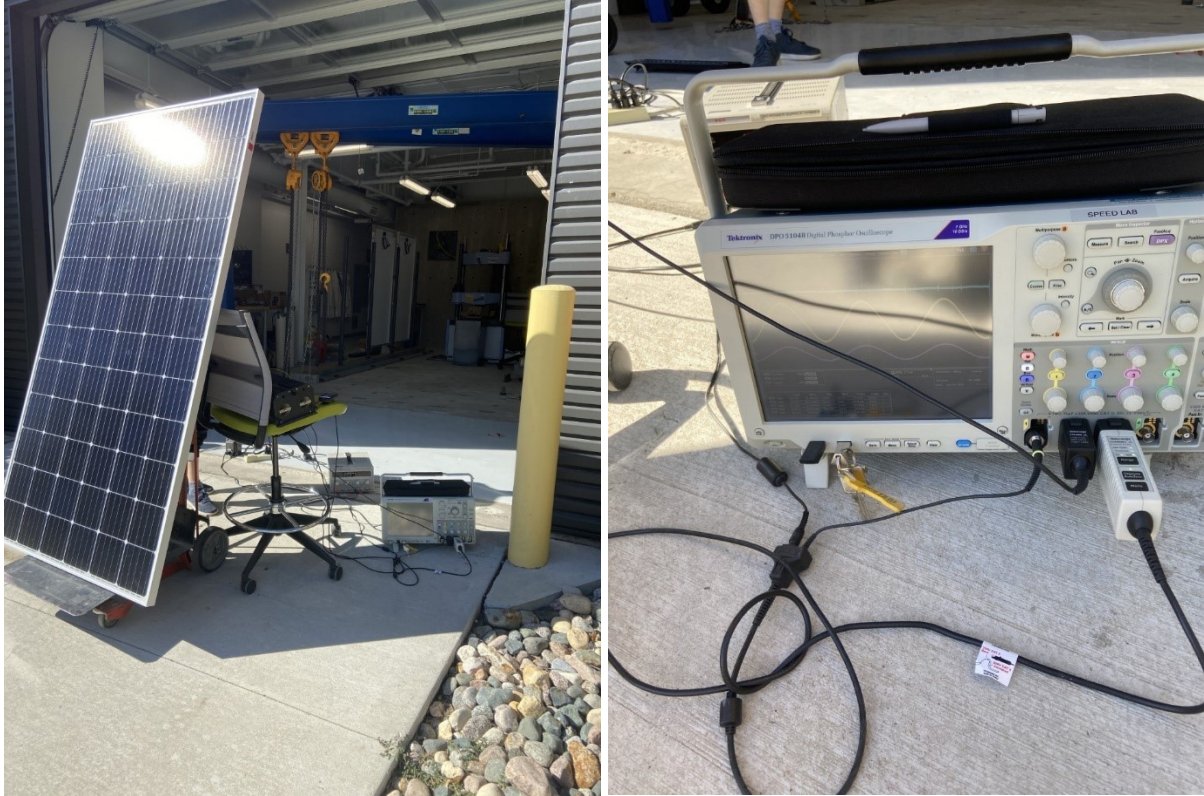
Figure 8.26 Testing the solar highway system with ambient sunlight
