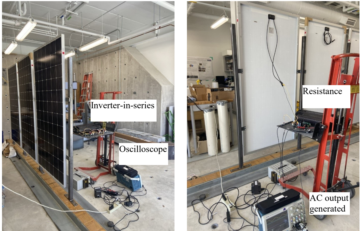
Figure 8.25 Prototype for the solar highway system
