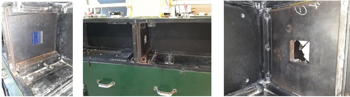
Figure 7.2 High-speed impact-test setup and the solar panel's broken pieces after the impact
