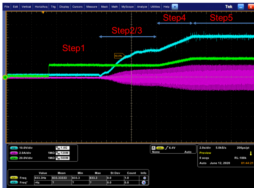
Figure 8.19 Single-inverter, soft-start experiment's waveform
