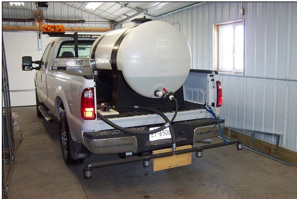
Figure 3.1 Pick-Up Truck Based Water Spray System
