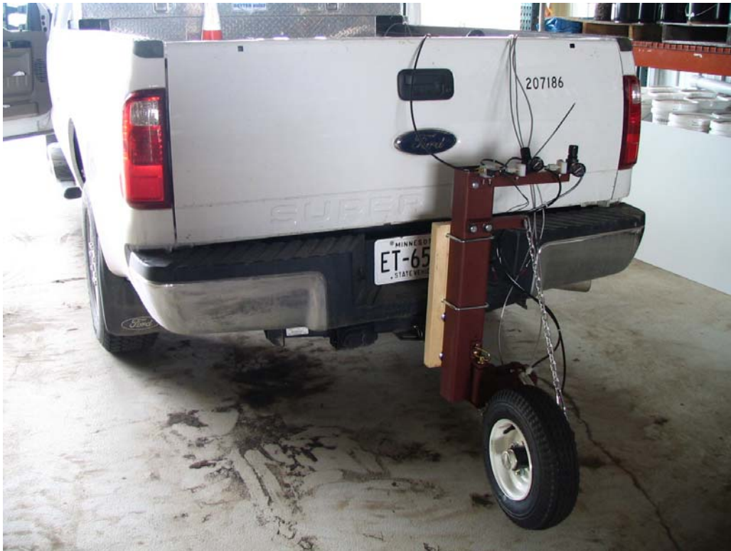
Figure 3.25 Friction Measurement System Installed on Pick-Up Truck
