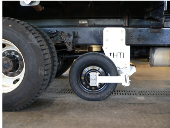
Figure 2.1 Photograph of the Norse Meter
