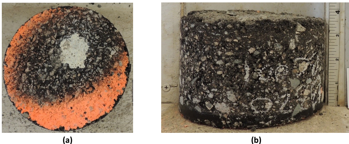
Figure 27. (a) Top and (b) side view of a pavement core from the outer lane of MnROAD Cell 133 (double chip seal, EE PG 58S-28)
