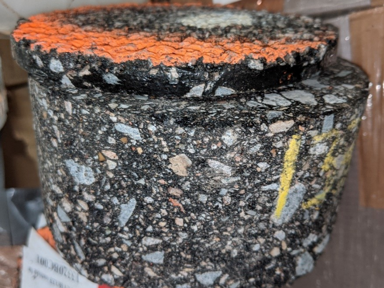
Figure 33. Processed core from MnROAD Cell 133 (double chip seal, EE PG 58S-28)
