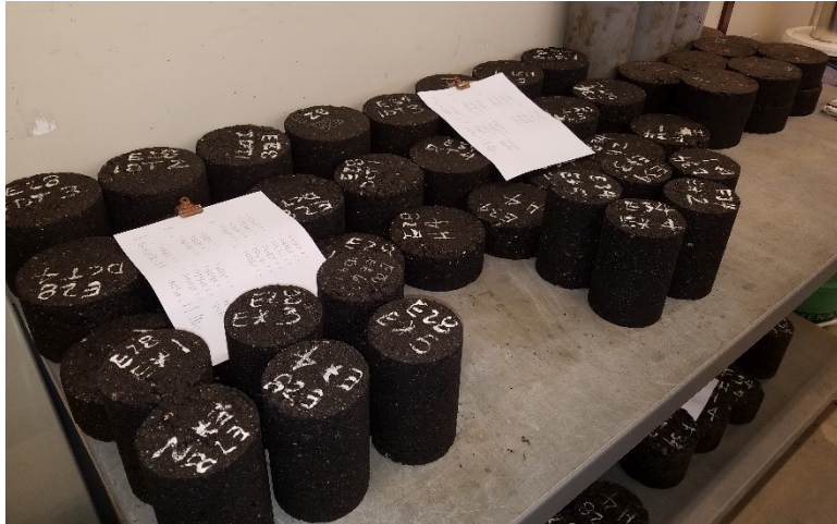
Figure 10. Laboratory batched, compacted CCPR mixtures for project tests
