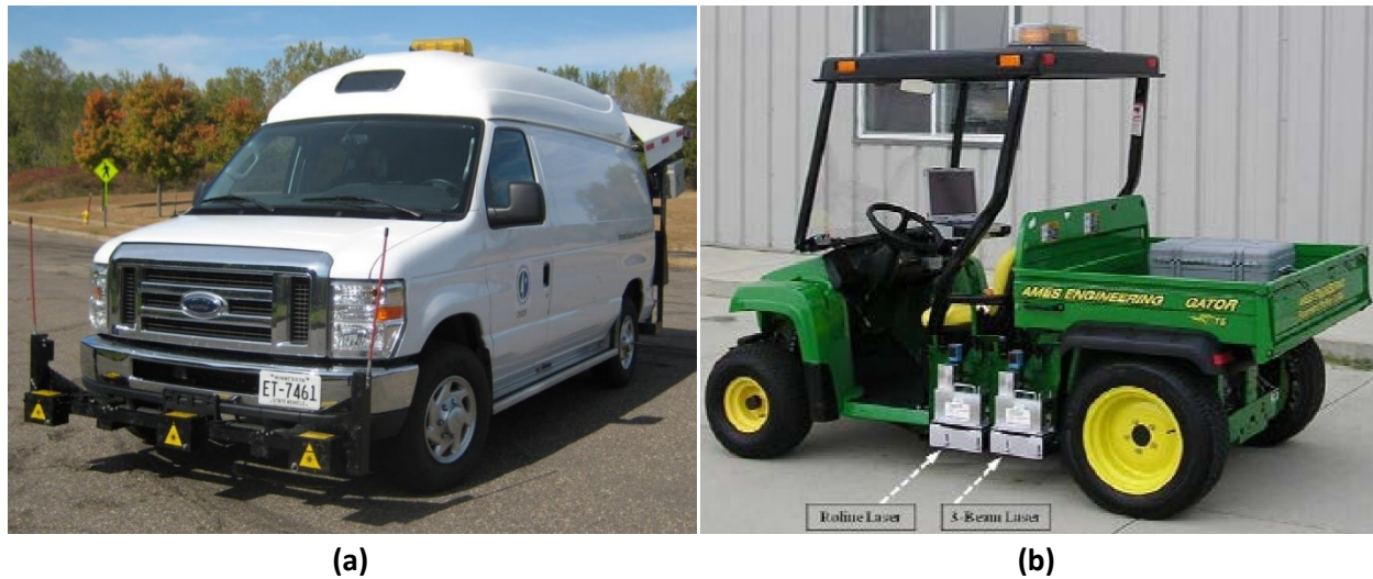
Figure 24. (a) Digital Inspection Vehicle and (b) vehicle-mounted LISA device to assess pavement condition and ride
