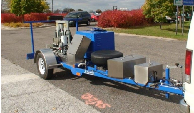
Figure 25. One of the trailer-mounted FWD test devices used at MnROAD
