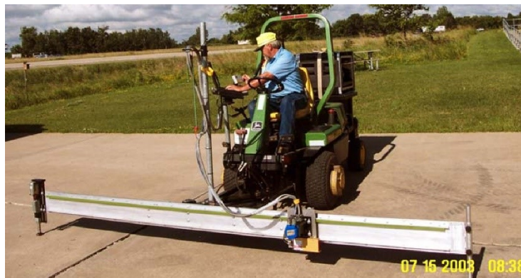
Figure 23. ALPS device mounted to a vehicle to provide rutting profiles for MnROAD test sections
