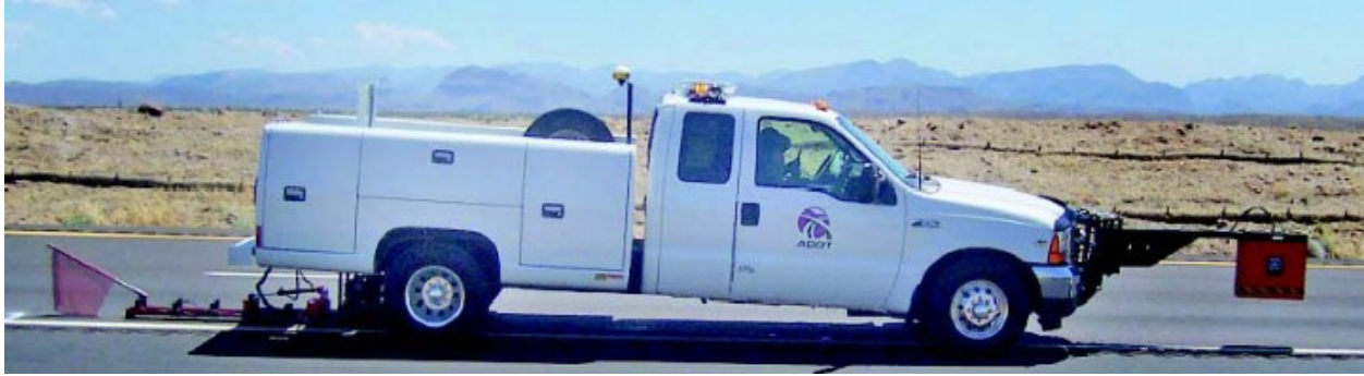
Figure 1. FWD vehicle integrated with GSSI GPR and horn antenna (Uddin, 2006)
