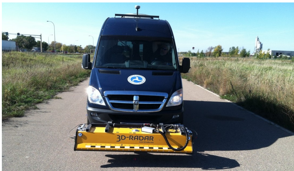
Figure 4. APE vehicle outfitted with 3D GPR system
