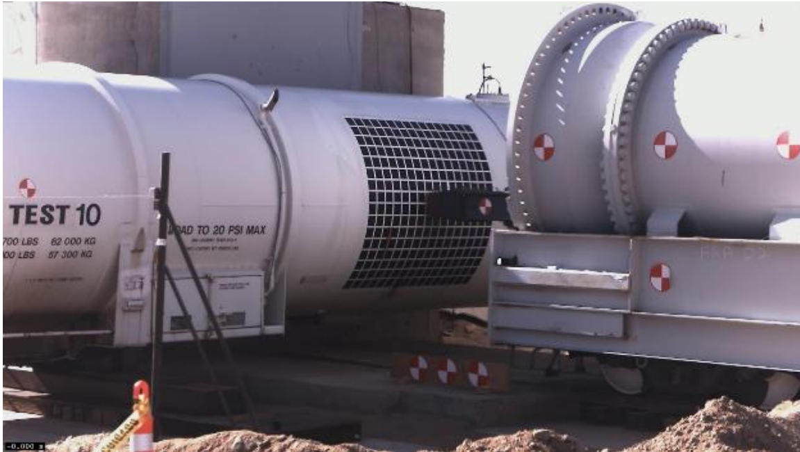
Figure 9. Ram Arm with 12-inch by 12-inch Indenter Aligned with Impact Zone on the Tank Car (Frame Extracted from High-Speed Video)
