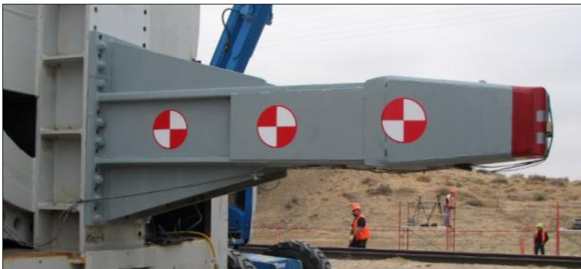
Figure 8. Ram Arm with 12-inch by 12-inch Indenter (Photo from Previous Test)
