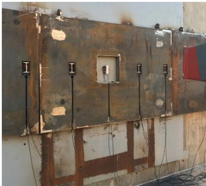
Figure 17. Laser Displacement Transducers on Crash Wall
