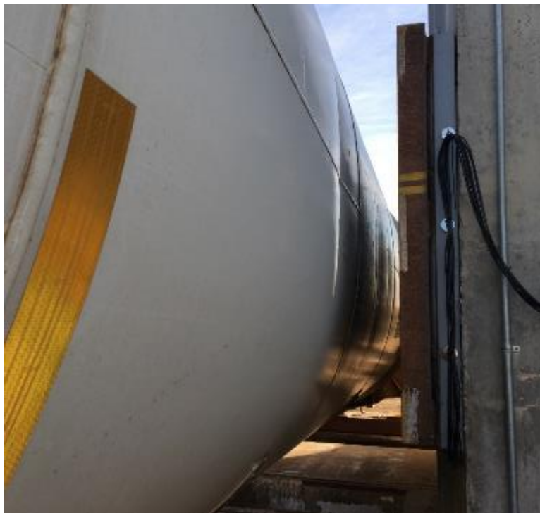
Figure 20. Post-Test Position of Tank Car (Wall Side)
