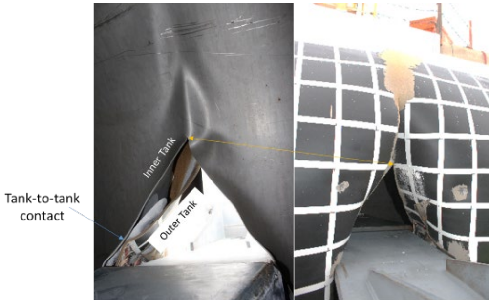
Figure 25. Interior (left) and Exterior (right) Views of Punctured Tanks Above Impactor (Prior to Impactor Removal)
