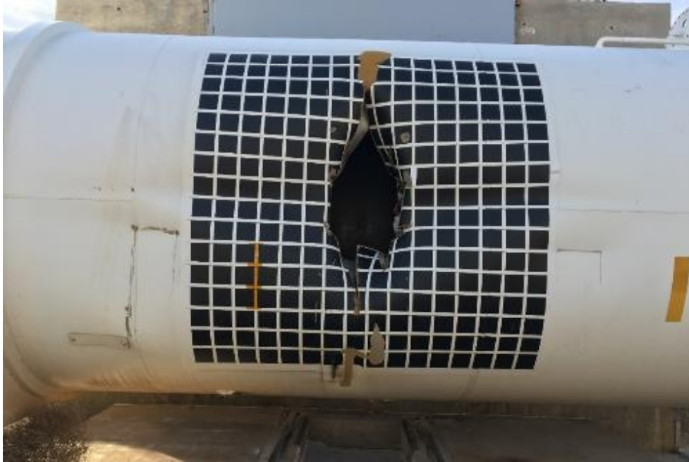
Figure 27. Tank Car After Impact (Impact Side, After Impactor Removal)
