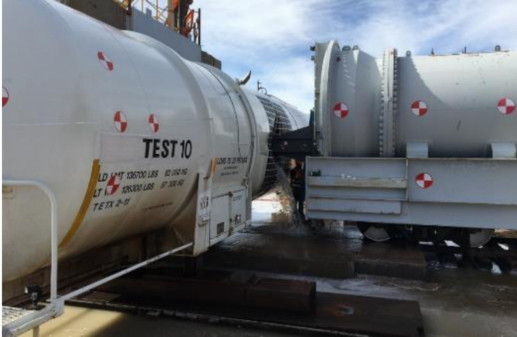
Figure 19. Post-Test Positions of DOT-113 and Ram Car
