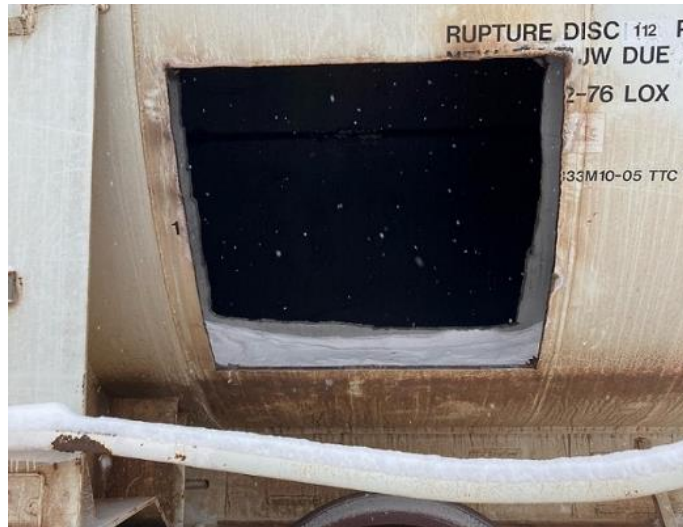
Figure 43. Photograph of DOT-113 with Area of Material Samples Removed Post-Test
