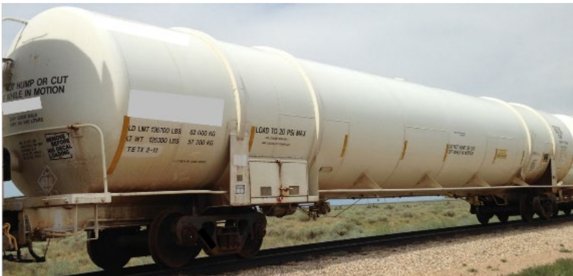
Figure 3. DOT-113 Tank Car Used in Test
