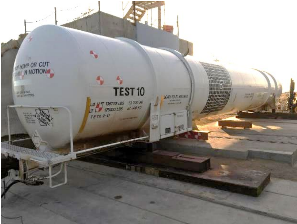
Figure 4. Target Tank Car Mounted on Support Skids
