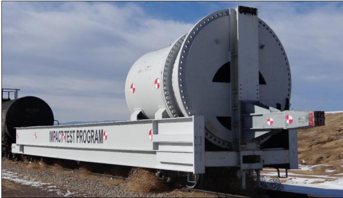
Figure 7. Ram Car and Head (Photo from Previous Test)
