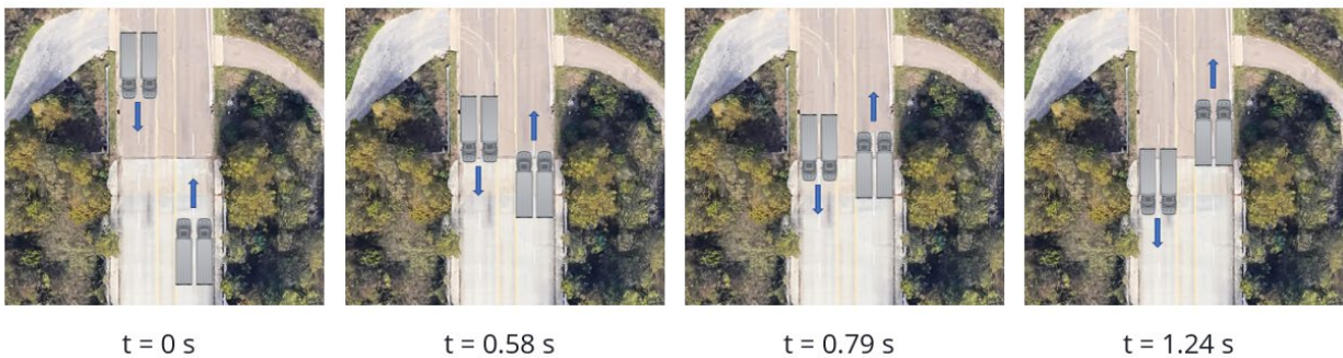
Figure 4-2. Position of AASHTO HL-93 truckloads with time
