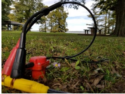
Figure 3-3 Vertical geophone with a corner frequency of 4.5 Hz
