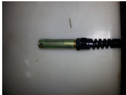
Figure 3-7. The trigger that attaches to the sledgehammer and signals the hit time
