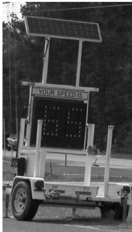
Figure B2. Mobile, lighted DSFS that displays speed without flashing. (Speed displayed for all drivers.) (Bullough et al., 2012)
