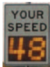
Figure B5. Static, lighted DSFS that displays speed and flashes. (Santiago-Chaparro et al., 2012)
