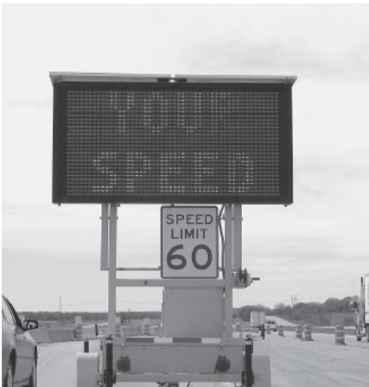
Figure B3. Mobile, lighted, DSFS with multiple messages prior to display of speed – no flashing. [(a) default DSFS message for non-violations; (b) first pass phase for violators; (c) second pass phase for violators; and (d) final phase for violators.] (Brewer et al., 2006)
