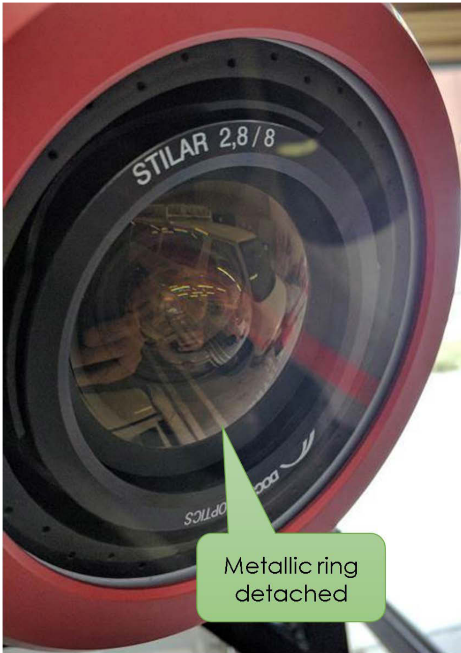
Figure 2.5: Close-up view of VMX-1HA Camera 2 lens. The metallic ring detached from the lens and contacted the camera housing glass cover.
