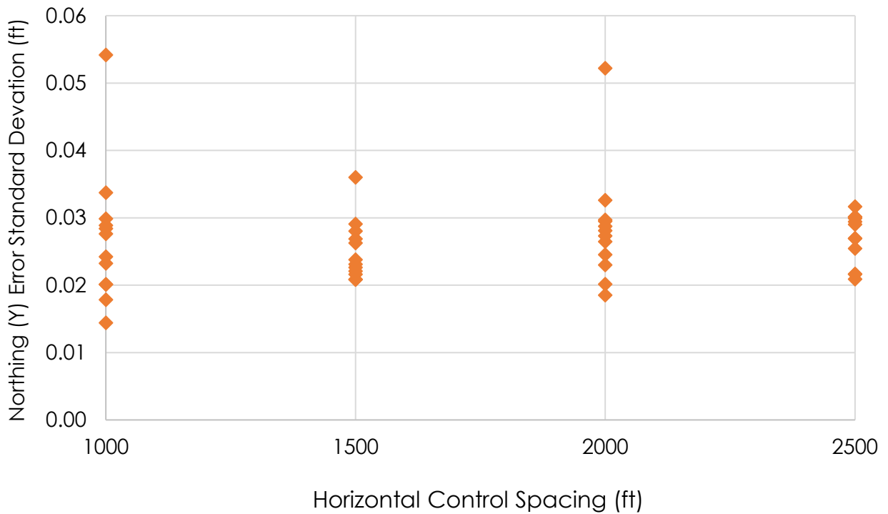
Figure 6.9: Left laser Northing (Y) standard deviation of each pass traveling on number 1 lane at various registration control spacings
