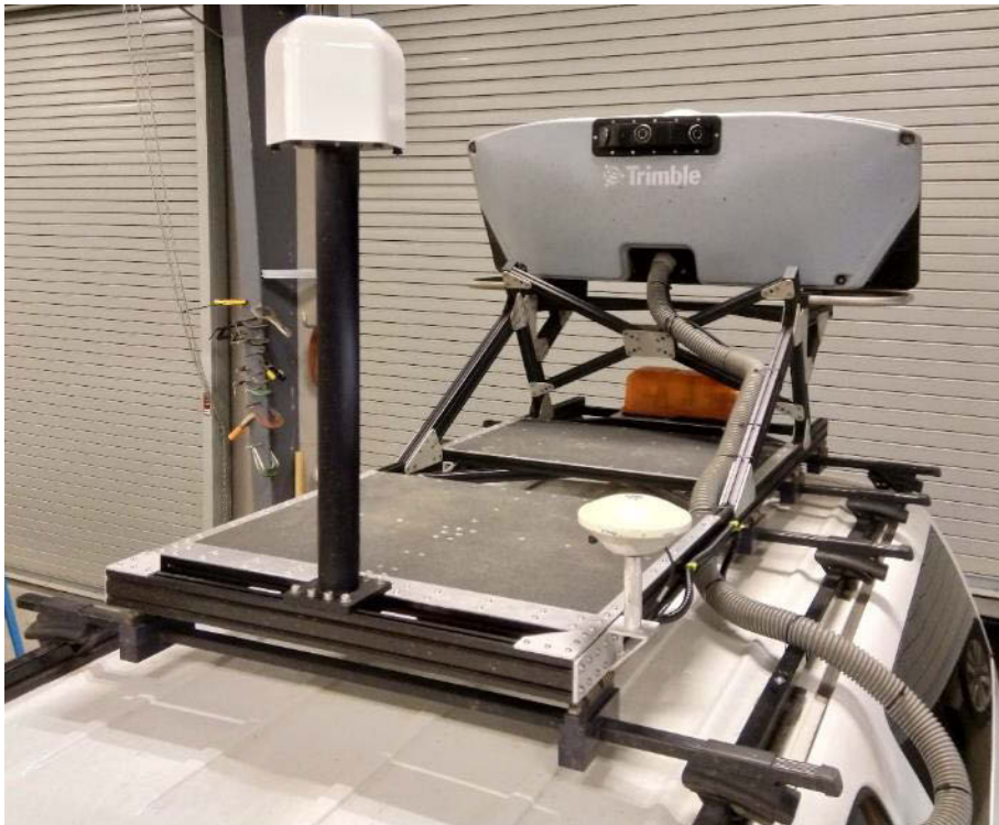
Figure 5.4: MX8 roof-mounted sensor pod with standing platform and Ladybug 5+ camera mount with camera cover
