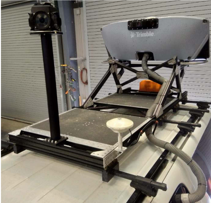
Figure 5.5: MX8 roof-mounted sensor pod with standing platform and Ladybug 5+ camera mount with camera cover removed
