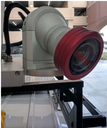
Figure 2.4: VMX-1HA Camera 2 mounted on the rear passenger side of the vehicle
