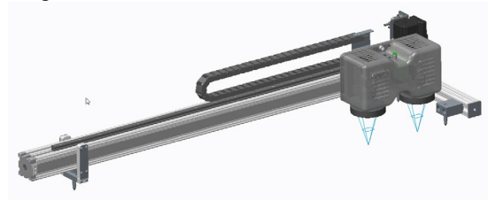
Figure 1: The automated laser-speckle imaging (LSI) strain sensor
