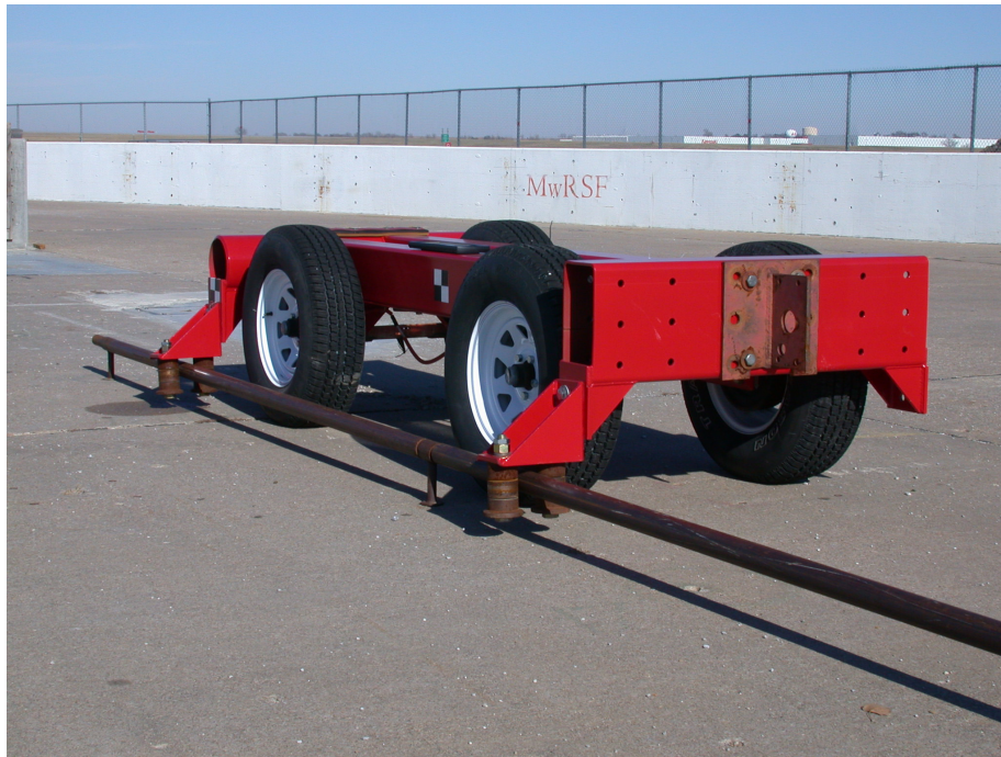
Figure 4. Bogie Positioned in the Guide Track Configuration
