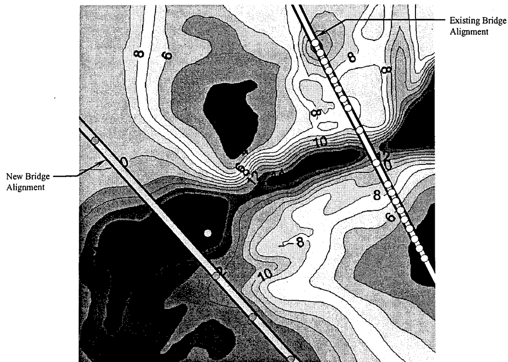
Figure 6-1 Bathymetric Survey conducted by University of Florida (Contour elevations in ft.)
