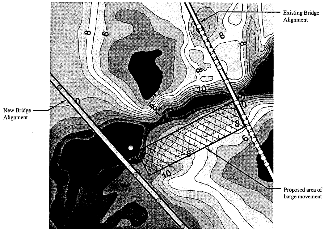
Figure 6-2 Proposed area of barge movement
