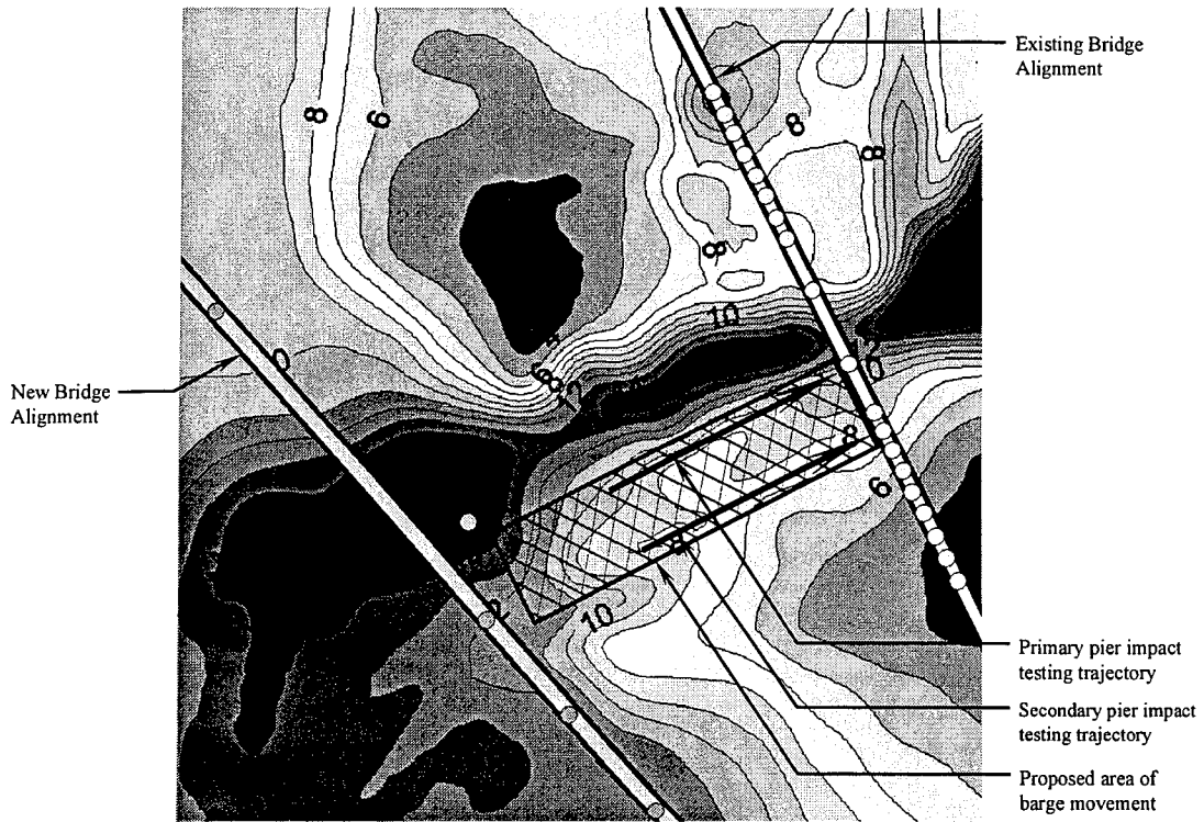
Figure 6-3 Proposed trajectories for impact tests
