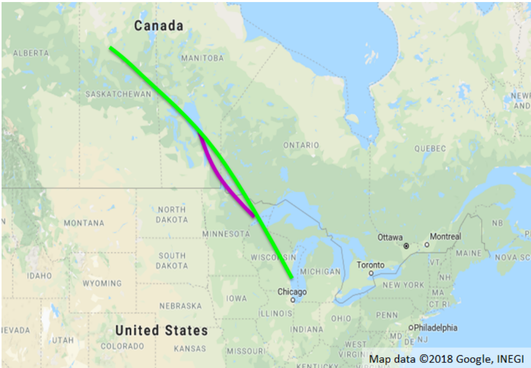
Figure 6-12: Flight 3 lateral deviation due to MOA with as-flown trajectory (green) and original planned trajectory (magenta)
