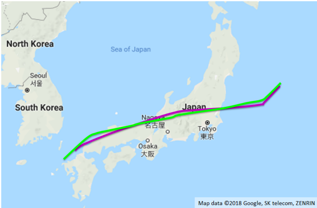
Figure 6-20: Flight 4 lateral deviation with as-flown trajectory (green) and original planned trajectory (magenta)
