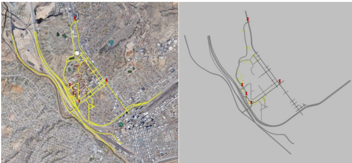
Figure 5. 1 Coded road network in VISSIM.
