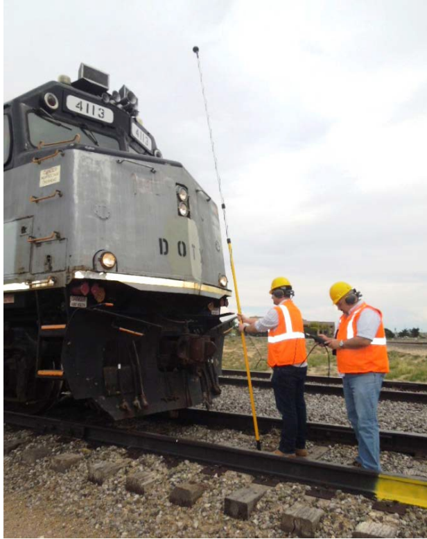
Figure 58. Measuring the DOTX 4113 5-Chime Air Horn Sound
