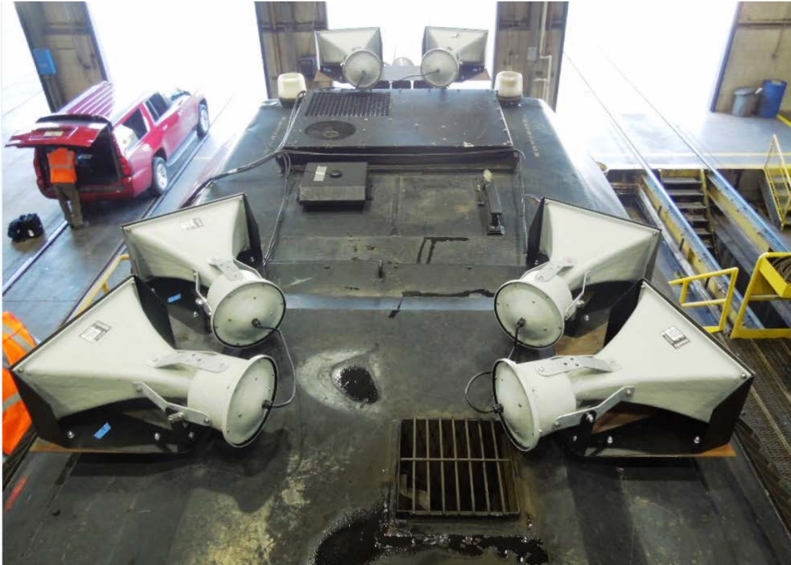
Figure 56. AWD Speakers Mounted on an F40 Locomotive (DOTX 4113)
