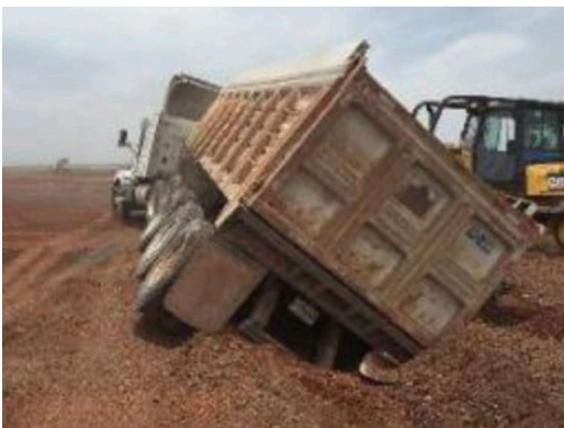
A. Truck on soil geogrid-reinforced soil
