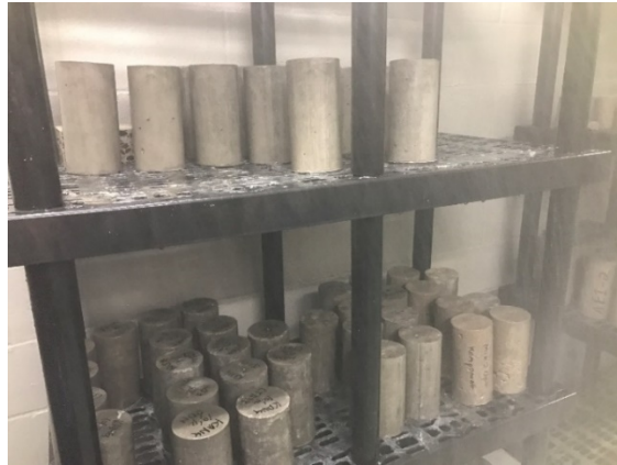
Figure 3.2.2: 100% moist room at 23±2°C temperature
