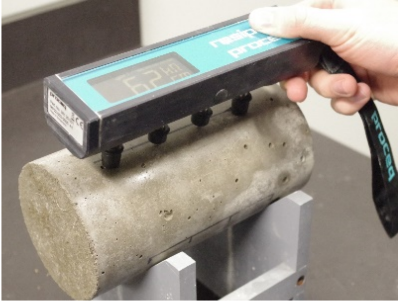
Figure 3.3.2 Illustration of surface resistivity meter
