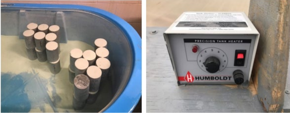
Figure 3.2.1: Limewater tank at 23°C temperature and precision tank heater
