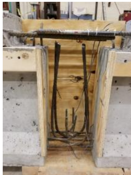
Figure 180. Reinforcement within continuity joint specimen representing new construction
