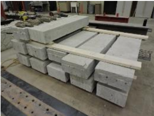
Figure 297. Large-scale corrosion joint specimens before chipping
