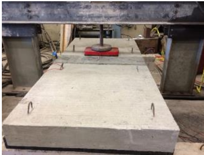
Figure 87. Full-depth UHPC slab joint load test setup
