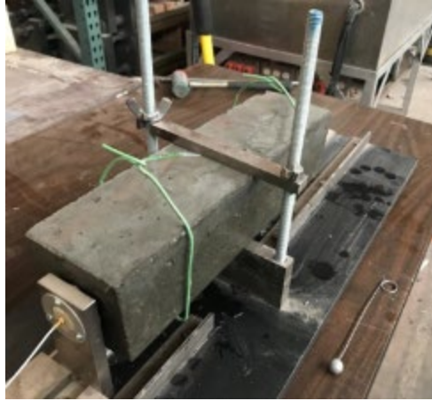
Figure 272. Freeze-thaw specimen arranged for dynamic modulus testing
