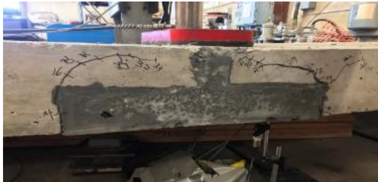
Figure 149. Cracks on the south side of Ductal® slab joint 2 after part 1 testing
