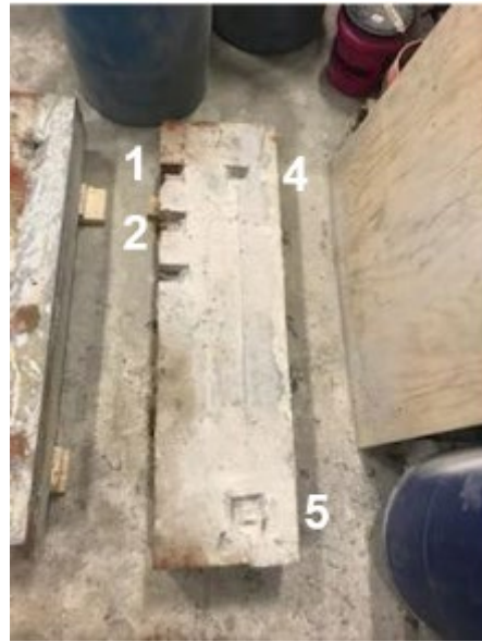
Figure 312. Chipping sequence of large-scale corrosion specimens
