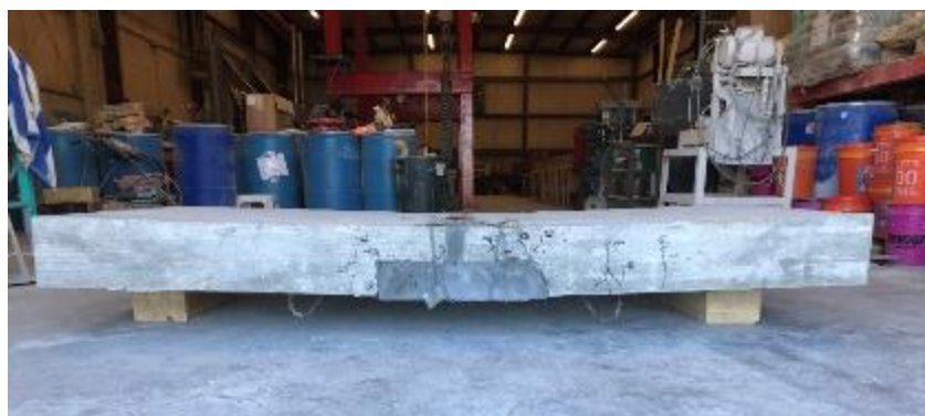
Figure 129. J3 Slab joint 1 curvature after failure
