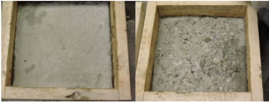
Figure 60. Sandblasted (left) and chipped (right) surface preparations
