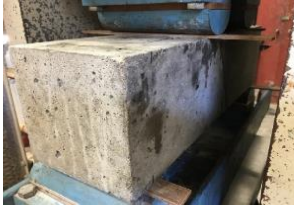
Figure 55. Composite MOR specimen testing apparatus
