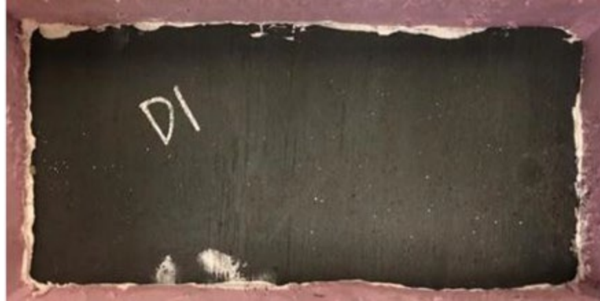
Figure 284. Visual corrosion of steel fibers on Ductal® specimen - 25 cycles
