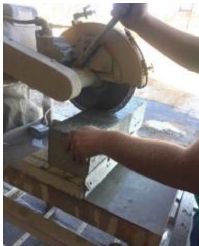
Figure 52. Cutting small-scale specimen at 90° angle to the horizontal
