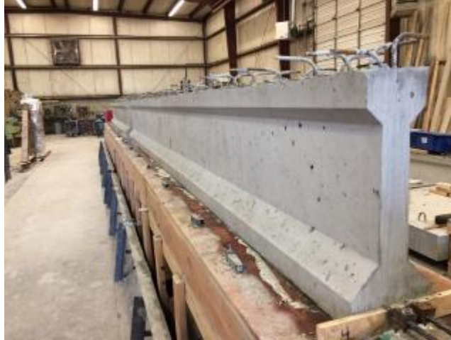
Figure 174. Completed set of two prestressed beam specimens
