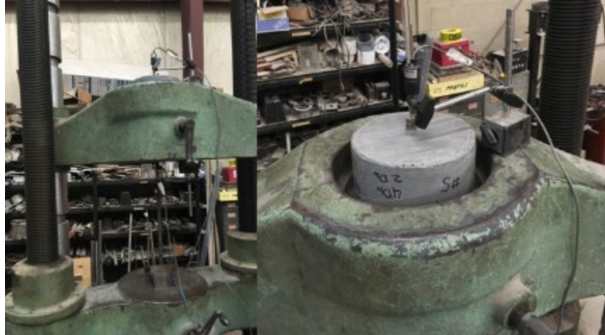
Figure 66. Pullout test of No. 5 bar specimen with 1% fiber mix showing the overall setup (left) and a closeup view of the as tested top of the specimen (right)
