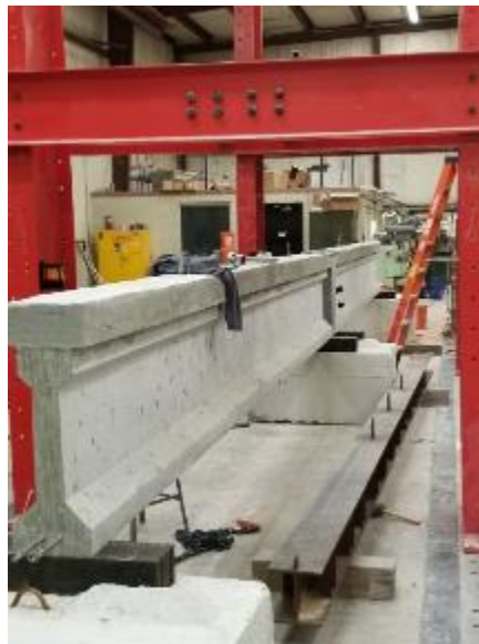
Figure 195. Continuity joint specimen in place for testing
