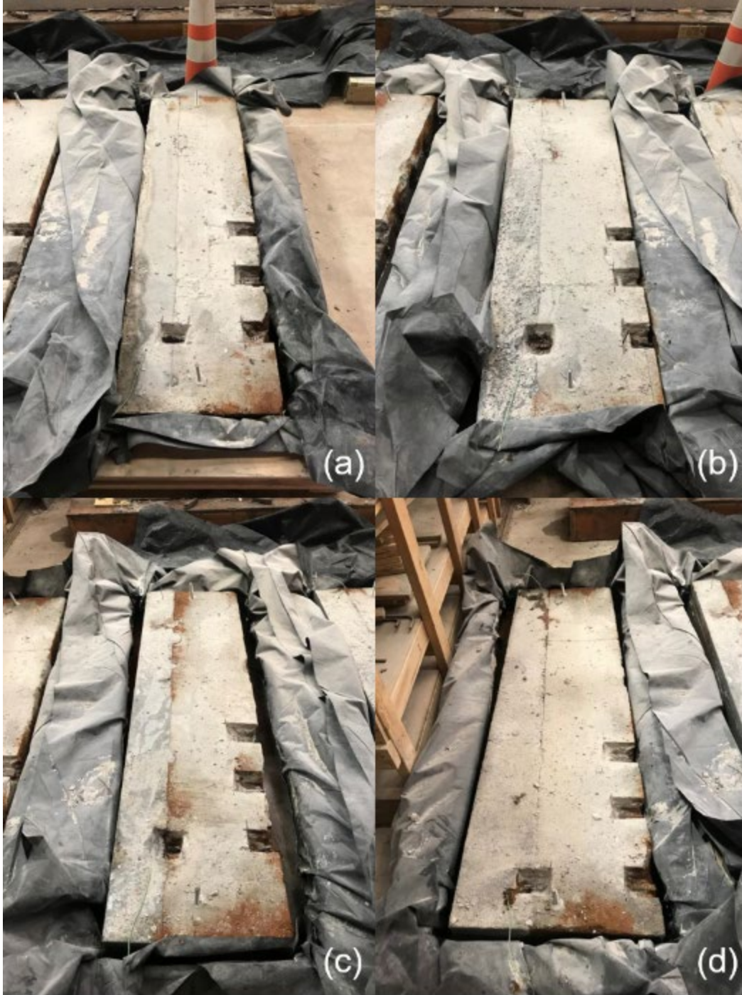
Figure 316. Week 10 update for large-scale corrosion specimens using (a) ODOT AA, (b) J3, (c) Ductal®, and (d) Phoscrete
