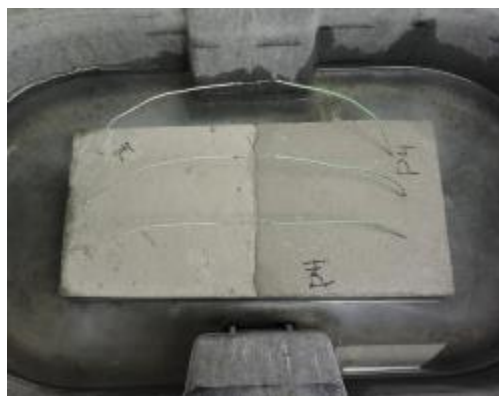
Figure 289. Typical small-scale corrosion testing specimen in the chloride solution
