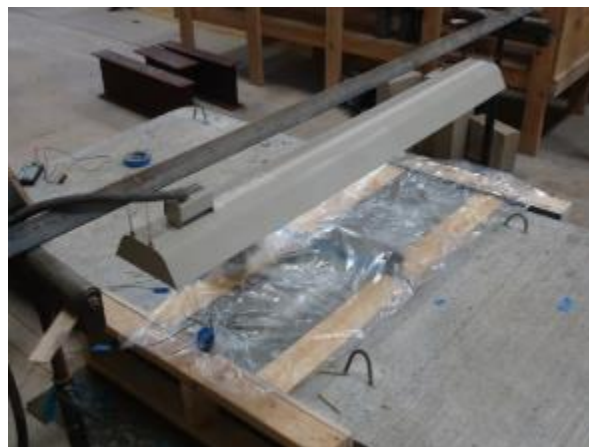
Figure 84. Heat curing for Ductal ® slab joint 1
