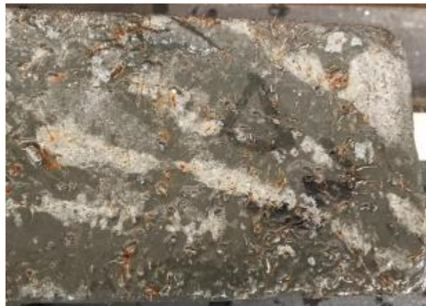
Figure 281. Surface corrosion of Ductal® freeze-thaw specimen - Cycle 350
