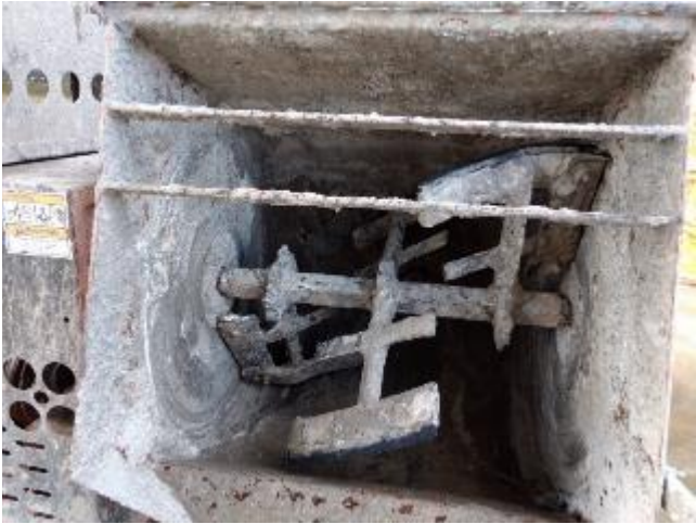
Figure 47. Paddles of the mortar mixer used at Coreslab demonstration
