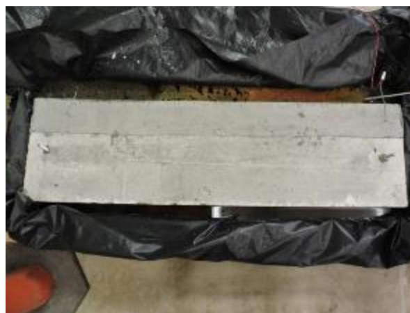
Figure 303. Corrosion in water of typical large-scale corrosion specimens
