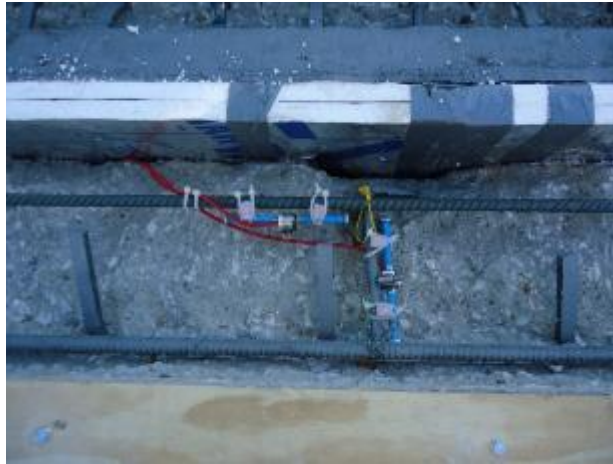
Figure 331. Strain gages within the joint header
