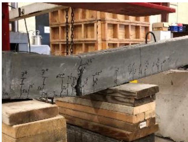
Figure 77. Crack pattern typical of SB-J5 with 2% fibers
