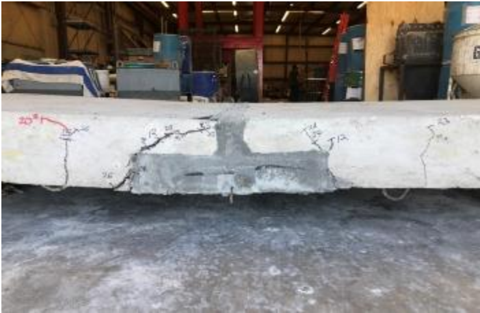
Figure 143. Ductal® slab 1 after part 2 of testing
