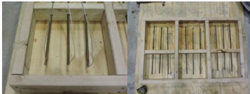
Figure 288. Small-scale corrosion specimen molds
