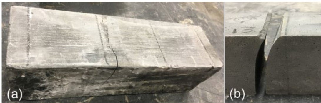
Figure 44. Photo showing typical crack pattern for fiber reinforced (a) and unreinforced (b) modulus of rupture specimens
