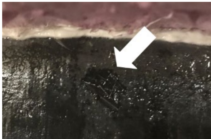
Figure 287. Visual pocketing on Ductal® specimen - 50 cycles
