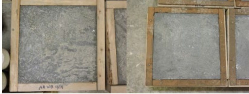
Figure 61. Pull-off test specimens for Ductal® (left) and J3 (right)
