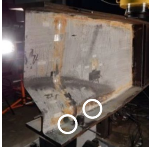
Figure 13. Undamaged girder failure (Zmetra 2015)
