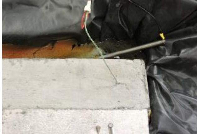
Figure 300. Stainless steel rod and electrical wiring for large-scale corrosion testing
