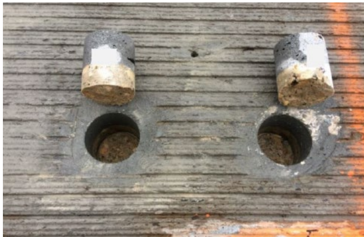
Figure 4. Direct pull-out test cores (Graybeal 2017)
