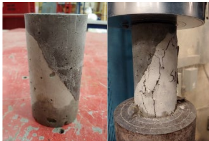
Figure 59. Composite slant shear specimen prior to testing (left) and after testing (right)
