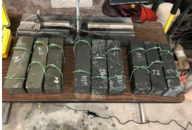
Figure 276. Condition of all freeze-thaw specimens - Cycle 0
