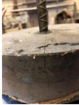
Figure 64. Splitting failure of 2d_b embedment bond test specimen
