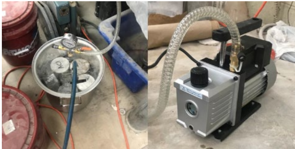
Figure 270. Vacuum desiccator (left) and pump (right) used for RCIP specimen preparation
