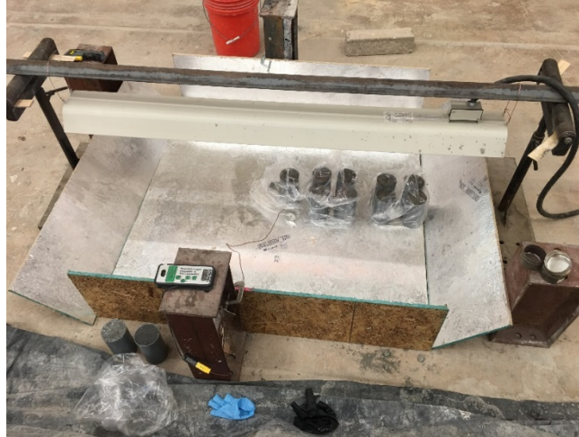
Figure 49. Heat curing apparatus and Ductal® specimens during heat curing test
