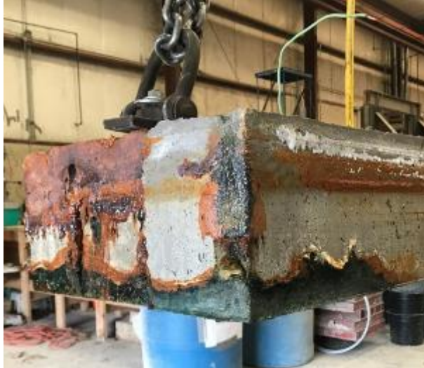
Figure 324. Final state of Phoscrete large-scale corrosion specimen after week 10
