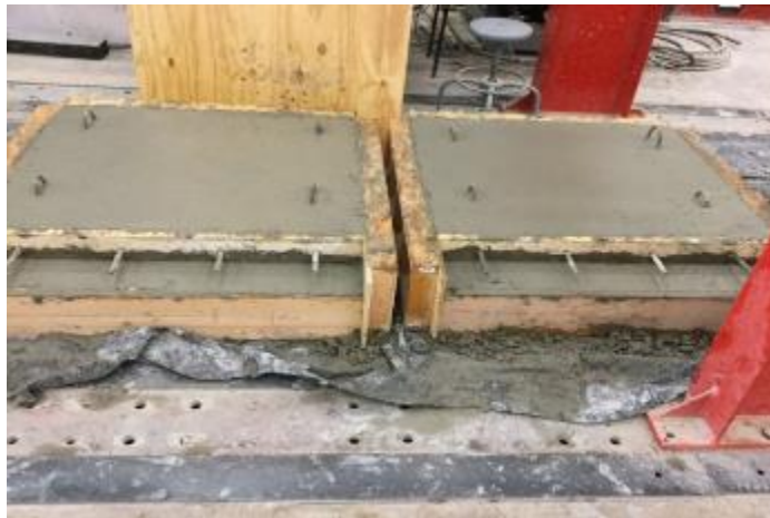
Figure 94. Side-by-side slabs after finishing applied
