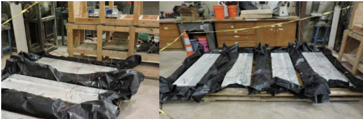
Figure 301. Large-scale corrosion testing setup showing power supplies (left) and all specimens in place (right)
