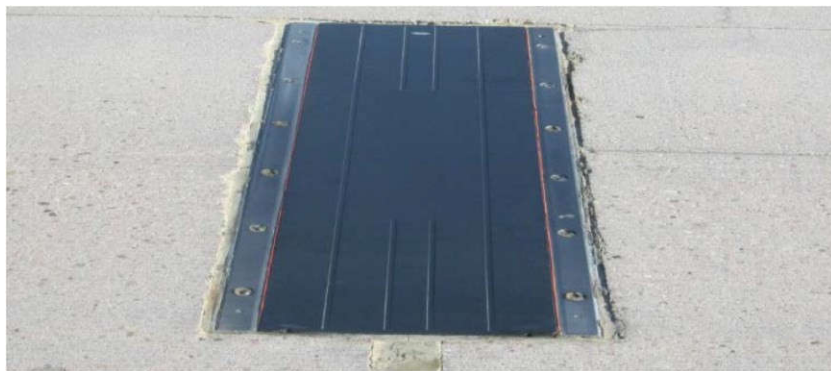
Figure 9. Photo. Bending plate installation (FHWA 2018).
