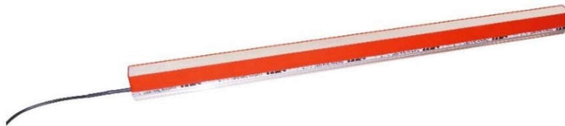
Figure 15. Illustration. Strain gauge strip sensor (FHWA 2018).
