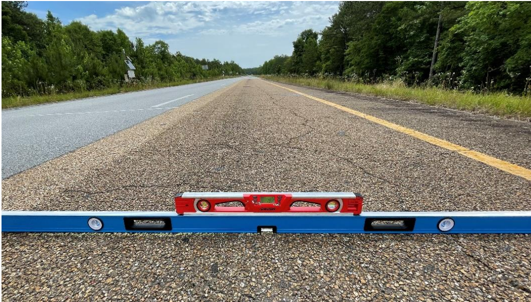
Figure 19. Picture. Straightedge and digital level used for superelevation measurements.
