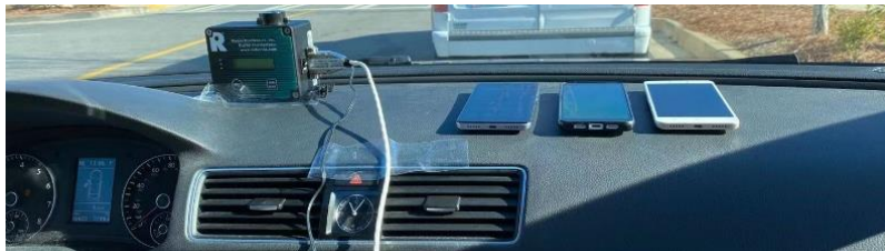
Figure 16. Picture. Device setup for multi-device sensor repeatability test.
