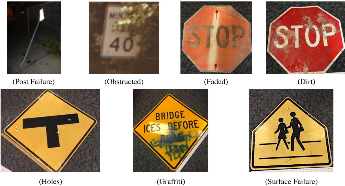
Figure 4. Pictures. Common distresses in sign condition assessment.
