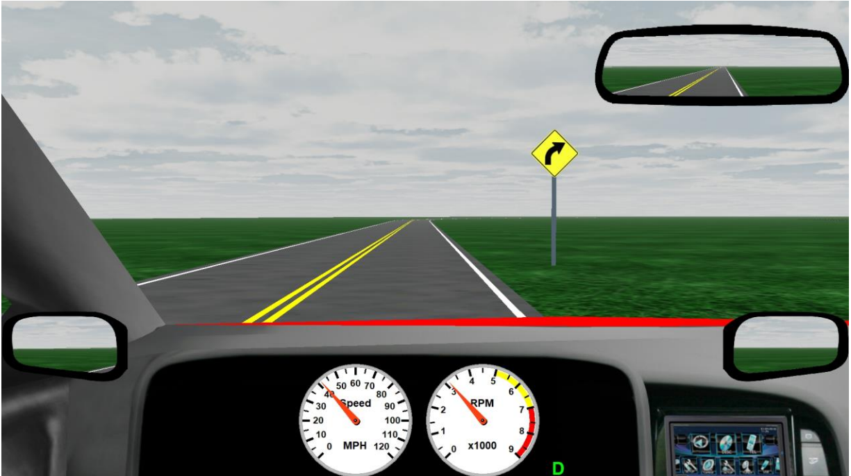
Figure 19. Screenshot. Countermeasure 6 – Curve warning sign.
