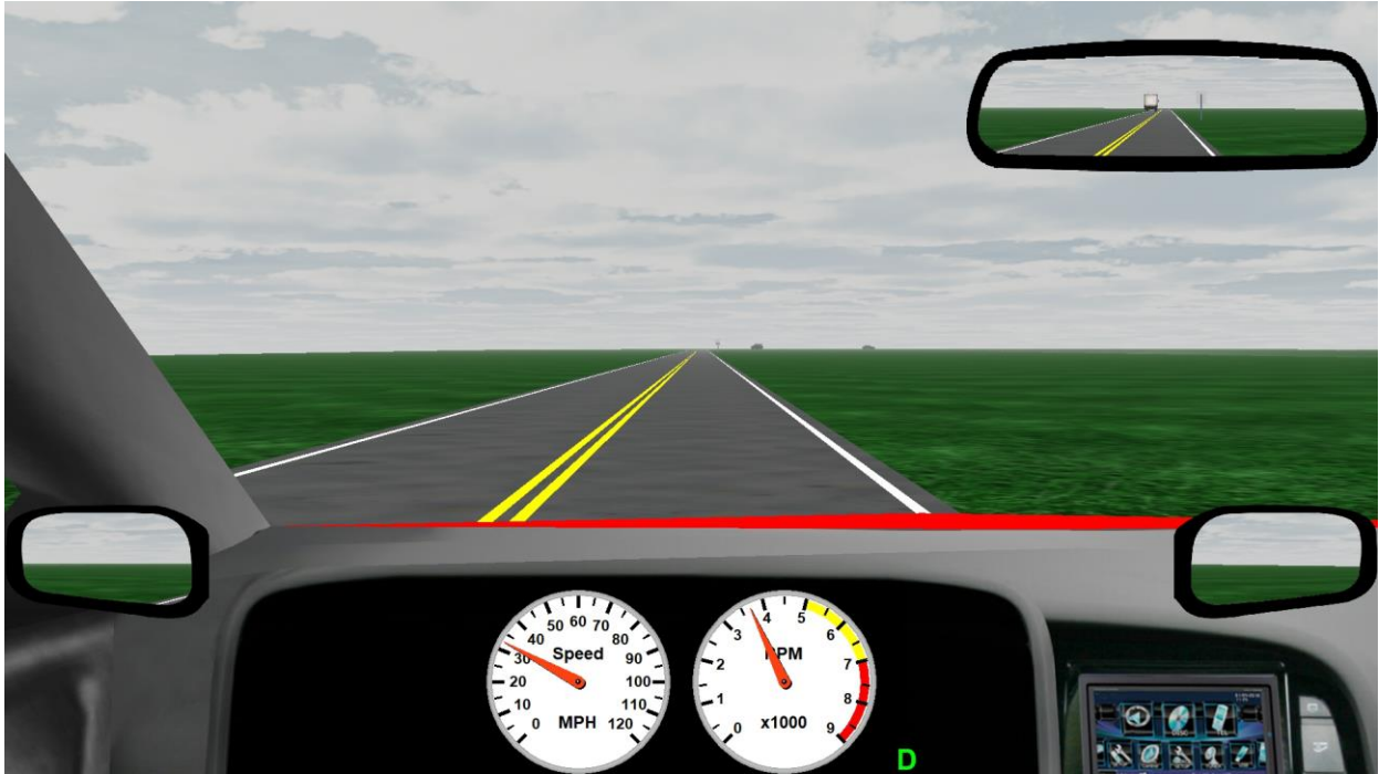
Figure 15. Screenshot. Countermeasure 2 – Edge line pavement marking.
