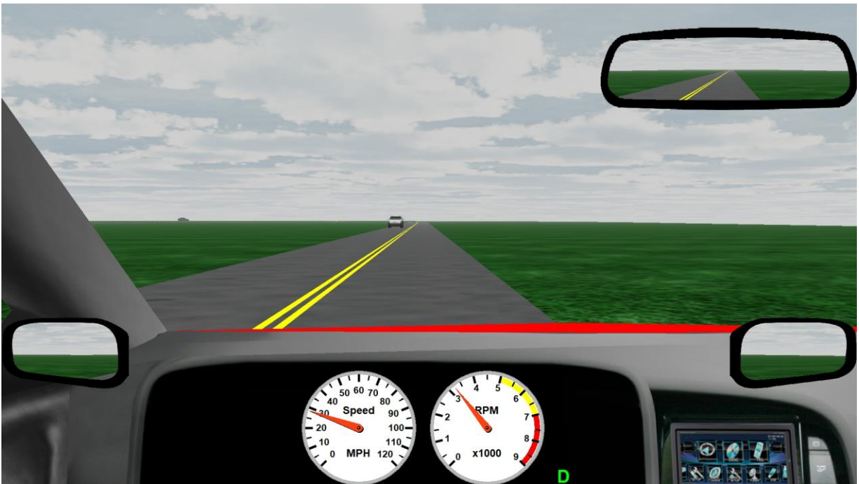
Figure 14. Screenshot. Countermeasure 1 – Centerline pavement marking.
