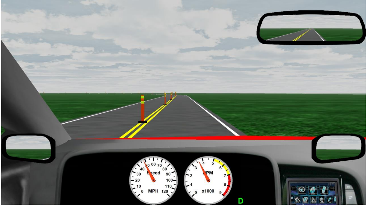
Figure 17. Screenshot. Countermeasure 4 – Flexible delineator posts.
