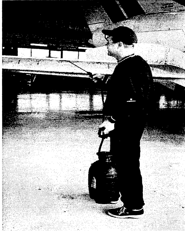
FIGURE 6a. FLUID APPLICATION BY PORTABLE SPRAYER
