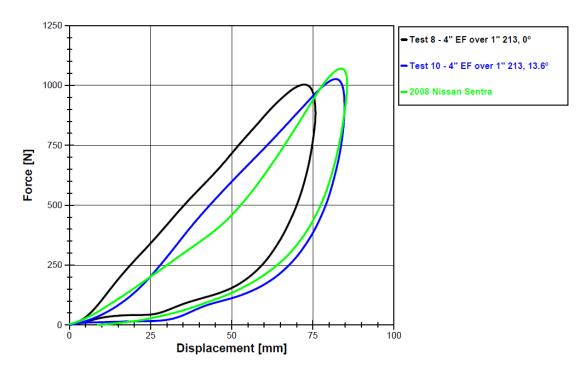
Figure 13. Out-of-Vehicle Foam Angle Verification
