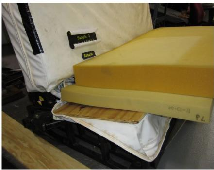
Figure 3. FMVSS No. 213 Test Bench Cushion Assembly
