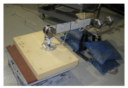
Step 3: Measure the angle of the pendulum arm when it makes first contact with the foam Secure the PID using sand bags and/or weights on either side to prevent movement during impact.
