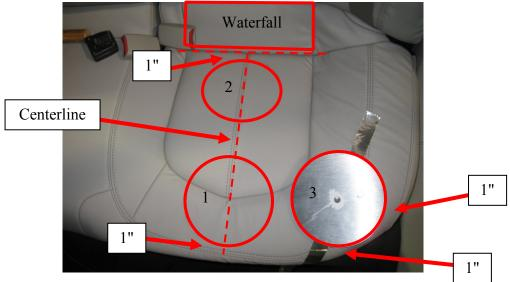
Step 2: Set up the PID and mark location
