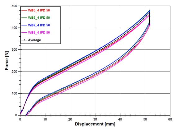
Figure 30. WB Foams 5 to 8 Force-Displacement Overlay for 50 Percent IFD Testing
