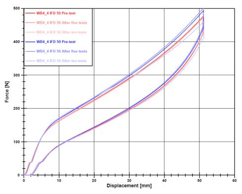
Figure 33. WB Foam 4 Force-Displacement Overlay for 50 Percent Testing
