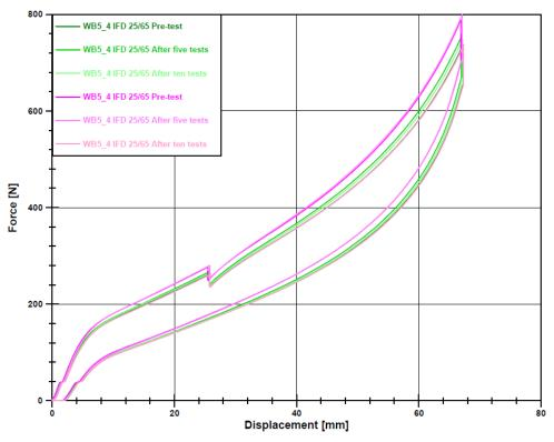
Figure 32. WB Foam 5 Force-Displacement Overlay for 25/65 Percent Testing
