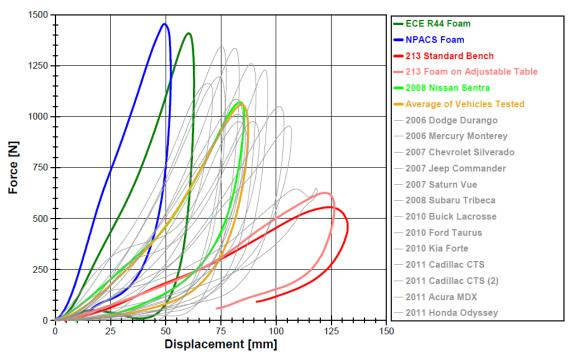
Figure 10. Force-Displacement Curves for the Vehicle Fleet at Location 2
