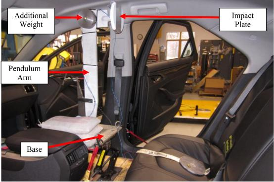
Figure 5. Pendulum Impact Device
