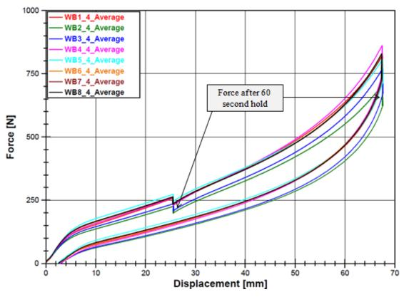
Figure 29. IFD Force-Displacement Curves for WB Foams 1 to 8
