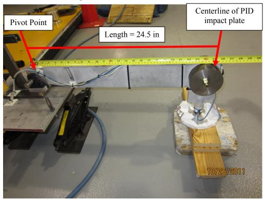
Step 5: Measure the length of the PID arm from pivot point to center of the PID impact plate
