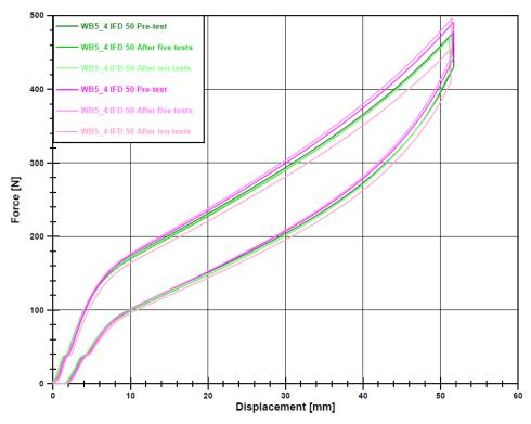
Figure 34. WB Foam 5 Force-Displacement Overlay for 50 Percent Testing
