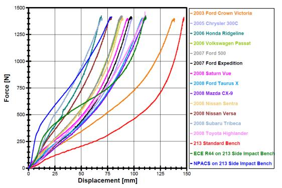
Figure 2. Force-Displacement Response for Quasi-Static Tests
