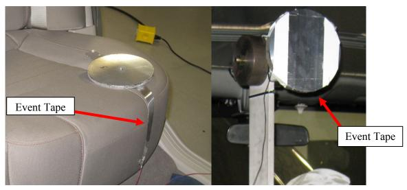
Step 5: Add event tape to the seat and PID impact plate
