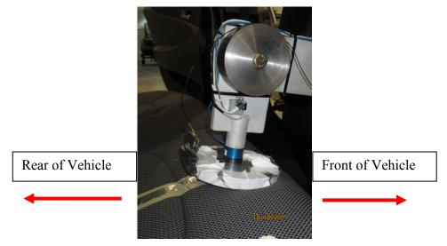
Step 5: Attach the accelerometers, angular rate sensor, and load cell to the pendulum arm
