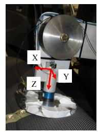
Step 4: Attach the accelerometers, angular rate sensor, and load cell to the pendulum arm
