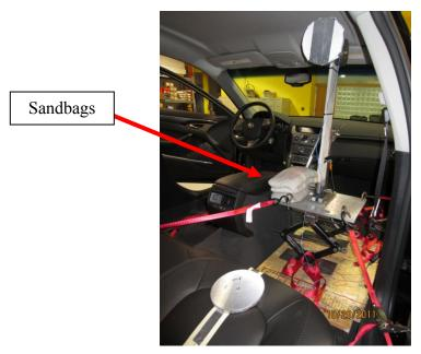
Step 4: Alternative - secure the PID using ratchet straps and sand bags
