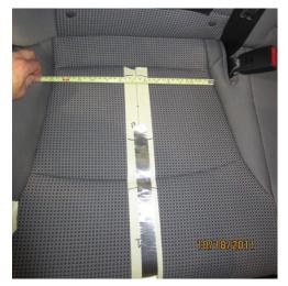
Step 2: Measure and mark the centerline of the outboard seat
