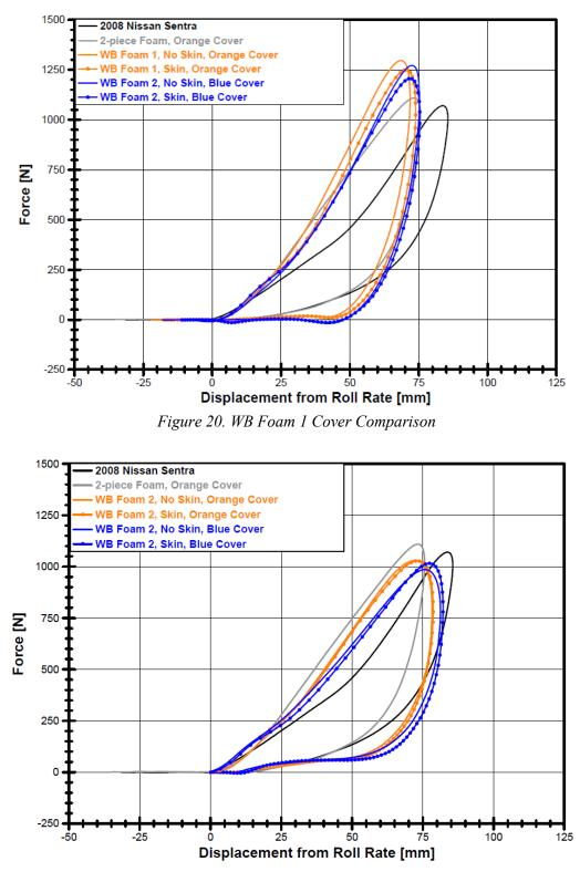
Figure 21. WB Foam 2 Cover Comparison
