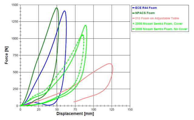
Figure 12. Dynamic Force-Displacement Plots of Foam Samples
