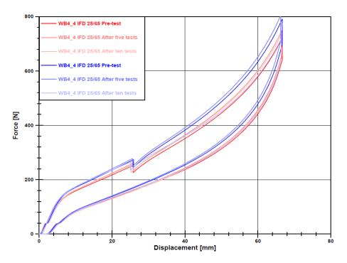
Figure 31. WB Foam 4 Force-Displacement Overlay for 25/65 Percent Testing
