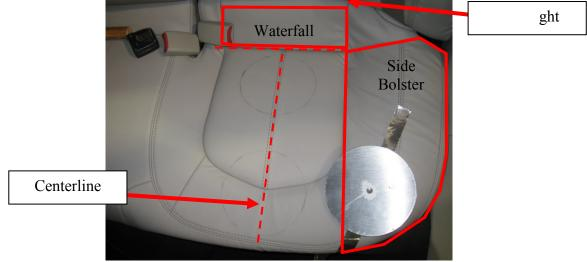
Figure 6. Geometry of the Rear Seat
