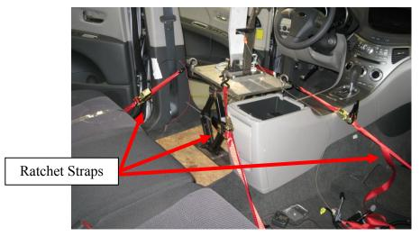
Step 4: Secure the PID using ratchet straps
