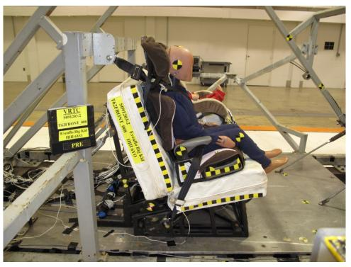
Figure 4. FMVSS No. 213 Set-up
