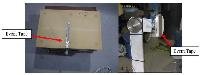
Step 4: Add event tape to the foam and PID impact plate
